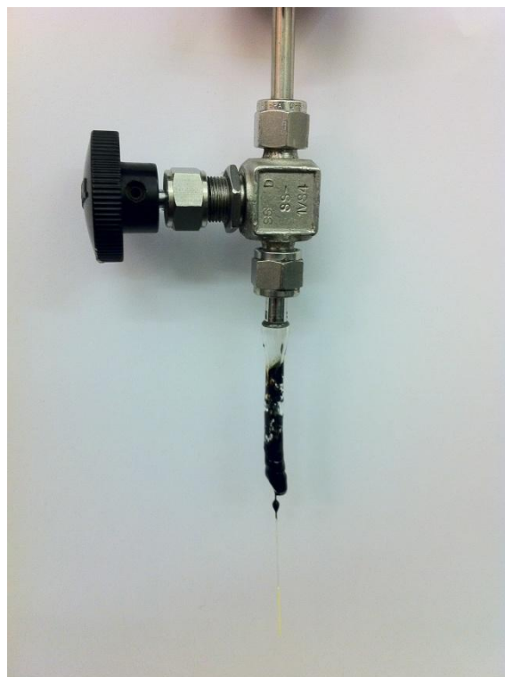
Figure 6-26: Capillary adapter containing a sample of Zn (TBAPy) 1'
