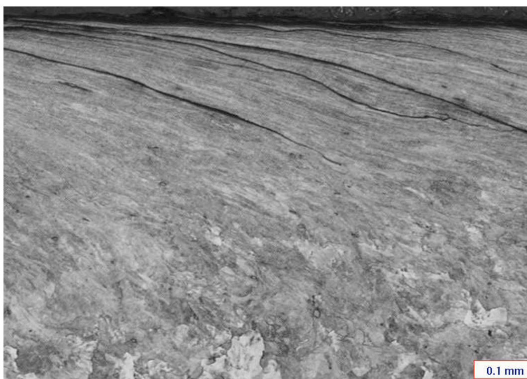
Figure B.2 Optical microscope image, P260, 5000 cycles dry and 5000 cycles wet.
