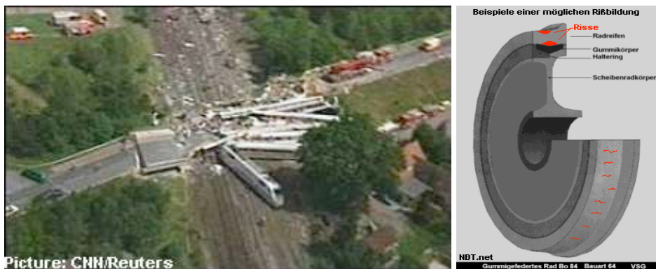
Figure 1.2 Accident at Eschede, Germany, 1998. “101 people killed and a further 88 injured” 1 . “A cracking inside the ring of the wheel was responsible. There was no indication of material or production failure. This crack was caused by excessive load and wear.” 2
