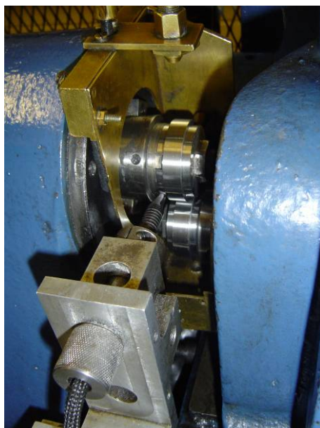
Figure A.8 Discs INR1 and INW1 mounted on the machine before testing.
