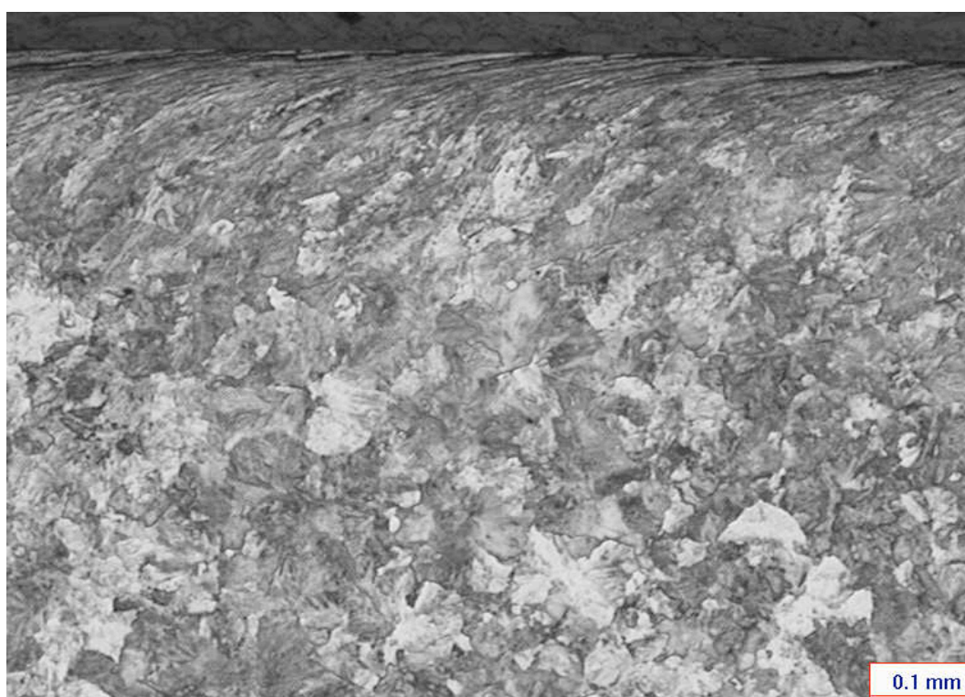
Figure B.8 Optical microscope image, V350, 5000 cycles dry and 5000 cycles wet.
