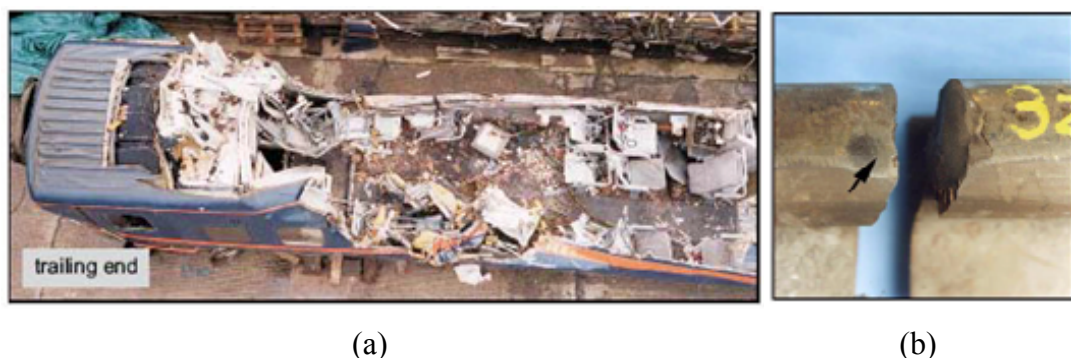
Figure 1.1 The Intercity 225 train derailed roughly 0.8 km south of Hatfield Station on 17 October 2000. Four passengers were killed and over seventy people were injured. The immediate cause was the fracture and subsequent fragmentation of the high rail, due to the presence of multiple and pre-existing fatigue cracks in the rail. (a) Coach G showing extent of damage to seating area, (b) One of the fractures, with arrow indicating polished area (ORR, 2006).
