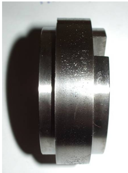
Figure A.12 VA 350 Grade rail disc after testing for 5000 cycles under dry conditions in test INNOT-04. Very small amounts of surface flaking could be seen.
