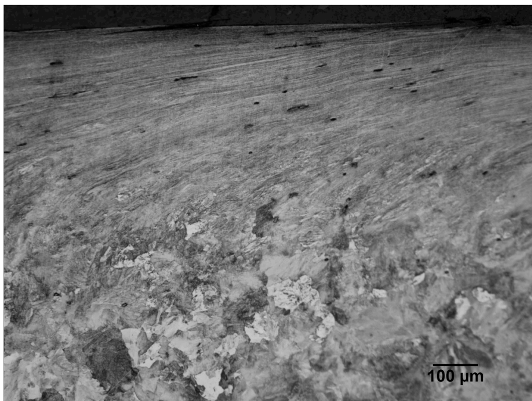
Figure B.21 Optical microscope image, P260, 15000 cycles dry, INNOT-22
