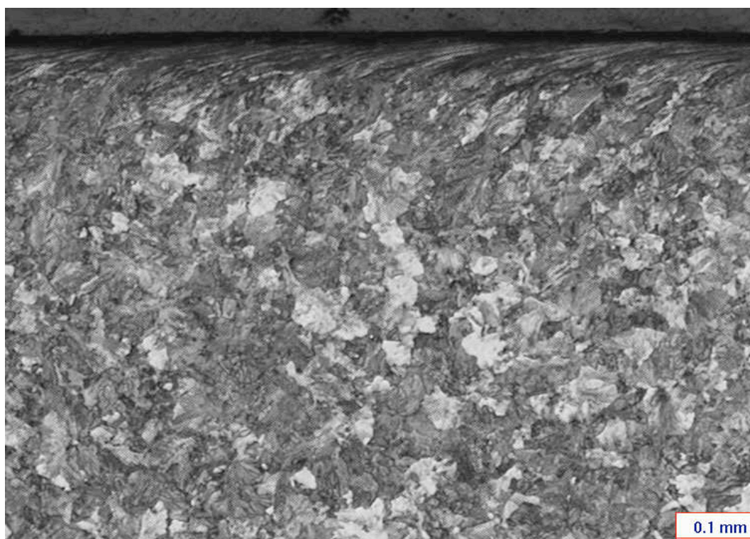
Figure B.7 Optical microscope image, V350, 5000 cycles dry.
