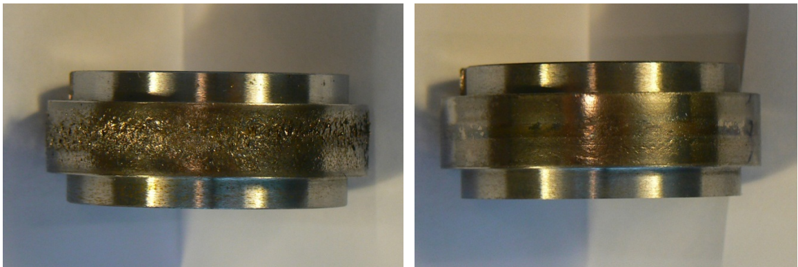
Figure A.22 Test INNOT-08. 5000dry + 5000wet. Left: rail C260 – INR23. Right: wheel – INW13
