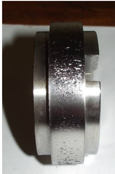
Figure A.14 VA 350 grade rail disc from test INNOT-06, after 15000 cycles dry contact. Considerable surface flaking has taken place.
