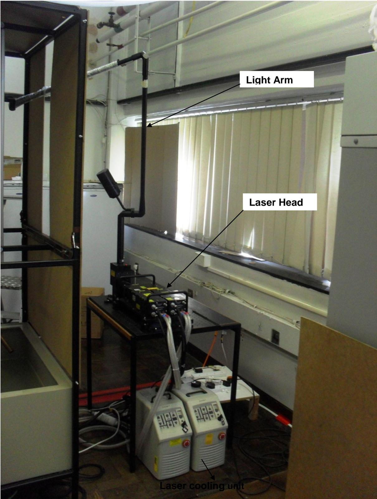
Figure 3.13: Lasers Used for S-PIV System
