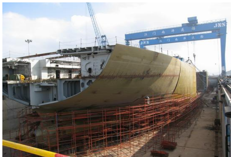
Figure 8.7 Section Constructing Method in Nanyang Shipyard
