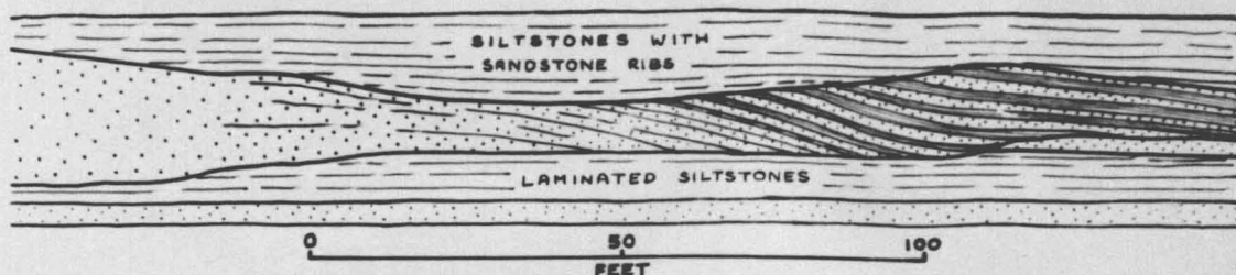
FIG. I.34 LATERAL PASSAGE OF CHANNEL SANDSTONE INTO SILTSTONE/SANDSTONE UNIT SHOWING INCLINED BEDDING
