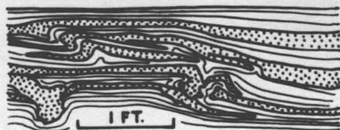
FIG. 1.33 CONTORTIONS IN LAMINATED SANDY SILTSTONE
