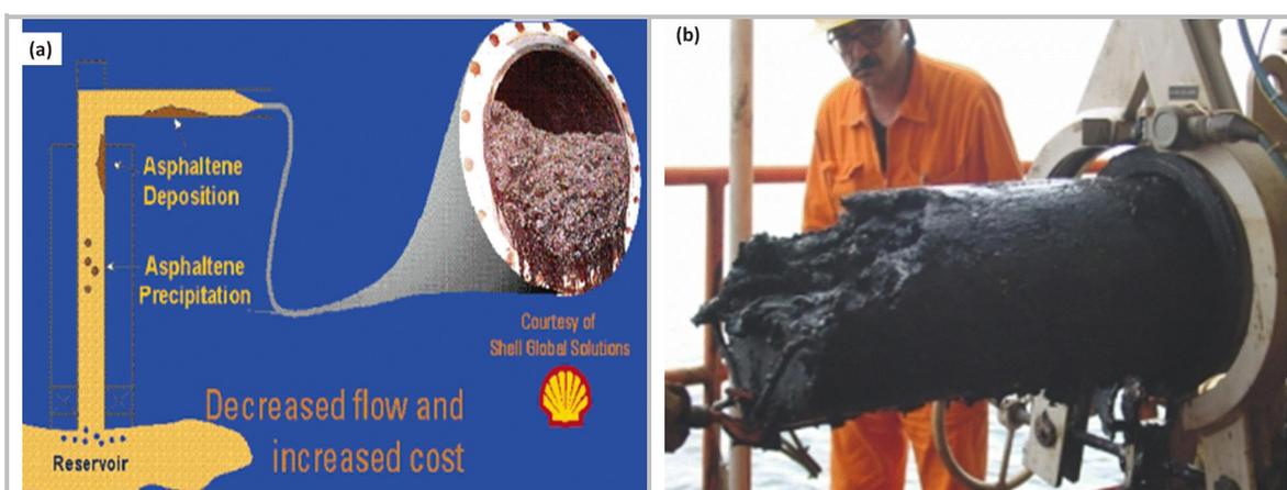
**Figure 1.1: Asphaltenes are likened to cholesterol in human body that precipitates and deposits to plug the pipeline leading to shut down of the system for repairs (Headen et al., 2007; Creek, 2005).**
