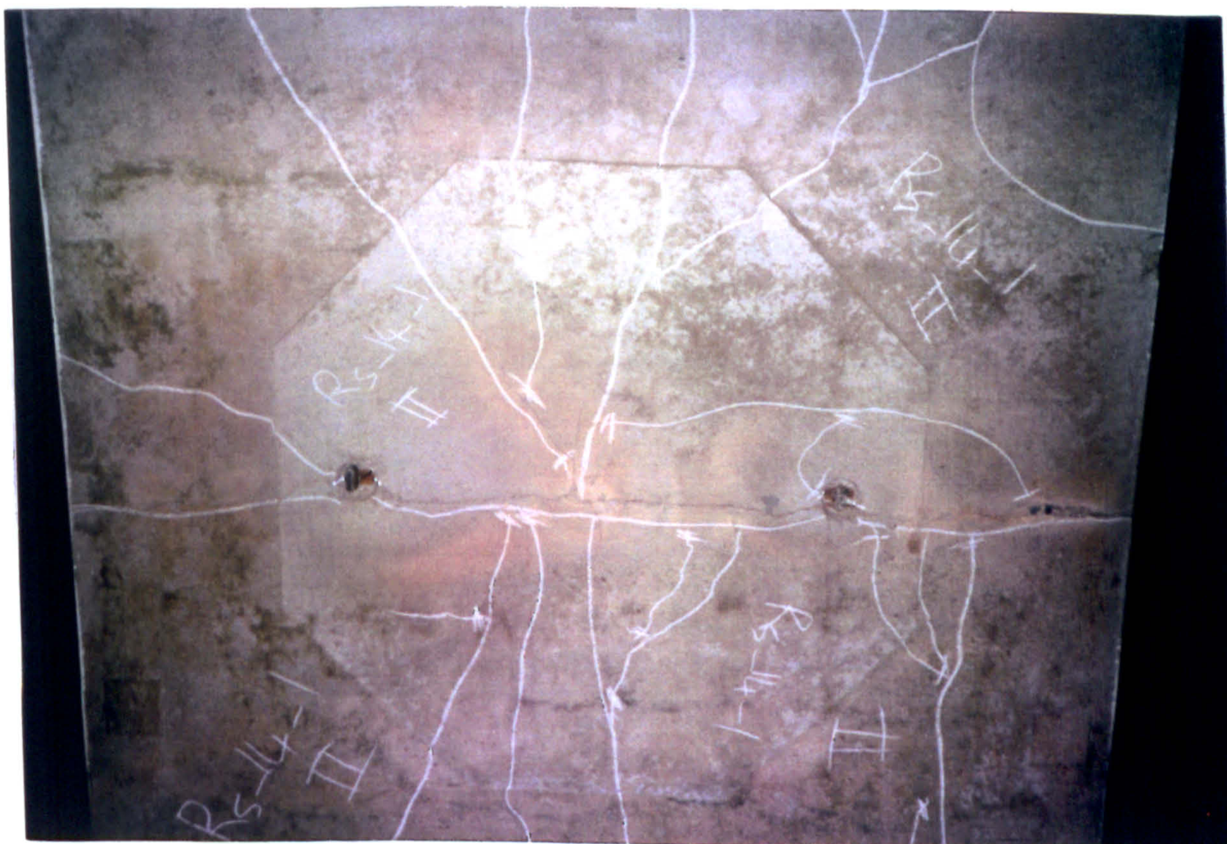
PLATE 6.3 : Bottom Crack Patterns at Failure of Raft RS1 - Module M2
