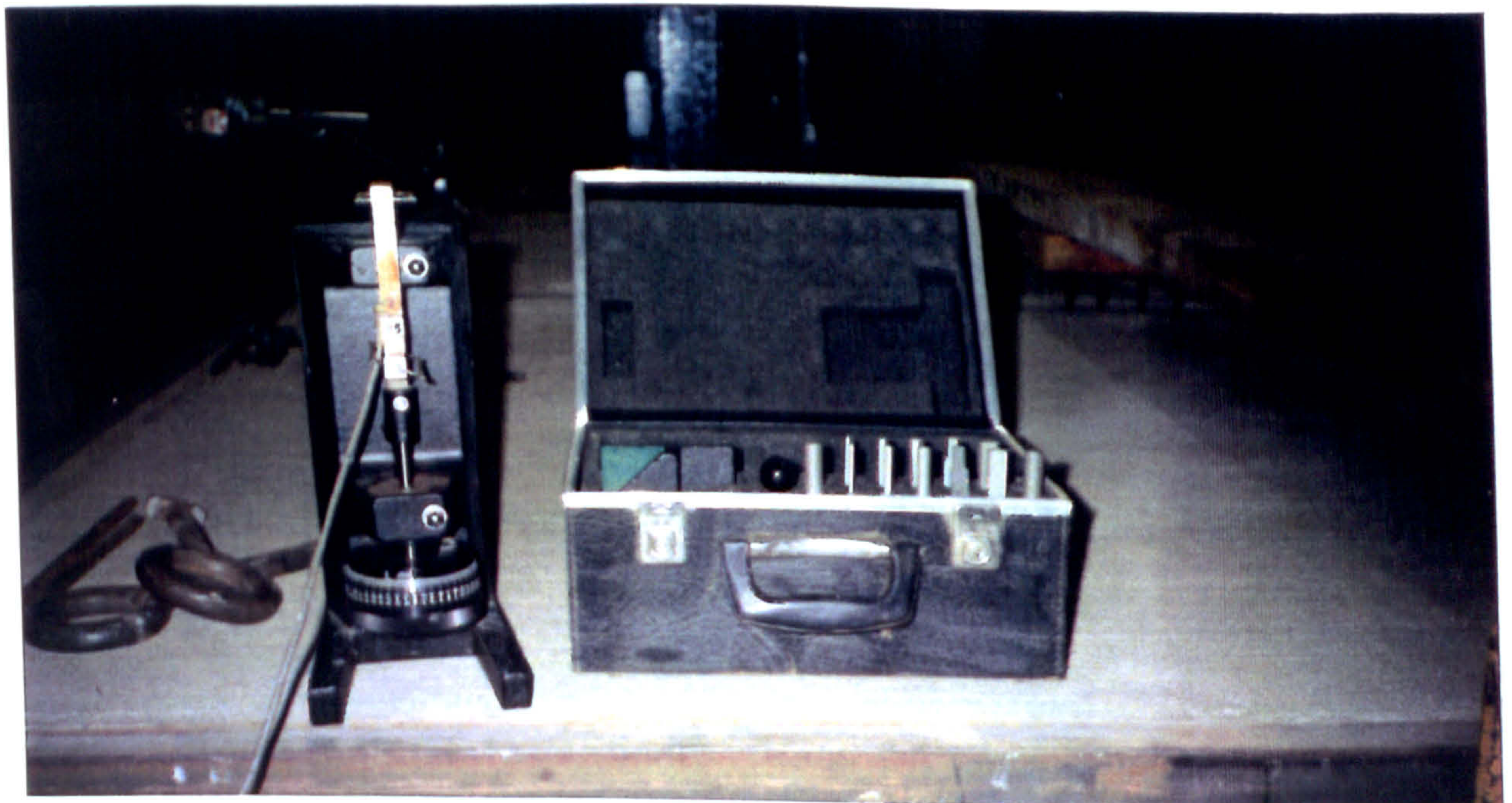
Fig. 4.6 : Extensometer Calibrator For Strain Transducers
