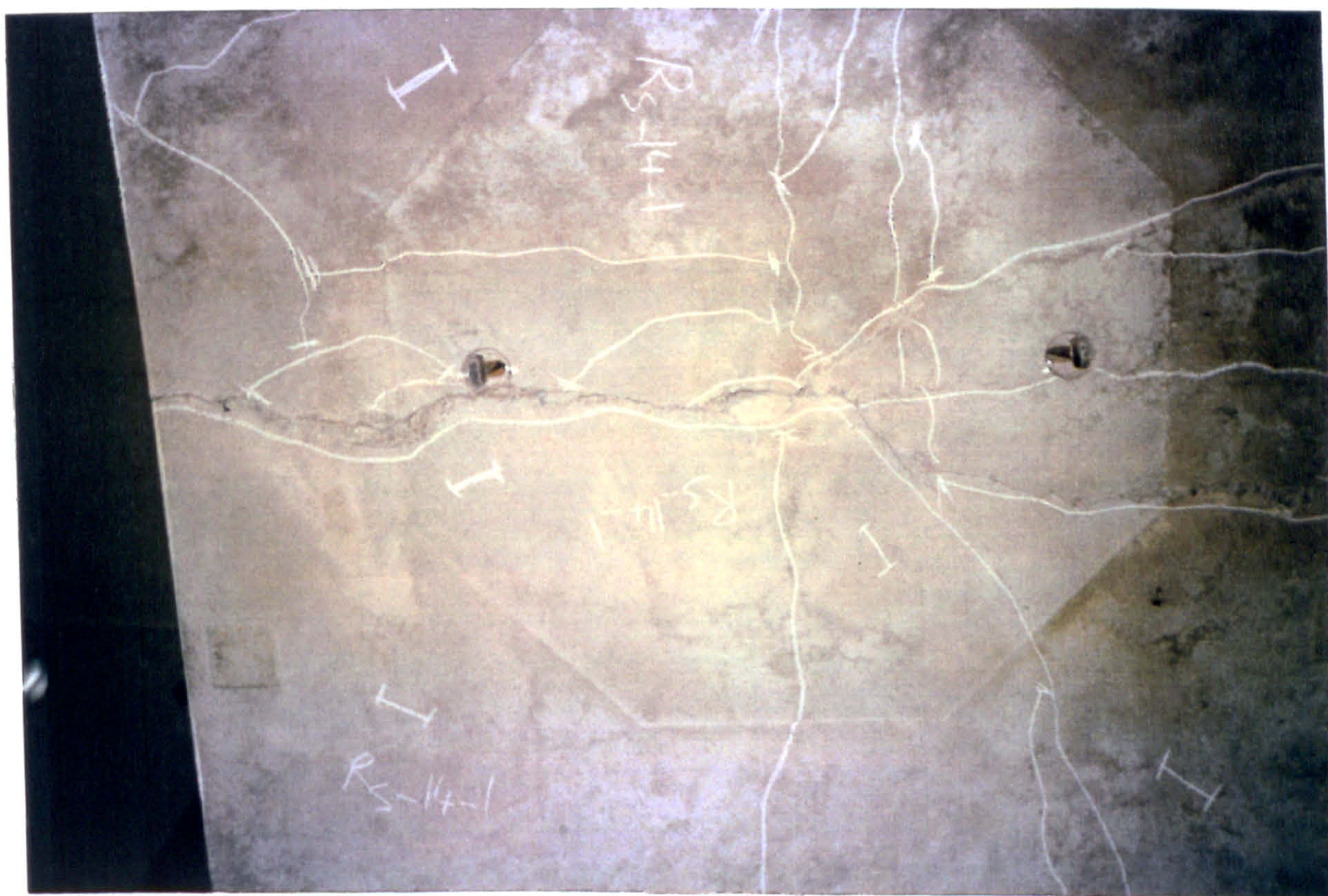
PLATE 6.3 : Bottom Crack Patterns at Failure of Raft RS1 - Module M2
