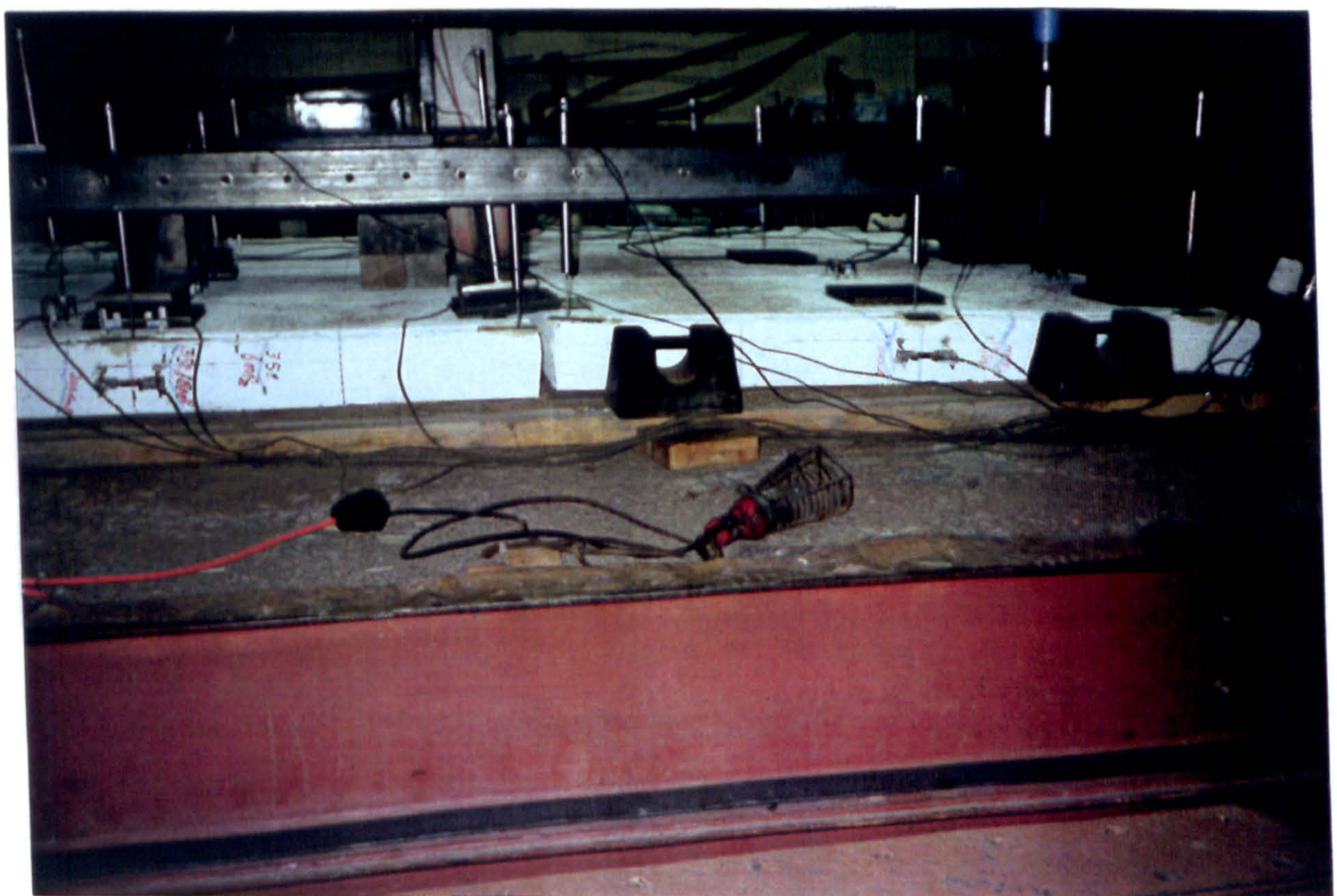
PLATE 5.6 : The Differential Deflection at the Joint due to Loading P4
