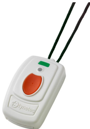
Figure 2-3: A Tynetec telecare alarm (from [163]) designed to be worn on a belt or waistband or threaded onto a pendant, the red button on the device can be pressed to send an alarm to a call centre.
