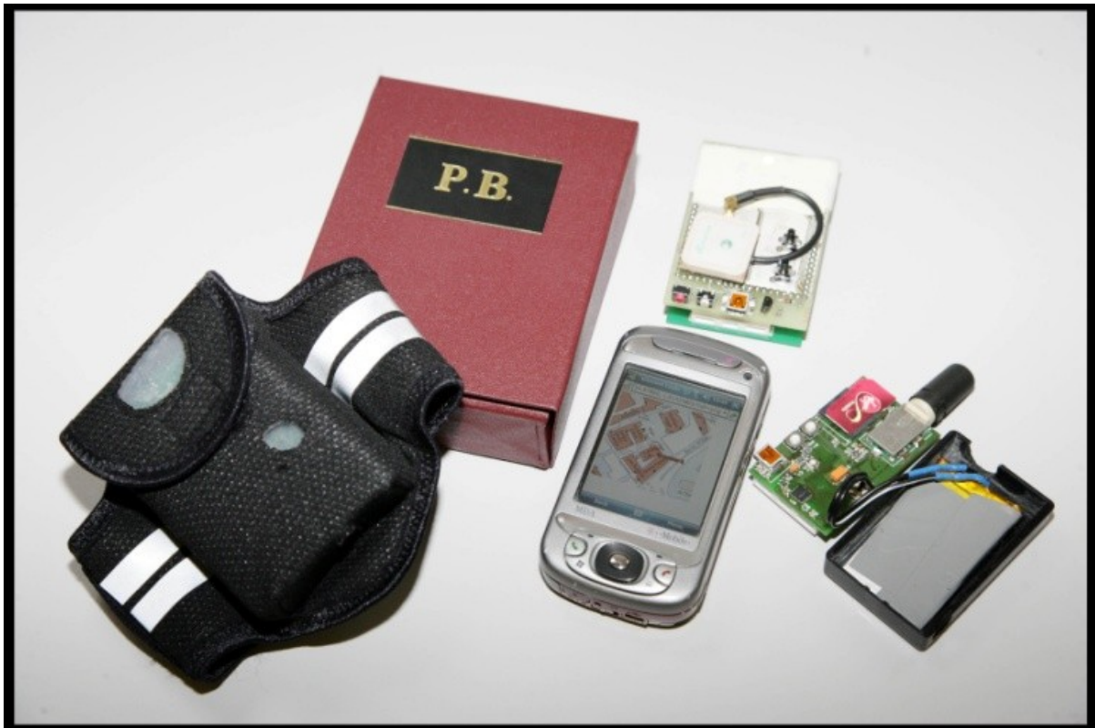
Figure 4-3: From left to right John's armband tracker, The Driver's notebook tracker, (bottom) The Wife's mobile interface and (top) the internal electronics of the device
