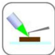
**Figure 3.6. Depiction of off-axis coupling where the Raman microscope objective is set at an angle such that there are no effects from the AFM cantilever. The Raman microscope is still in back scattering mode [Horiba Jobin Yvon, 2011]**
