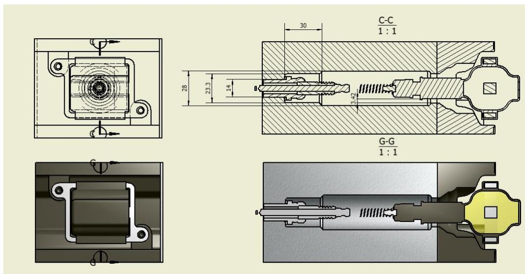
Figure 4.82: Spark plug bore and coil channel 3D parametric model
