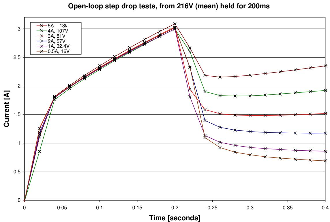
Figure 4.68: Open-loop response step decreases in applied voltage, initial response
