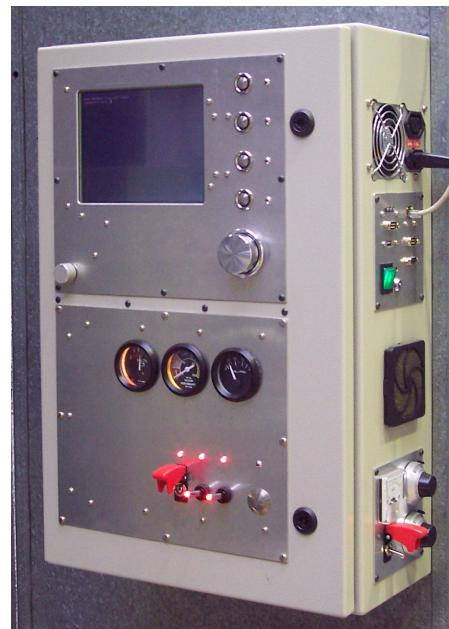
Figure 4.3: Operator control box mounted on the outside of the engine cell
