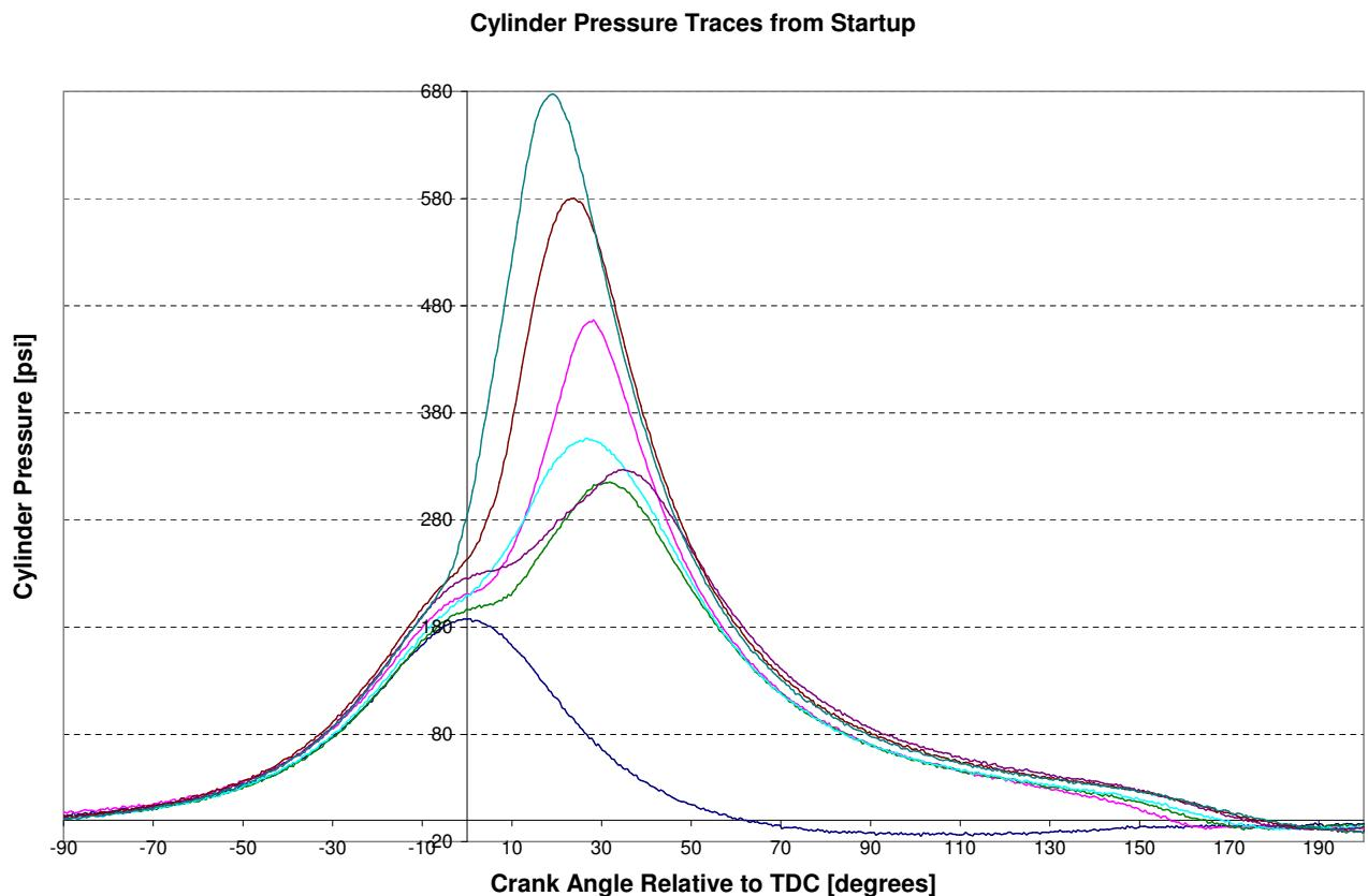
Figure 4.83: Cylinder pressure curves obtained during engine start-up
