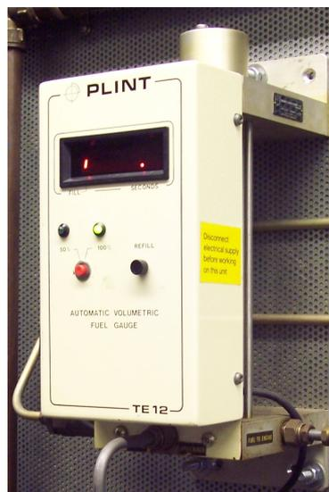
Figure 4.77: Plint TE12 volumetric fuel meter with digital range selection
