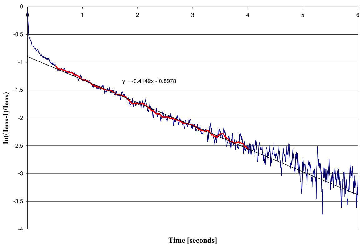
Figure 4.41: Natural logarithm of normalised field current for a 5 V transient
