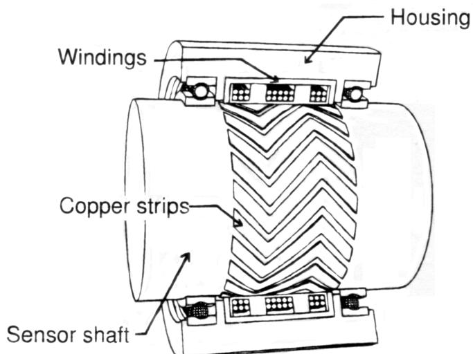
Figure 3.23: ABB's magnetoelastic torque sensor called a *Torductor*
