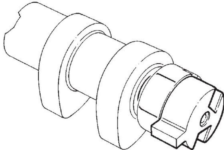
Figure 5.19: Camshaft timing ring (Jaguar, 1996)
