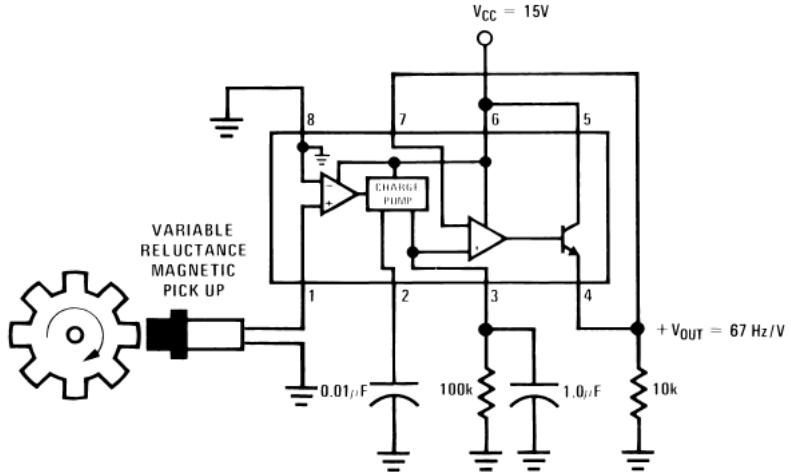
Figure 4.74: Typical tachometer circuit using the LM2907 IC (National-Semiconductor, 2000)
