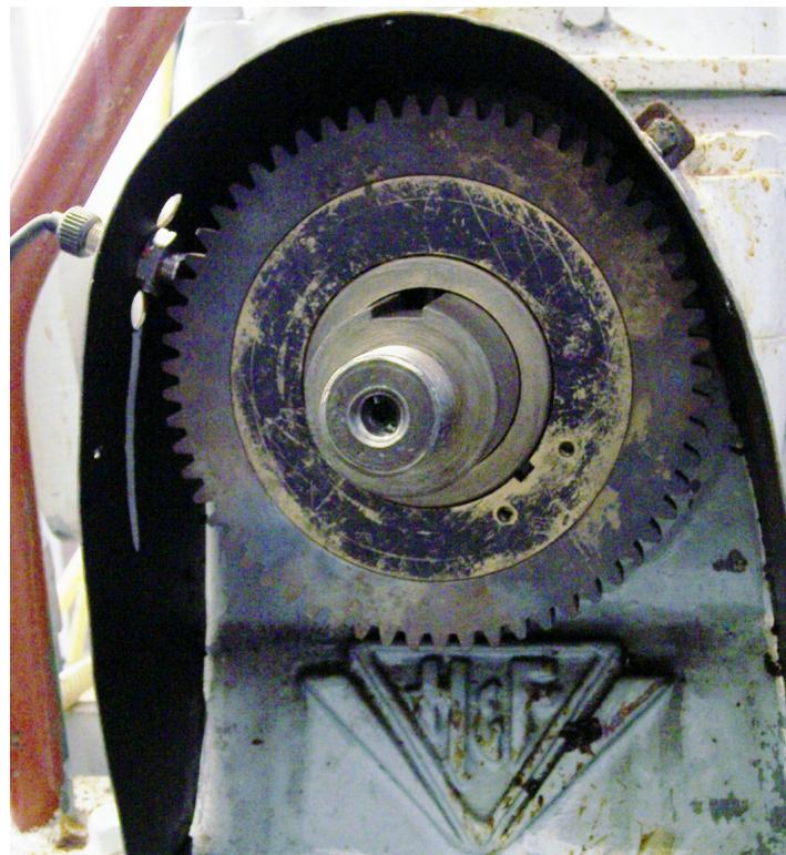
Figure 4.73: Dynamometer 60-tooth shaft-end gear and variable-reluctance sensor
