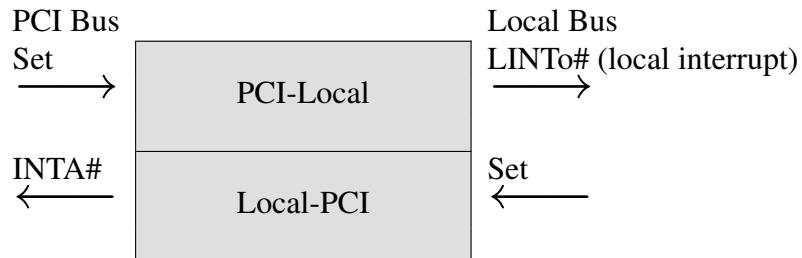
Figure B.8: PLX PCI 9056 32-bit doorbell registers
