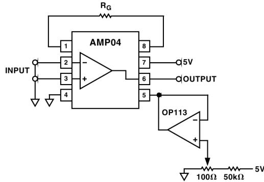
Figure 4.75: AMP04 offset nulling scheme (Analog-Devices, 2000)
