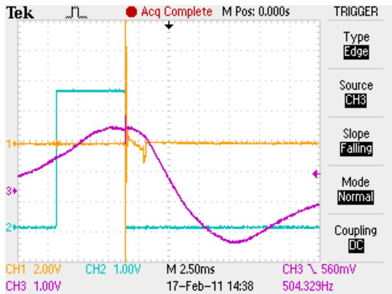
Figure 5.45: Camshaft key pulse to ignition phase. CH1 is the injector voltage, CH2 is the ignition trigger pulse for cylinder 4A from the ECU, and CH3 is from the camshaft sensor.
