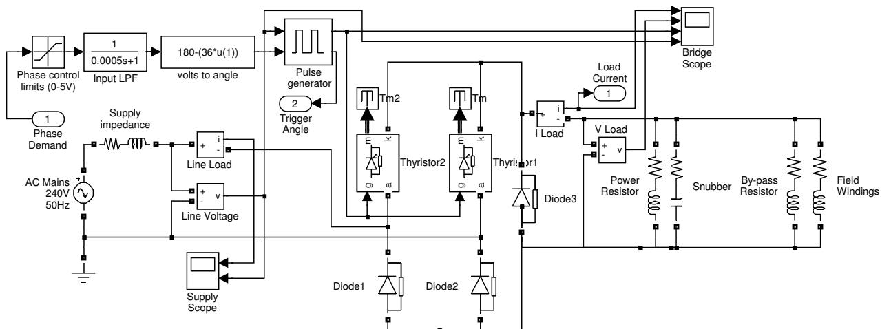
Figure 4.22: SCR bridge, phase angle control, supply and load
