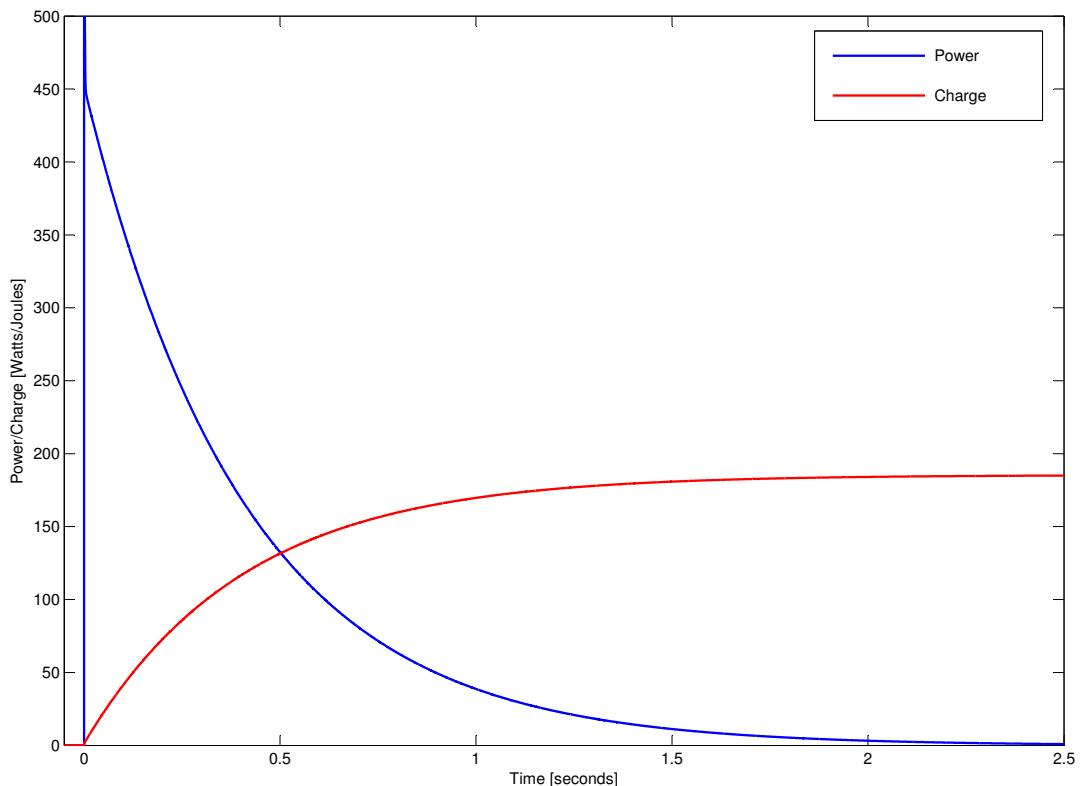
Figure 4.63: Plot of the modelled power dissipation and integrated charge in the external shunt resistor from maximum (4 A) to zero current
