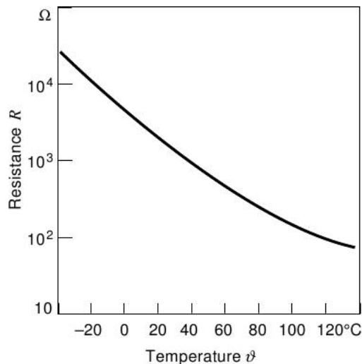
Figure 5.41: Typical automotive NTC thermistor characteristic
