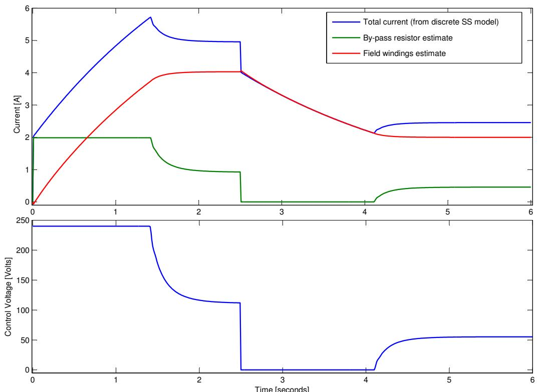
Figure 4.56: Plot of discrete controlled system response to step demand changes of 4 A ( $t=0$  seconds), and 2 A ( $t=2.5$  seconds)
