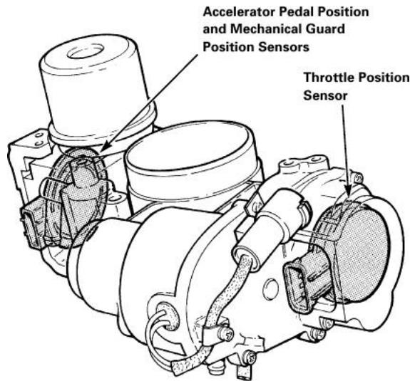
Figure 5.33: Electronic Throttle Sensors (Jaguar, 1996)
