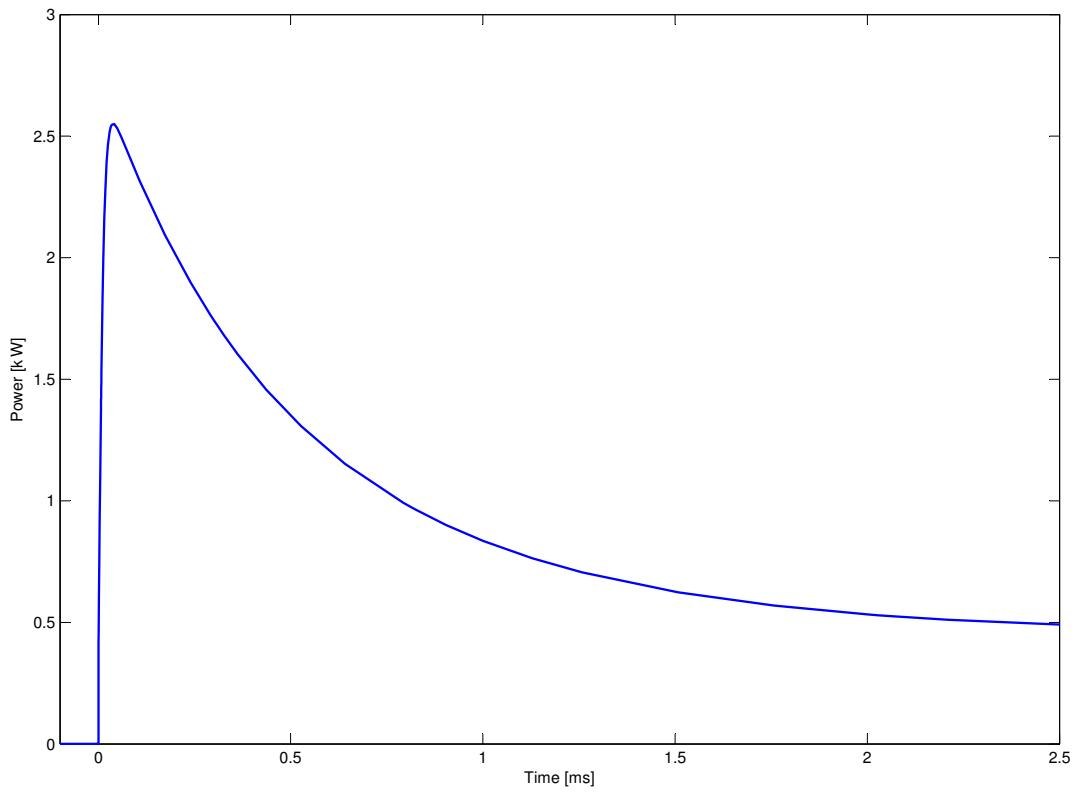
Figure 4.64: Plot of the modelled instantaneous peak power dissipation in the shunt resistor
