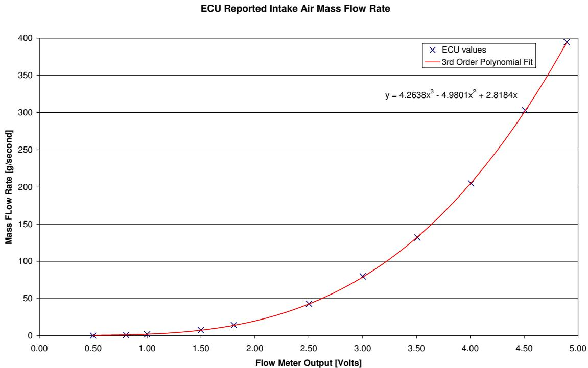
Figure 5.43: MAFS characteristic measured from the ECU
