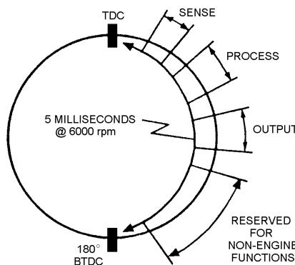
Figure 3.25: Crank angle representation of computer time usage (Mills, 1985)
