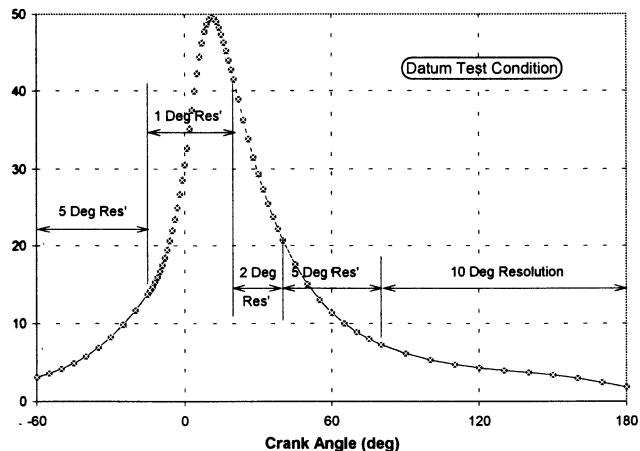
Figure 3.10: Mean cylinder pressure curve for datum test condition for reduced format resolution, showing the stored data points and the interpolated curve (Brunt et al., 2000)
