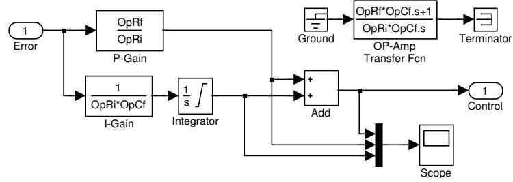
Figure 4.21: PI Controller subsystem
