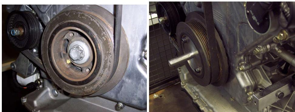
Figure 4.78: Engine crank pulley (left) fitted with adaptor for an encoder shaft (right)
