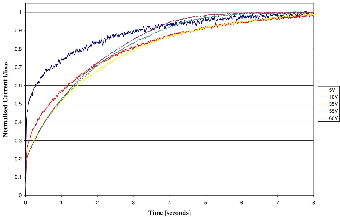
Figure 4.40: Normalised field current transients for several applied voltages
