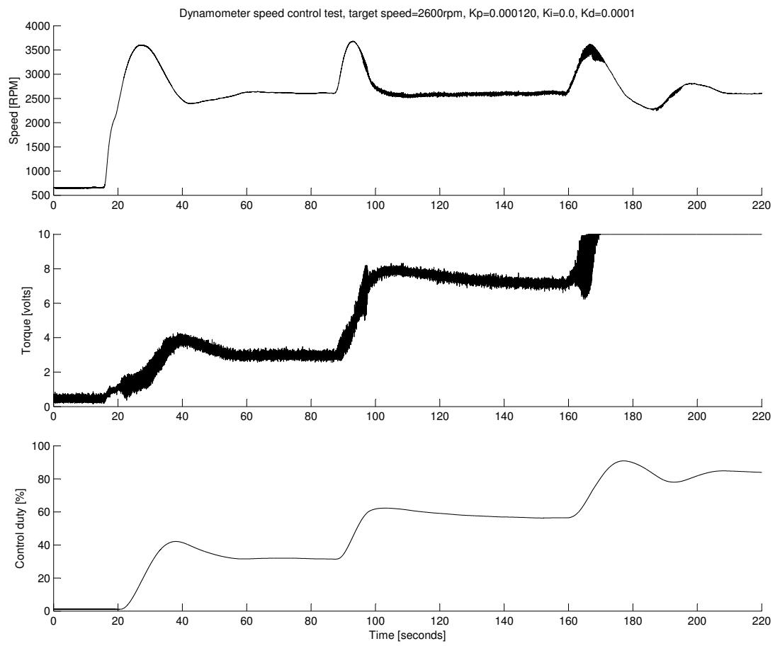
Figure 4.29: Plot of engine speed control test, low gain
