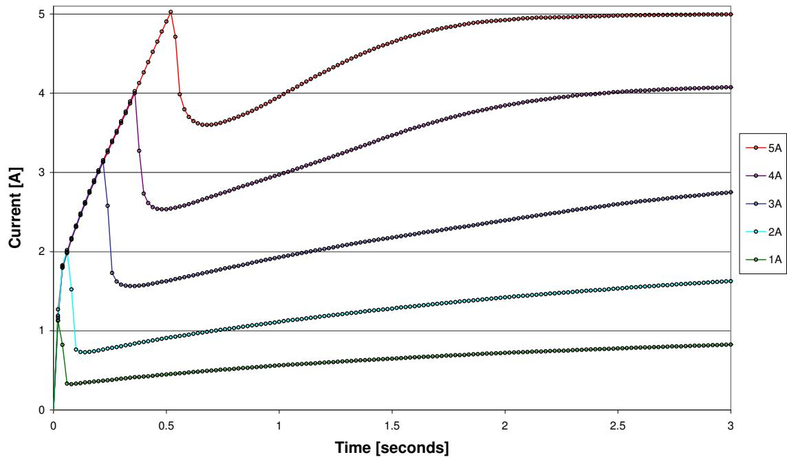
Figure 4.69: Open-loop response step decreases to voltage for equivalent steady-state current
