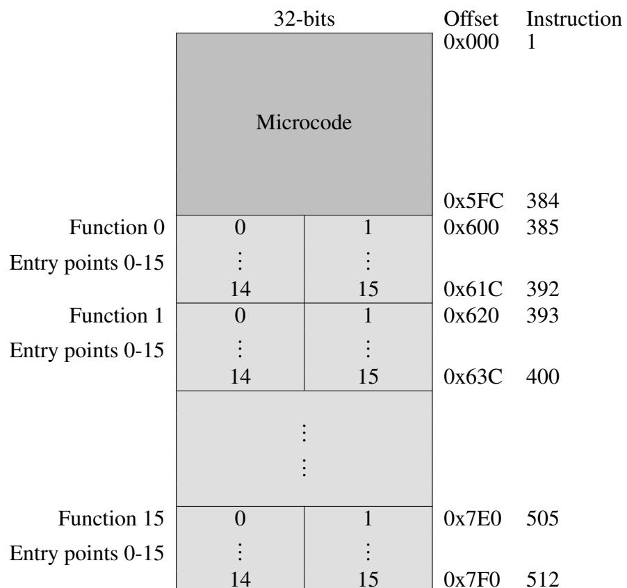
Figure B.6: Microcode and function entry point 2kB address region
