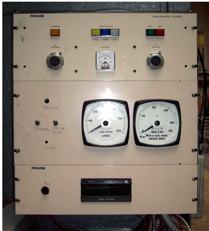
Figure 4.2: Froude operator's control panel for the dynamometer
