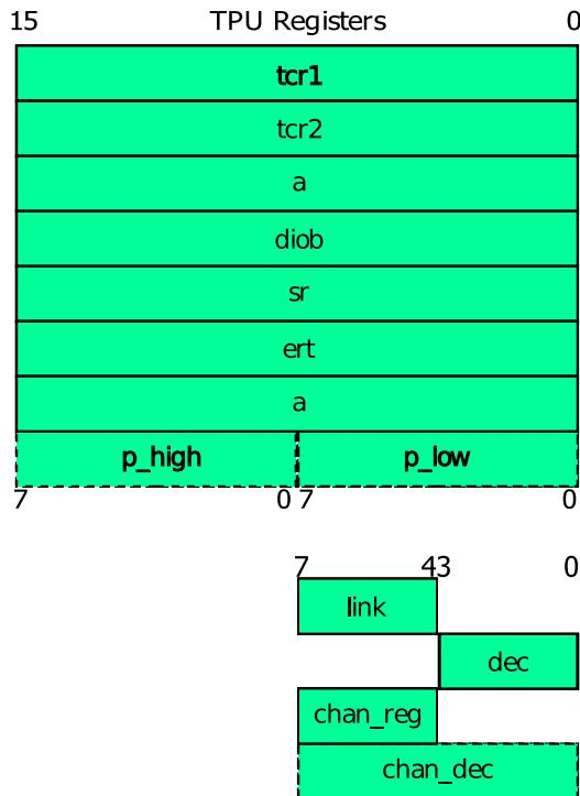
Figure B.5: Layout of the ten TPU User Registers
