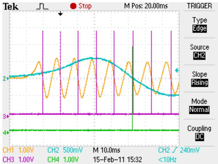
Figure 5.44: Camshaft to crankshaft phase shown from dual LM1815 outputs. CH1 from is the flywheel sensor and CH3 the zero crossing detection pulse, CH2 is from the camshaft sensor and CH4 shows the corresponding detection pulse.
