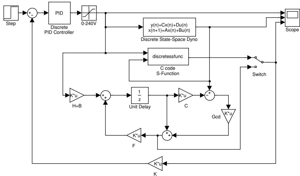
Figure 4.55: Discrete plant and controller with C coded estimator block diagram
