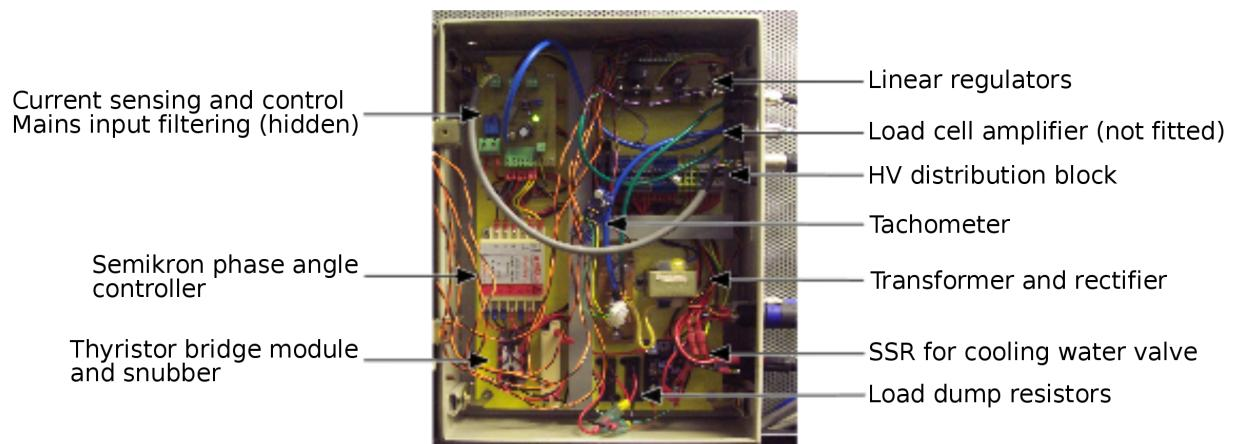
Figure 4.4: Dynamometer power electronics and signal conditioning box
