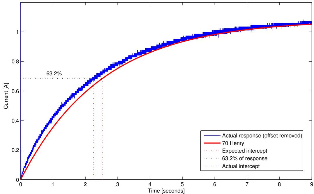
Figure 4.33: Measured 30V DC step response, plotted with step offset removed to estimate time constant
