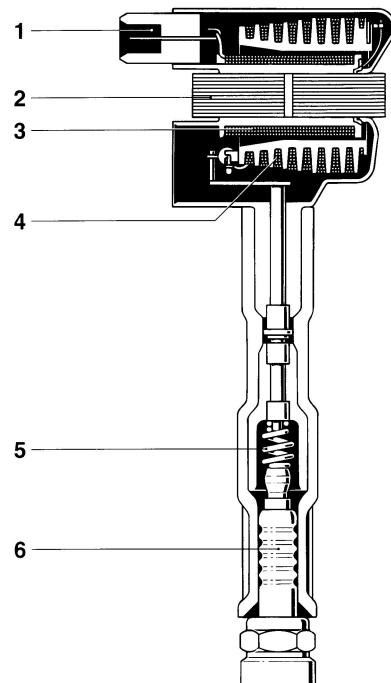
Figure 5.16: Coil-on-plug assembly (Steinbrenner et al., 1994), 1) LV terminal 2) Multiplate iron core 3) Primary winding 4) Secondary winding 5) HV terminal 6) Spark plug
