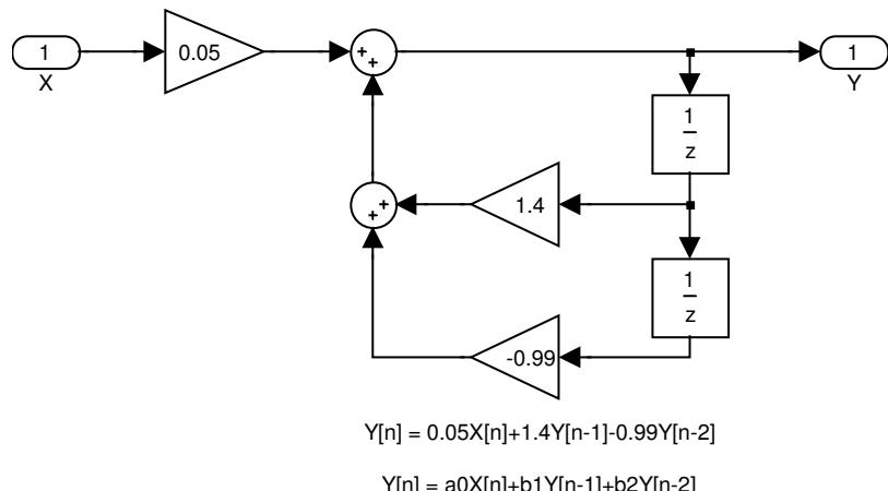
Figure 5.27: IIR Band-pass Simulink representation
