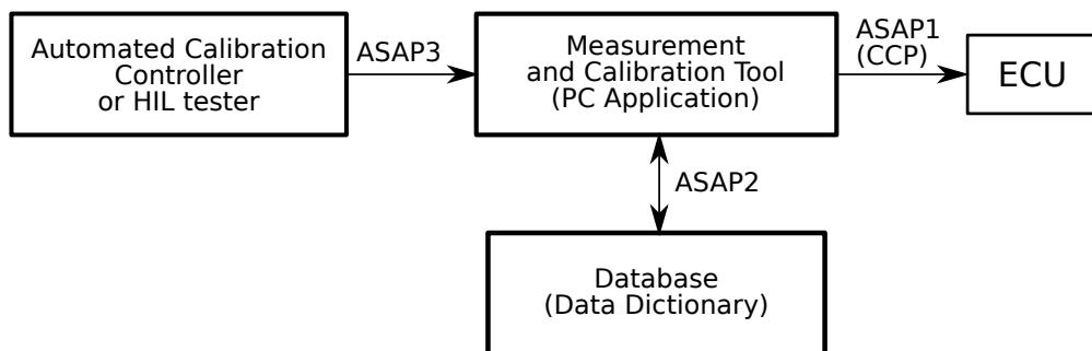
Figure 5.8: The relationship between the ASAP interfaces
