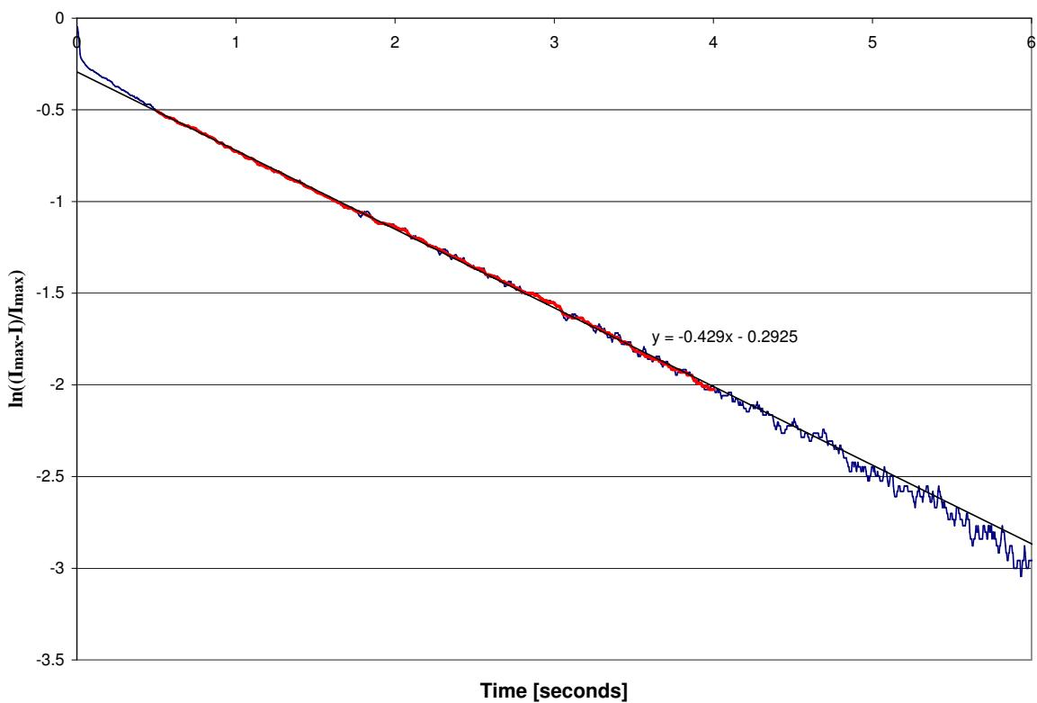
Figure 4.42: Natural logarithm of normalised field current for a 35 V transient
