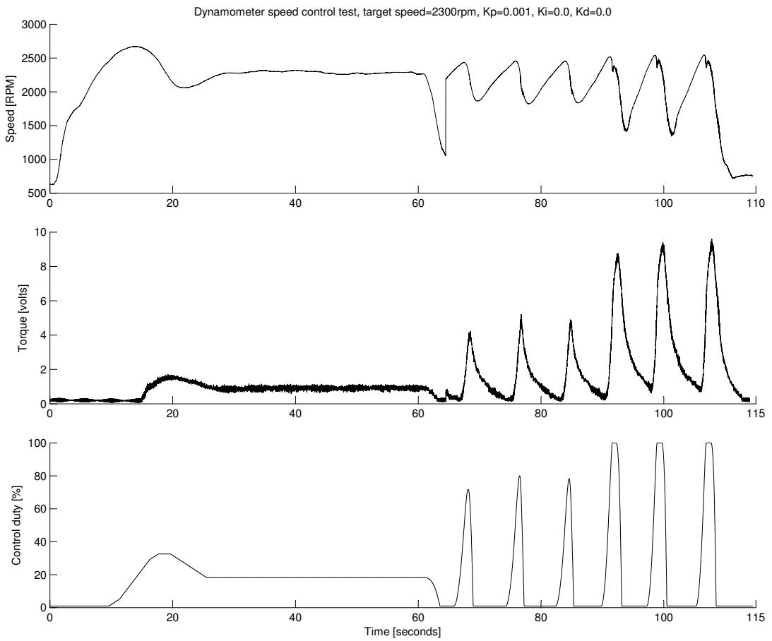
Figure 4.30: Plot of engine speed control test, high gain
