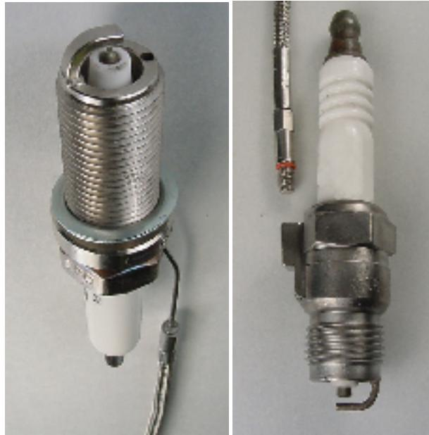
Figure 3.20: CALplug (left) and PSIplug (right) modified spark plugs using an optical pressure sensor
