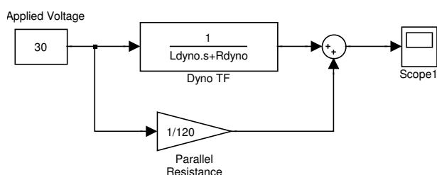
Figure 4.31: Block diagram of the simple DC step response model
