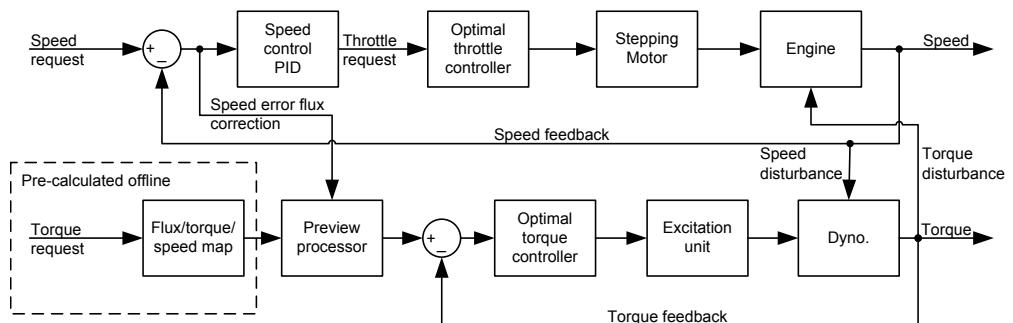
Figure 3.7: Block diagram of mode 2, torque and speed tracking with preview. (Koureas & Watson, 1984)
