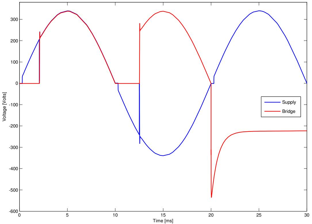
Figure 4.62: SCR bridge voltage spike occurring when a resistor is switched into the circuit at the full current rating
