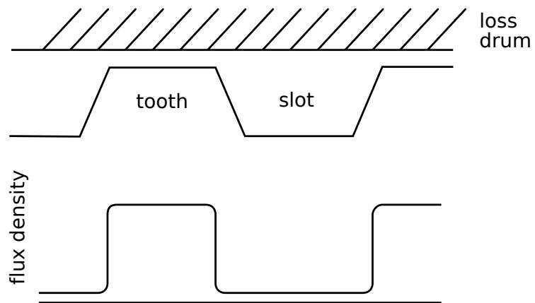
Figure 3.2: Eddy-current coupling static air-gap flux distribution (Davies, 1966)
