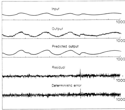
Figure 3.13: Estimation results using NARMAX input-output model compared with the original data set
