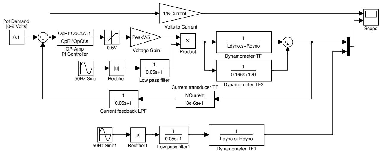
Figure 4.24: Block diagram of simplified current controller model
