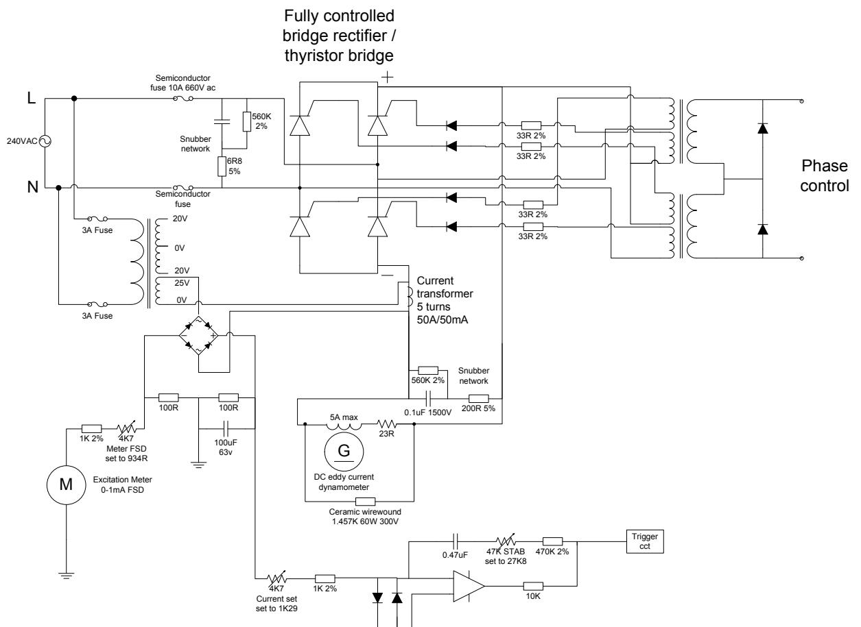
Figure 4.11: Simplified schematic of the original current controller
