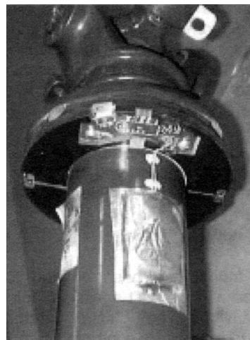
Figure 3.21: Propeller shaft fitted with strain gauges (Sandberg, 2001)
