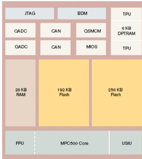
Figure 5.9: Block diagram of MPC555 internal features
