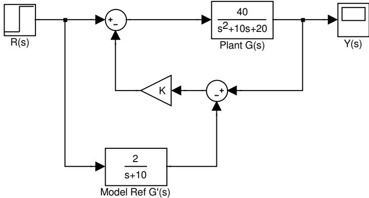
Figure 2.5: SIMULINK block diagram of a simple example MRAC scheme (Dutton et al., 1998)
