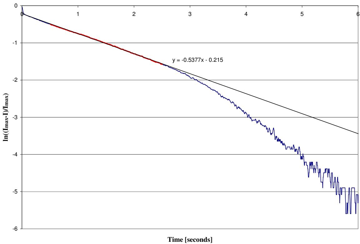
Figure 4.44: Natural logarithm of normalised field current for a 60 V transient
