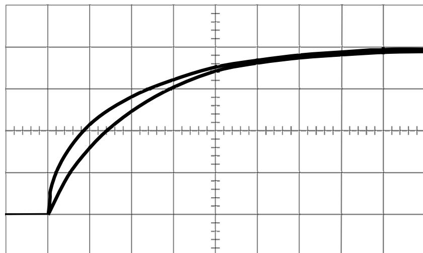
Figure 3.3: Eddy current coupling current (upper trace) and flux (lower trace) response at standstill (Wright, 1972). 20 ms timebase, arbitrary vertical scale
