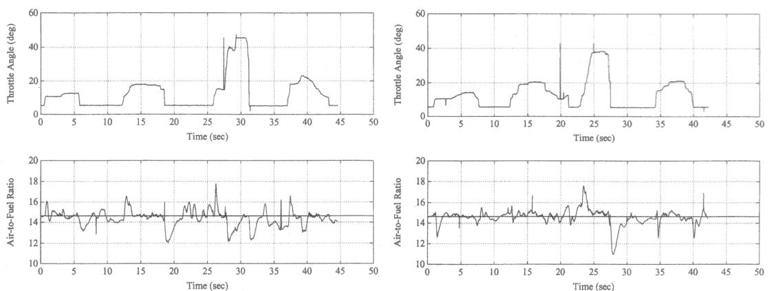
Figure 3.16: Throttle and A/F ratio control using the standard ECM (left) and using the proposed CMAC controller (right) under random driving conditions (Shiraishi et al., 1995)
