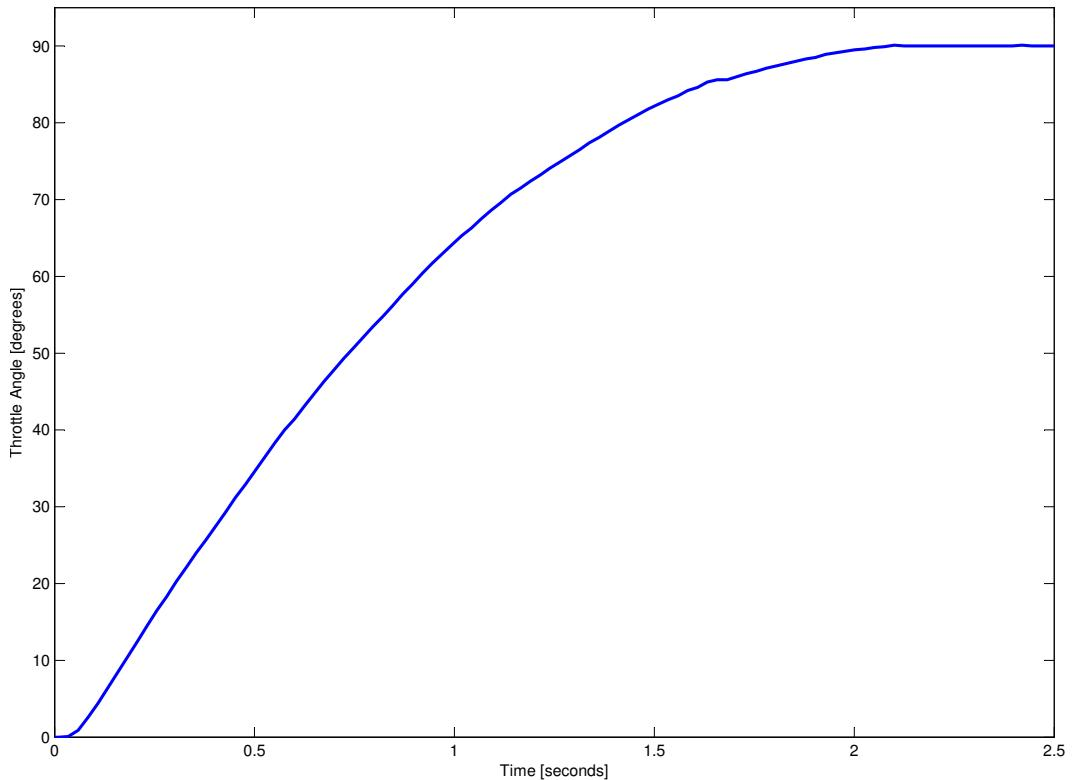
Figure 5.38: Throttle plate opening under spring action alone
