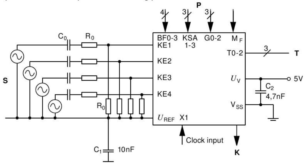
Figure 5.26: Bosch CC195 knock signal conditioner internal schematic
