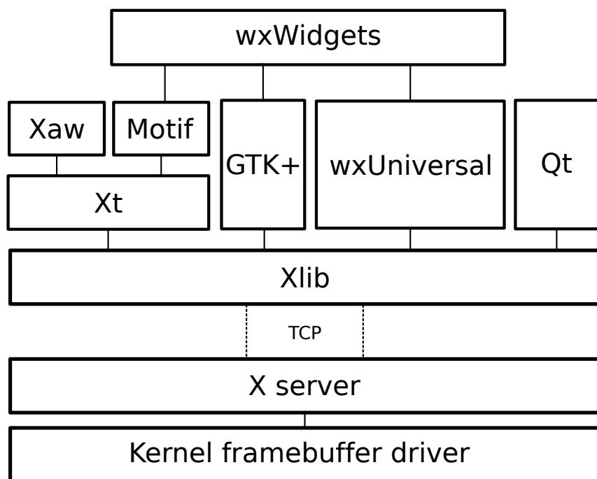
Figure B.3: wxWidgets and X Window System and widget toolkit stack
