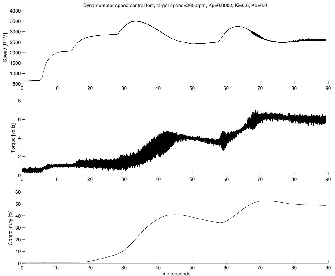
Figure 4.28: Plot of engine speed control test, medium gain
