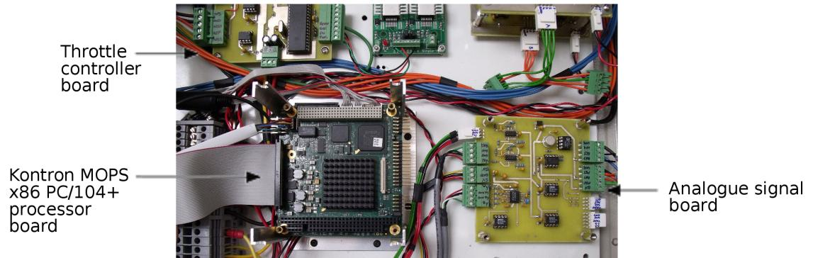
Figure 5.4: Inside the research ECU box showing the MOPS embedded PC and analogue signal board
