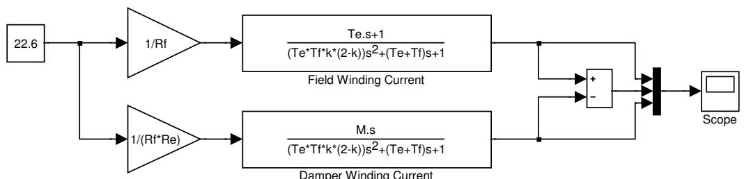
Figure 4.46: Transfer functions for applied voltage to field winding and damper winding current
