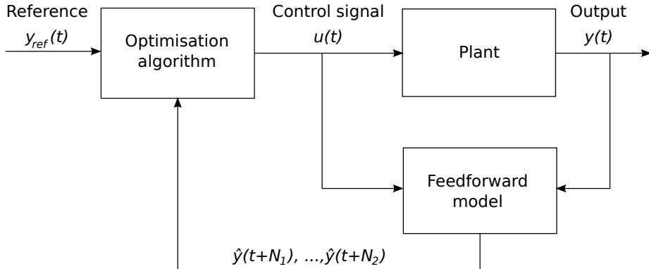
Figure 2.7: General structure of a model-based predictive controller (Barreto & Araujo, 2004)
