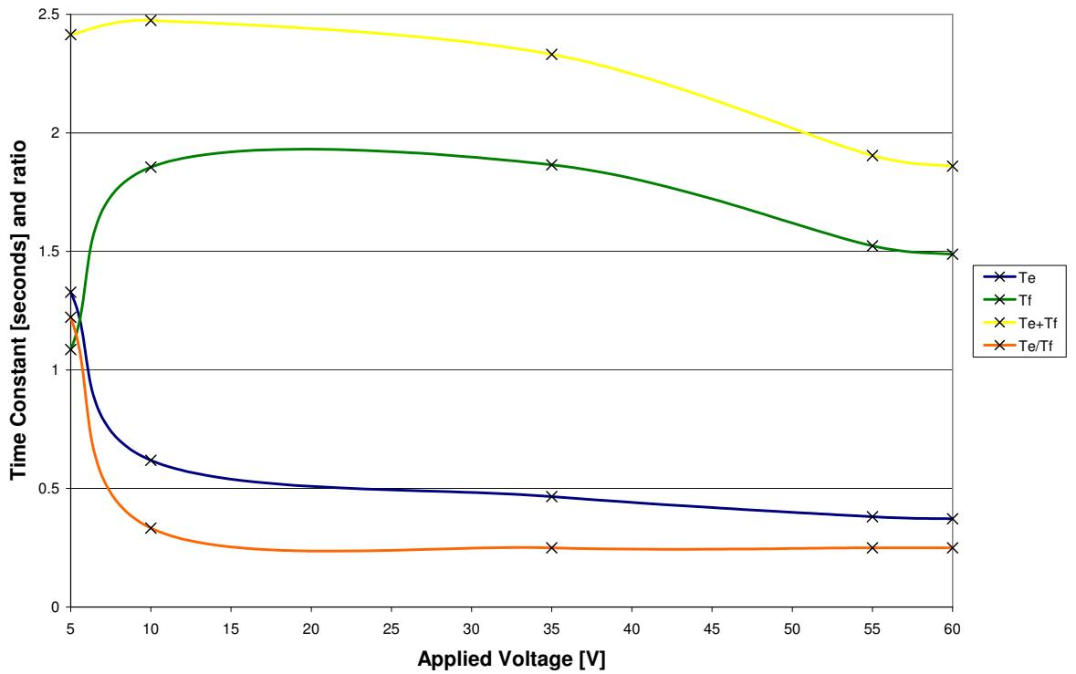
Figure 4.45: Time constant variation for several applied voltages
