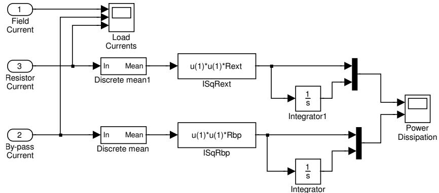
Figure 4.60: Current monitoring subsystem block diagram
