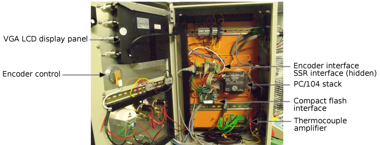
Figure 4.9: Inside the pendant operator's box
