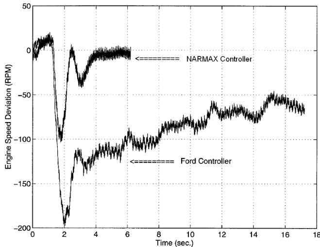
Figure 3.14: Comparison of the experimental response of on-board Ford idle speed controller with a NARMAX controller to a 20 Nm step load torque disturbance
