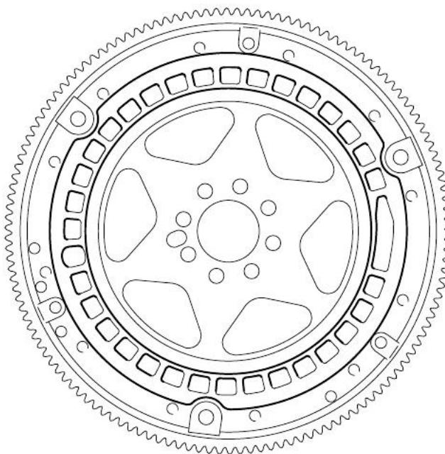
Figure 5.18: AJ-V8 flywheel embedded timing disc (Jaguar, 1996)
