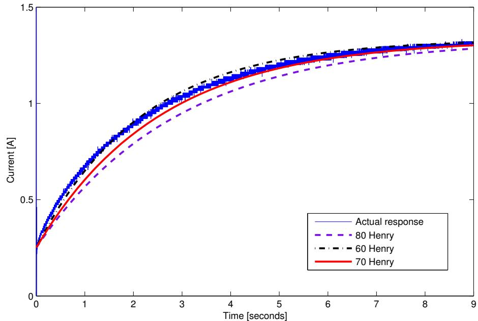
Figure 4.32: Dynamometer winding measured response to 30V DC step input plotted against different simulated responses
