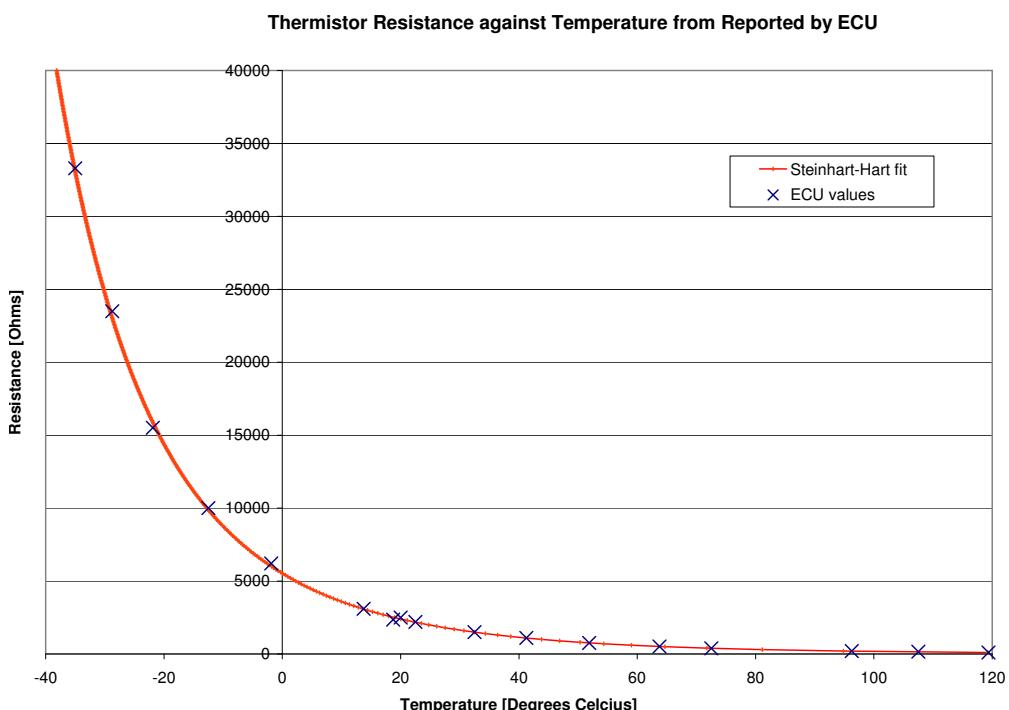
Figure 5.42: NTC thermistor characteristic measured from the ECU
