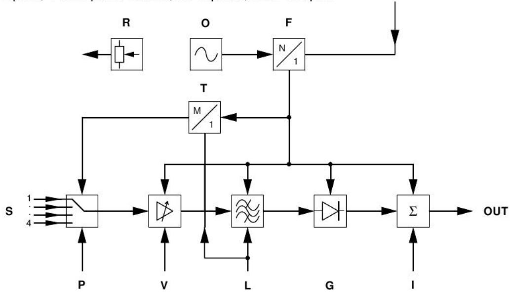
Figure 5.25: Bosch CC195 knock signal conditioner internal schematic
