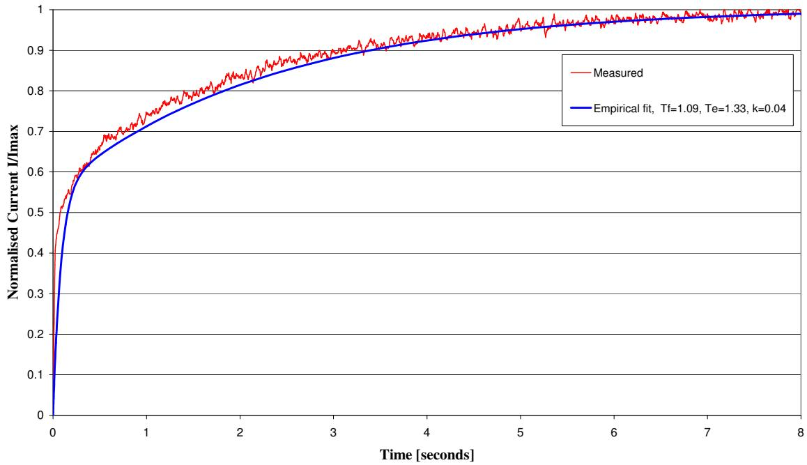
Figure 4.47: Modelled and measured normalised current responses to a 5 V applied voltage
