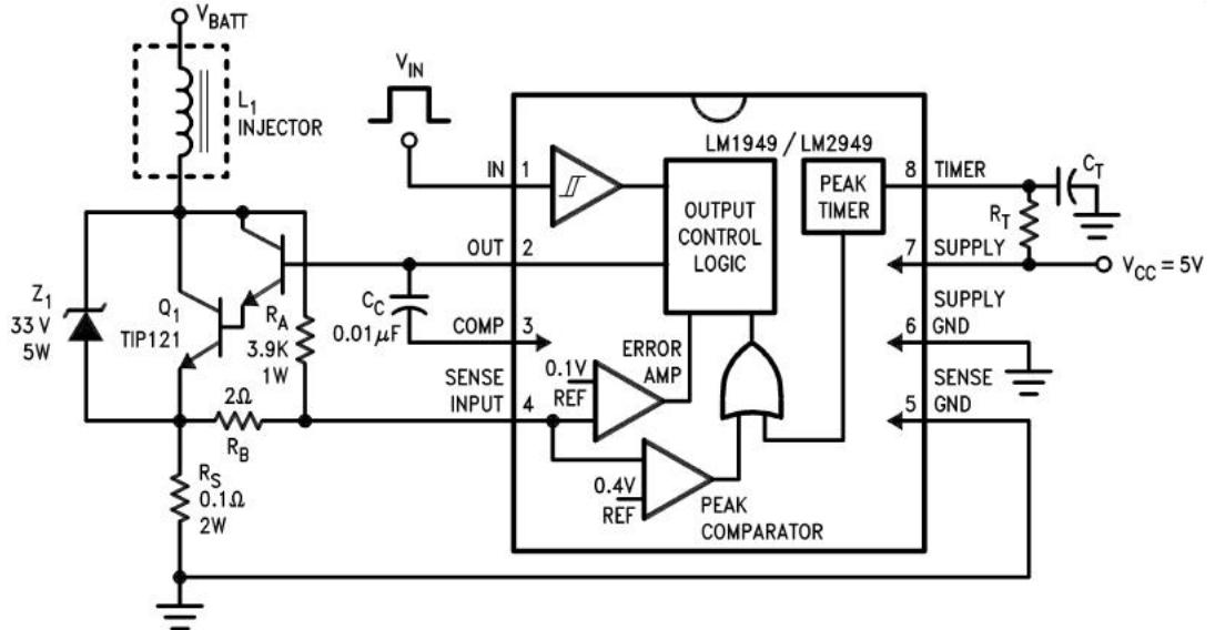
Figure 5.12: Injector drive controller typical application circuit (National-Semiconductor, 1995)
