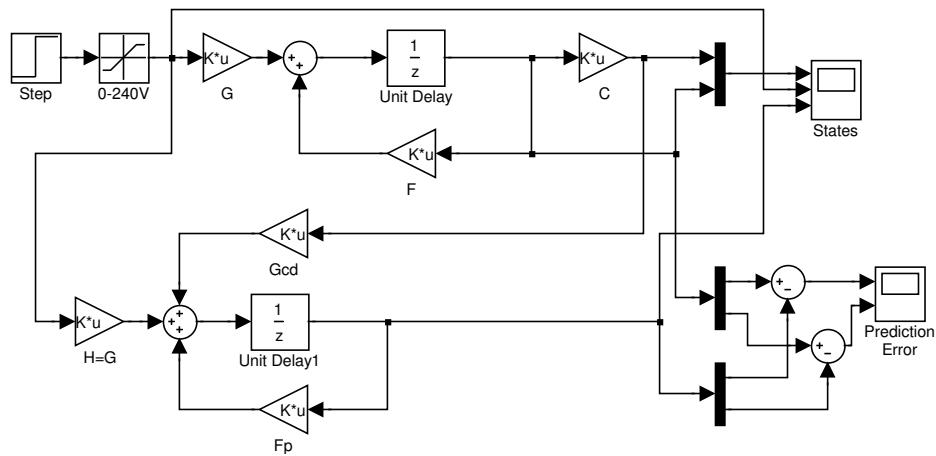
Figure 4.54: Discrete plant and estimator block diagram
