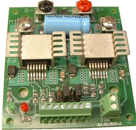
Figure 5.36: Simple-H driver board
