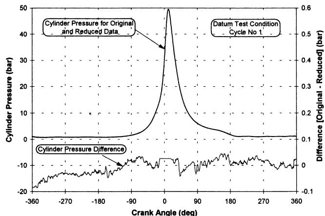
Figure 3.11: Typical comparison of cylinder pressure vs. crank angle curves for original and reduced cylinder pressure, difference is shown in lower region of the plot (Brunt et al., 2000)
