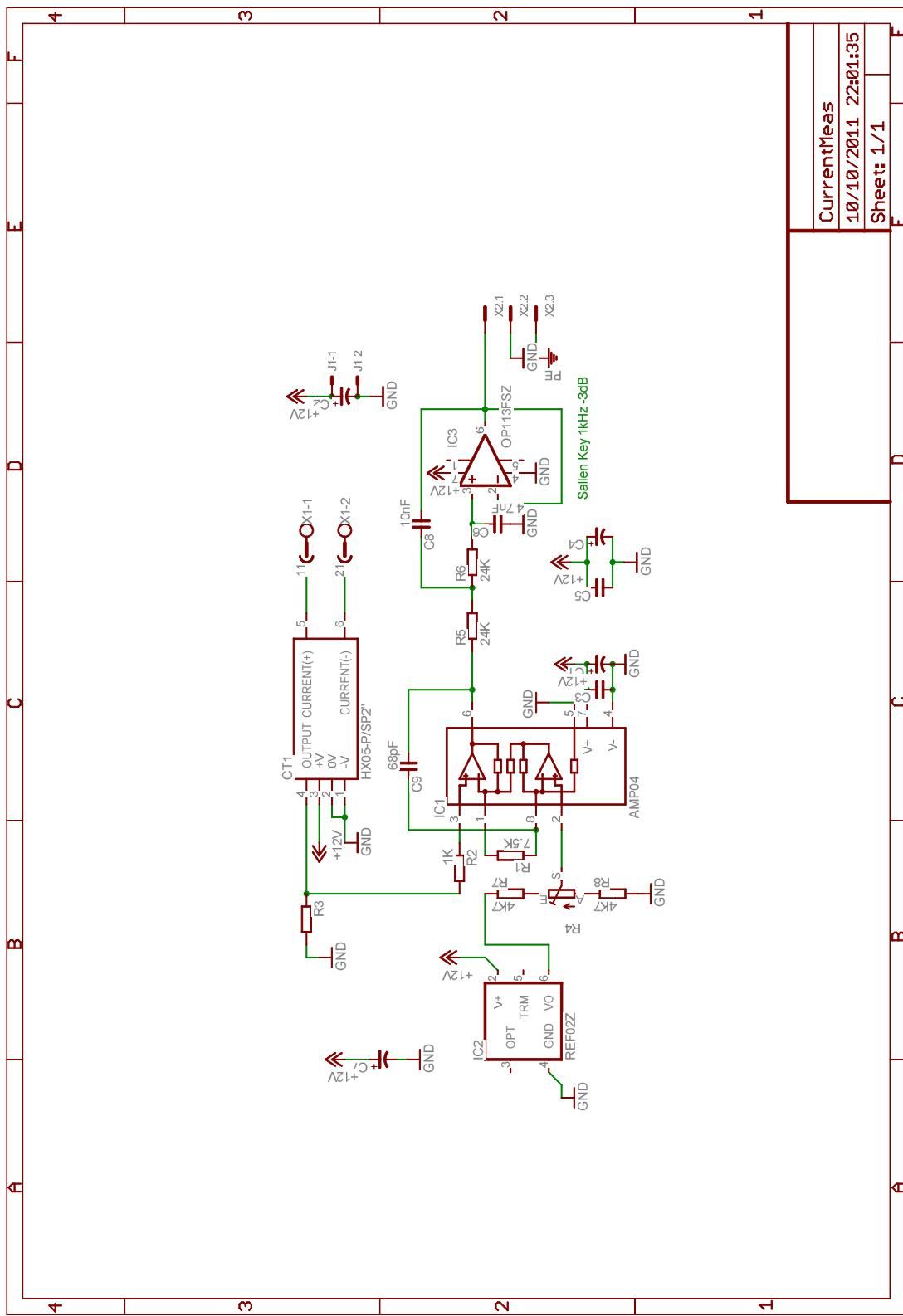
Figure A.9: Current transducer board circuit schematic
