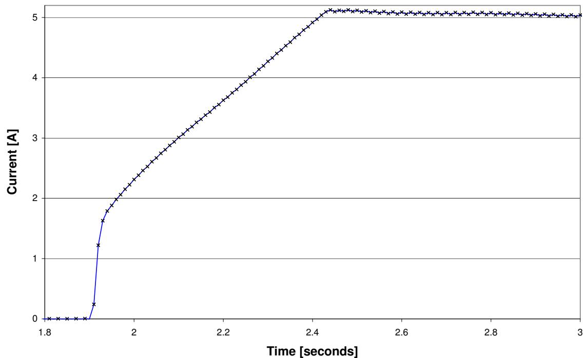
Figure 4.65: Step response to a full scale 5 A demand change
