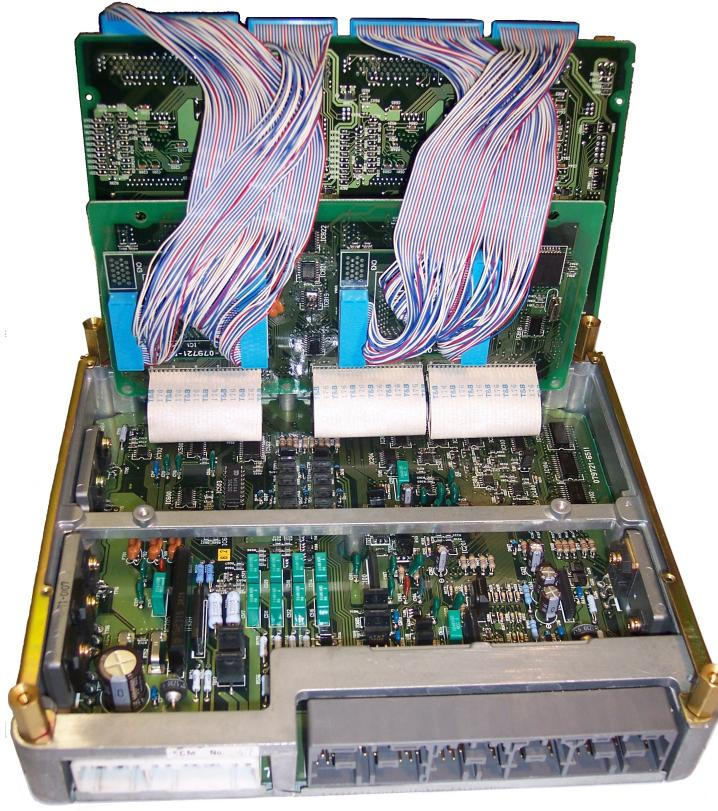
Figure 5.5: Nippon Denso ECM, middle and lower PCBs visible
