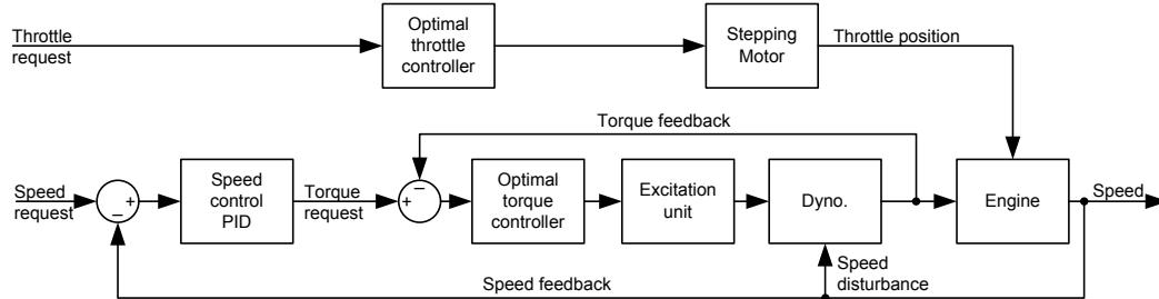
Figure 3.9: Block diagram of mode 5, control of speed using torque. (Koureas & Watson, 1984)
