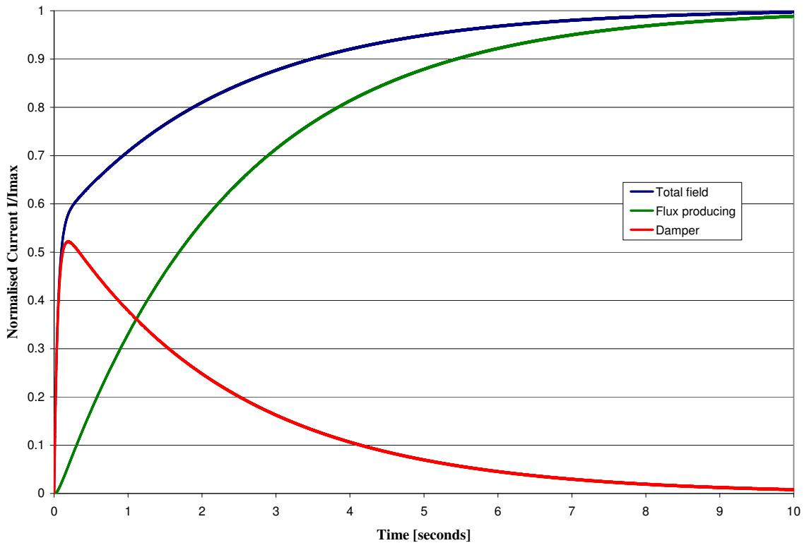
Figure 4.49: Modelled current winding responses and predicted flux current
