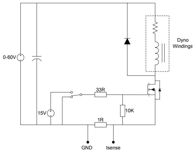
Figure 4.35: FET based step test circuit
