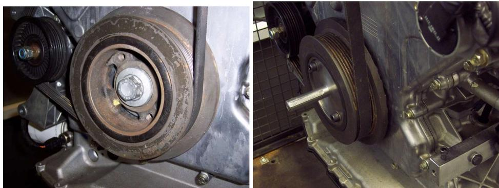
Figure 4.78: Engine crank pulley (left) fitted with adaptor for an encoder shaft (right)
