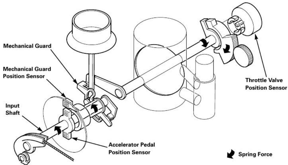
Figure 5.31: Simplified diagram of the electronic throttle unit (Jaguar, 1996)
