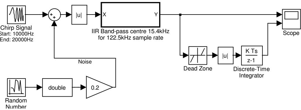
Figure 5.28: Knock detection example model
