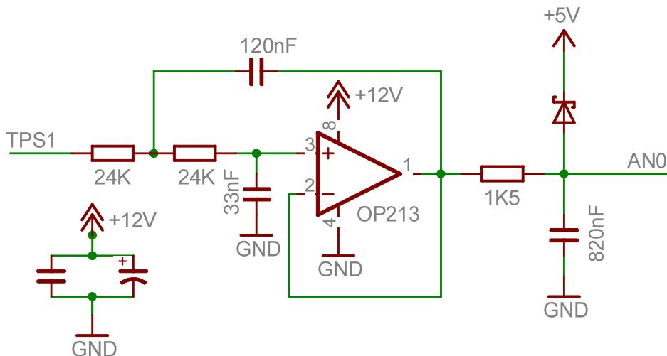
Figure 5.34: Active input filter schematic diagram
