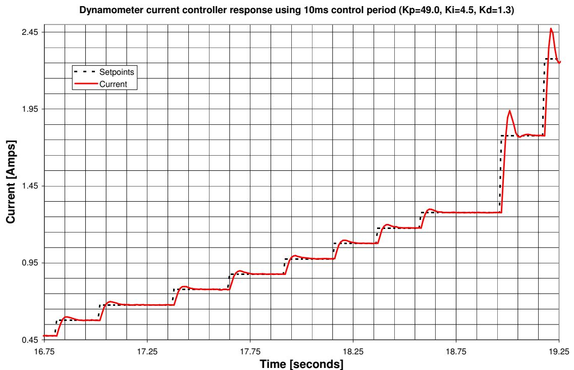
Figure 4.66: Response to incremental step increases in controller demand current
