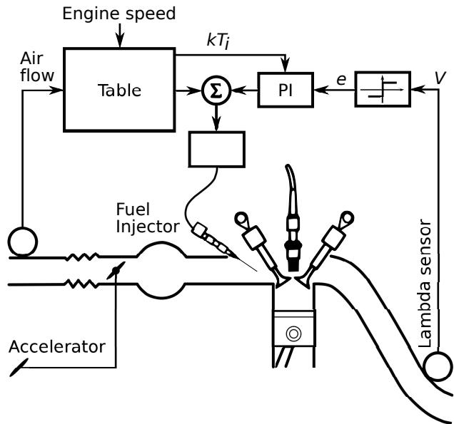
Figure 2.2: Engine mapping shown as a form of Gain Scheduling
