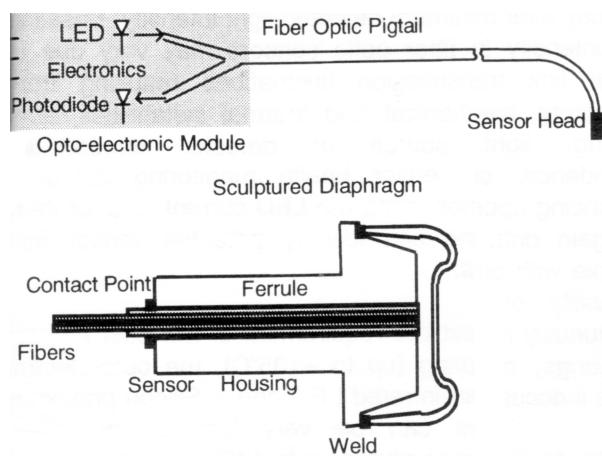
Figure 3.19: Schematic of optical pressure sensor construction (Ulrich et al., 2001)
