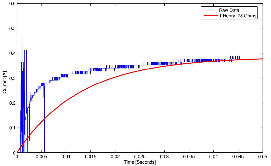
Figure 4.34: Plot of an expansion of the initial step in full response. A parallel resistance with some inductance is shown for comparison.
