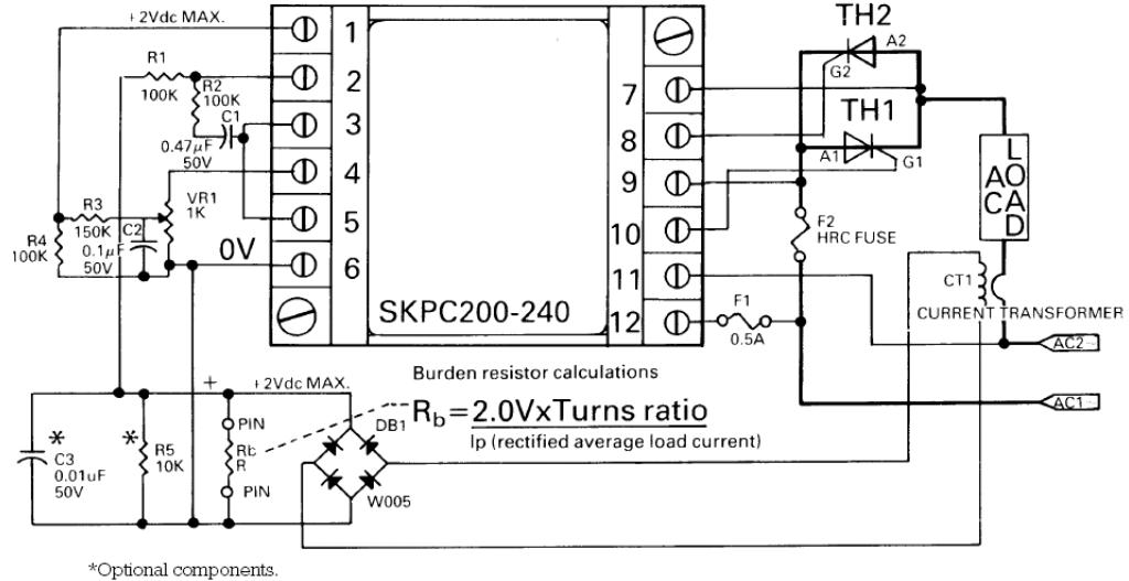
Figure 4.15: Semikron current control circuit for an AC load
