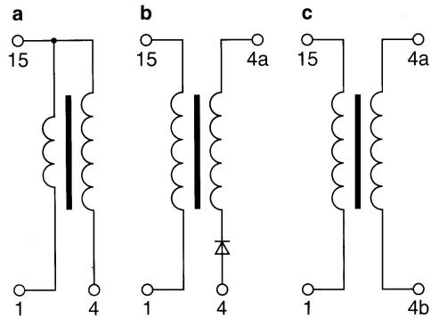
Figure 5.15: The three main types of ignition coil (Steinbrenner et al., 1994). a) Conventional single spark coil used with a distributor. b) single spark coil (coil-on-plug) c) dual spark coil (wasted spark)
