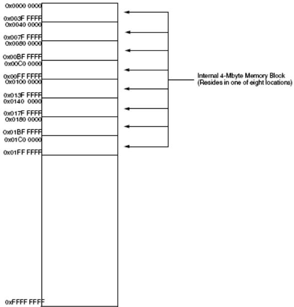
Figure B.9: Diagram of the eight possible IMMR locations within the full address space
