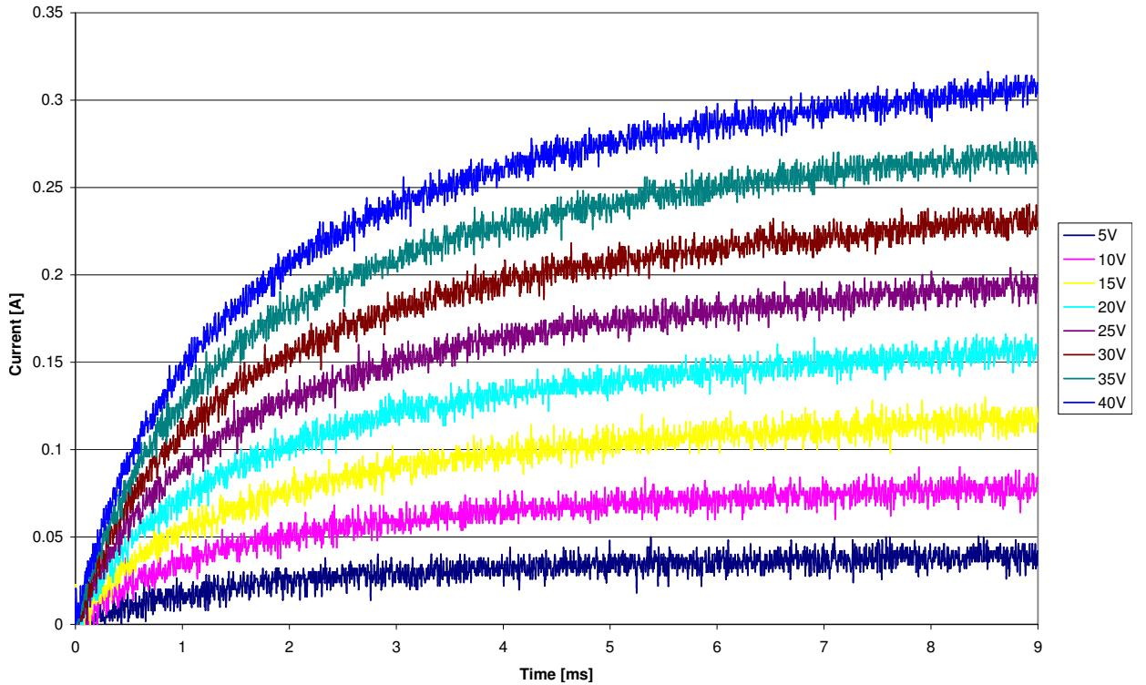
Figure 4.37: Initial rise in field current for a range of applied voltages
