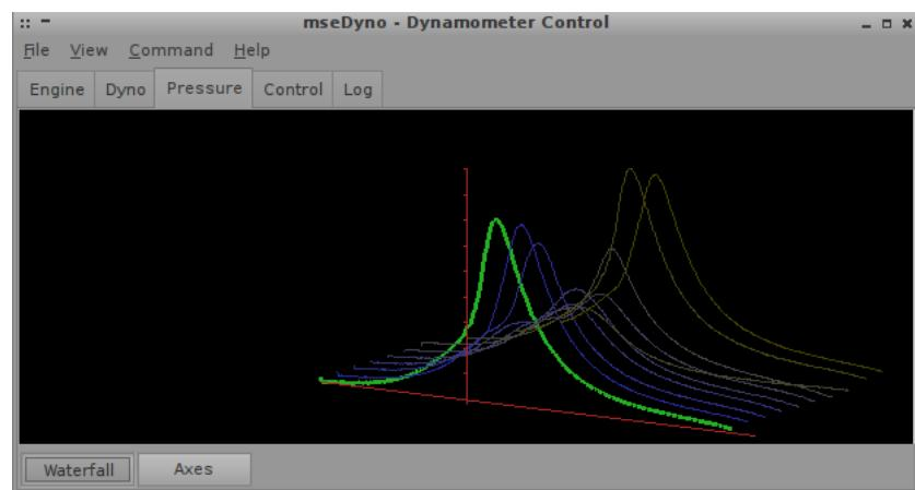
Figure 4.87: The mseDyno front end GUI showing the pressure plotter panel
