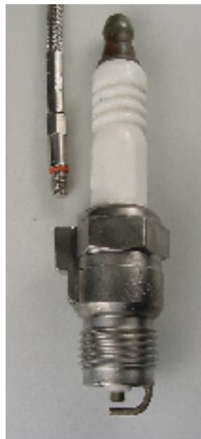
Figure 4.80: Optrand PSIplug and M3.5 sensor
