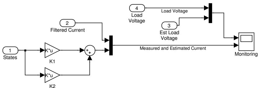
Figure 4.58: Monitoring subsystem block diagram
