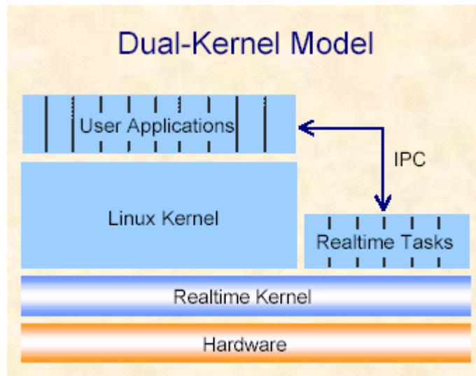
Figure B.1: RTLinux dual kernel model
