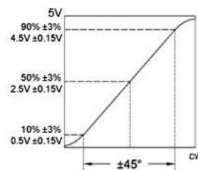
Figure 5.32: Rotary hall effect potentiometer characteristic (P3-America, 2005)
