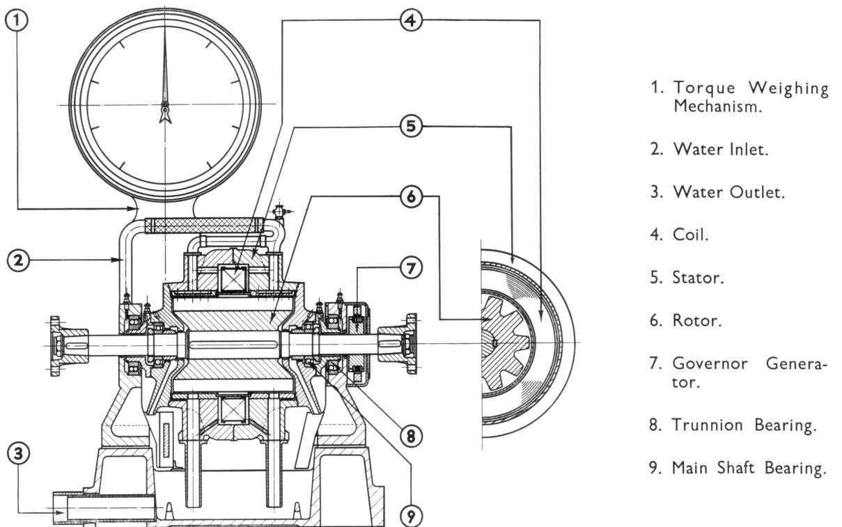
Figure 4.10: Heenan Froude G.V.A.L. Mk1 dynamometer cross-section
