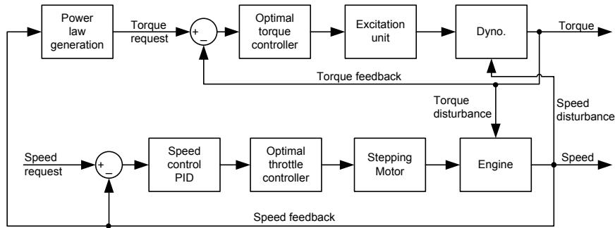
Figure 3.8: Block diagram of mode 4, power-speed law. (Koureas & Watson, 1984)
