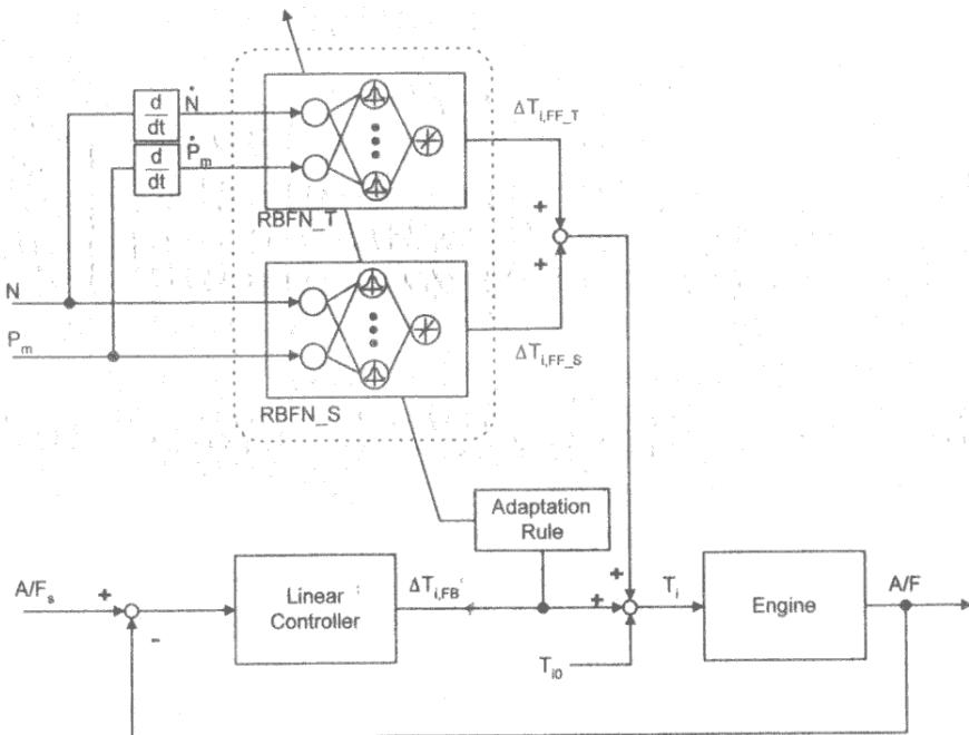
Figure 3.17: Radial Basis Function augmented controller (Park et al., 2003)
