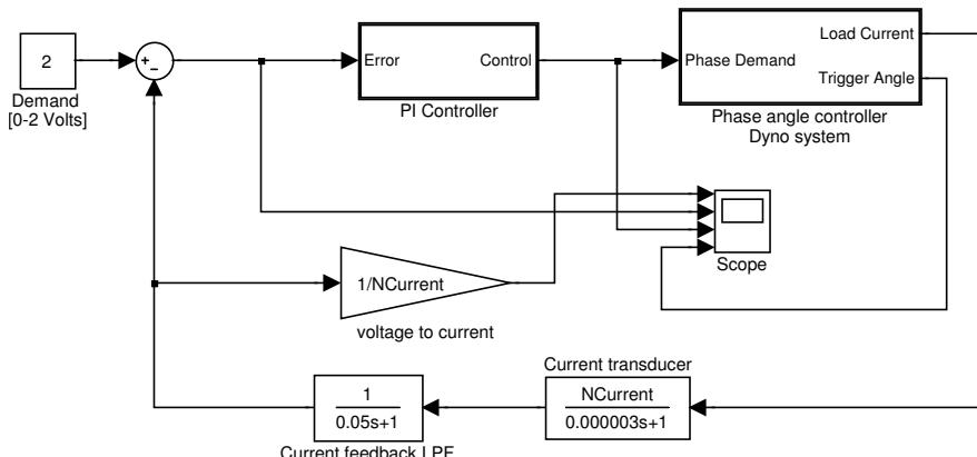
Figure 4.20: Top level of the control system model
