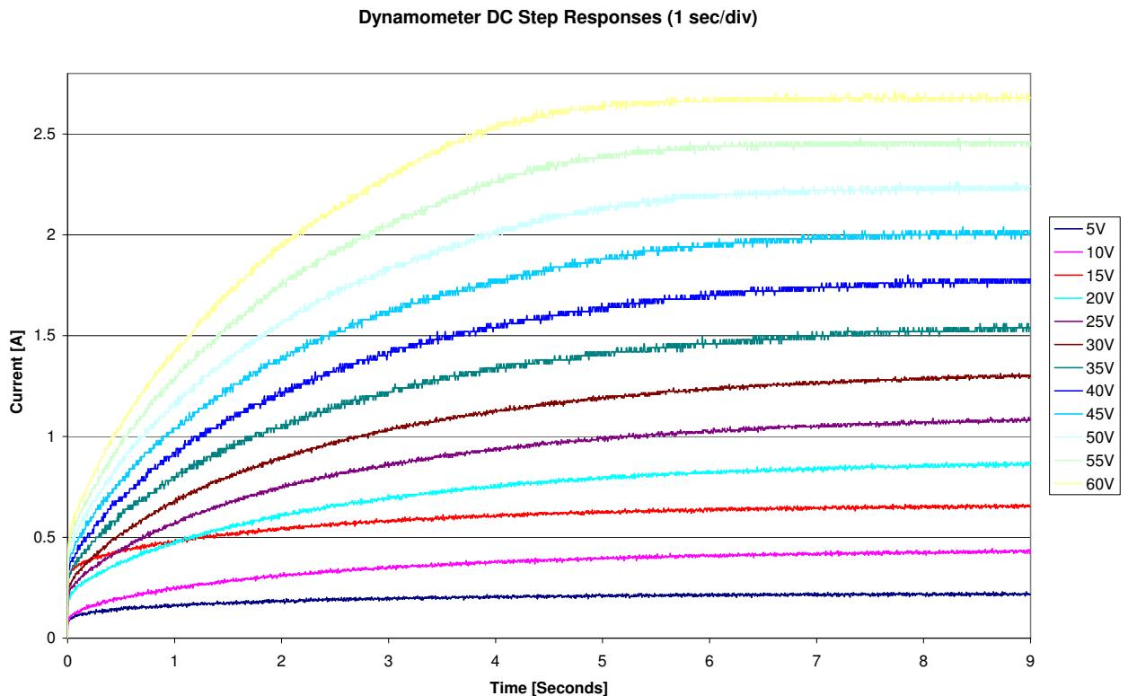
Figure 4.36: Field current step response to steady-state for a range of applied voltages
