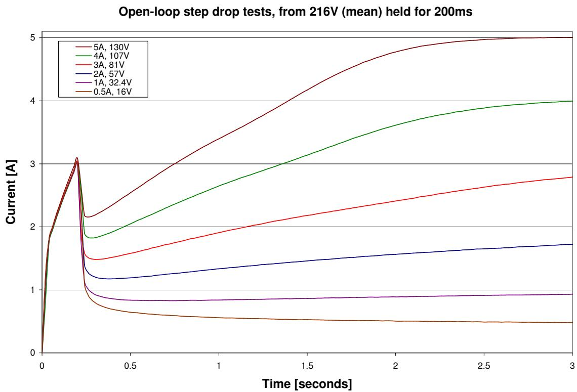
Figure 4.67: Open-loop response step decreases in applied
