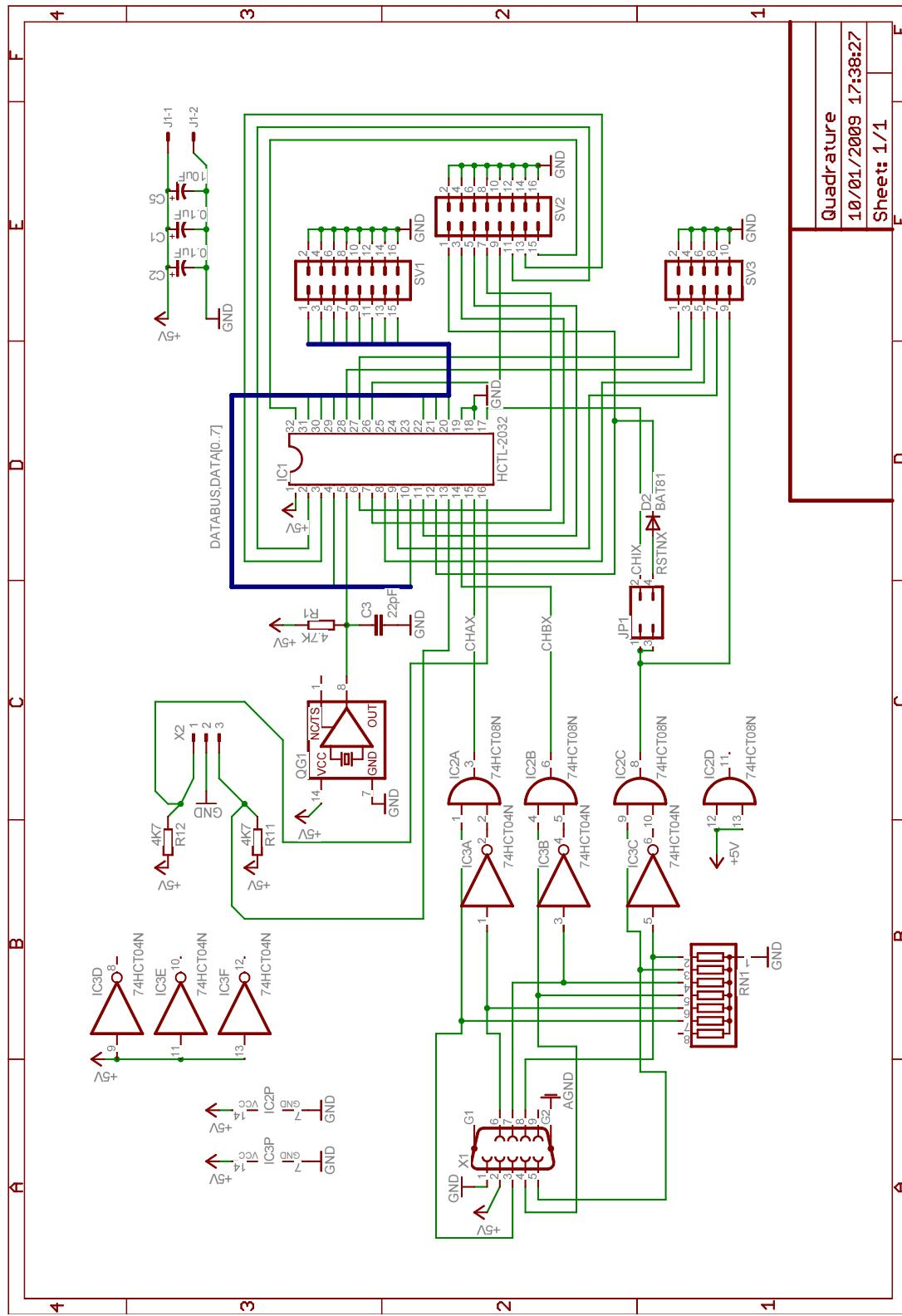
Figure A.7: Encoder quadrature interface circuit schematic
