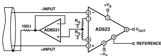
Figure 4.76: Common-mode shield driver (Analog-Devices, 1999b)
