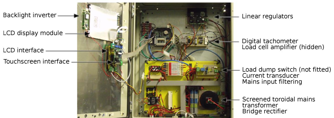
Figure 4.7: Dynamometer power electronics and control box inside view
