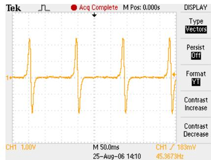
Figure 5.21: Camshaft variable reluctance sensor output
