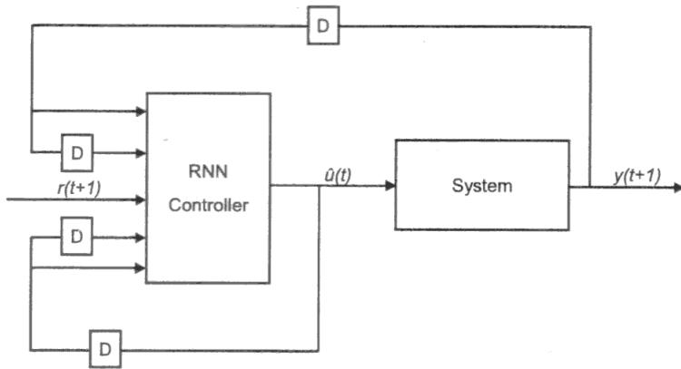
Figure 2.11: Direct Inverse Model structure: The controller performs the control action one time step later than the desired target
