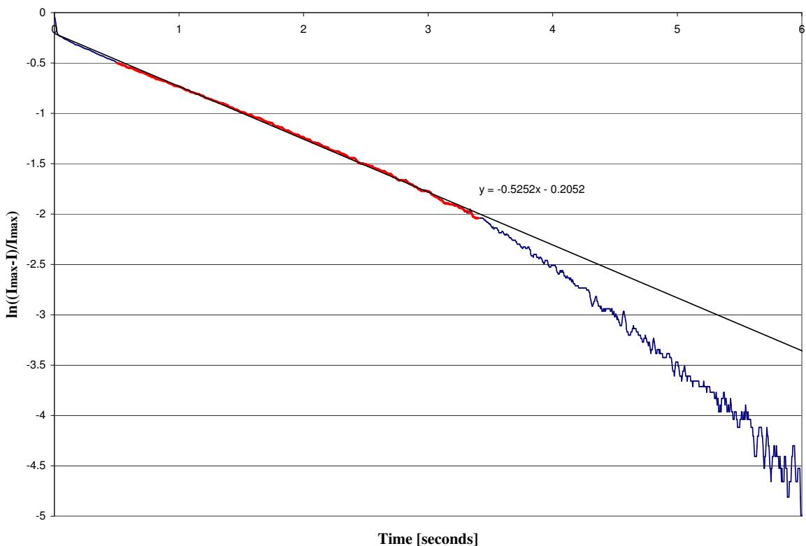
Figure 4.43: Natural logarithm of normalised field current for a 55 V transient
