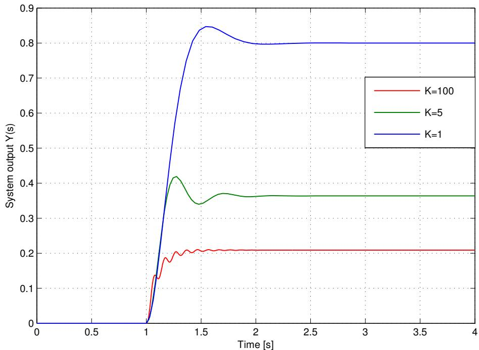
Figure 2.6: Example MRAC step responses for various gains showing decaying higher order oscillation (Dutton et al., 1998)
