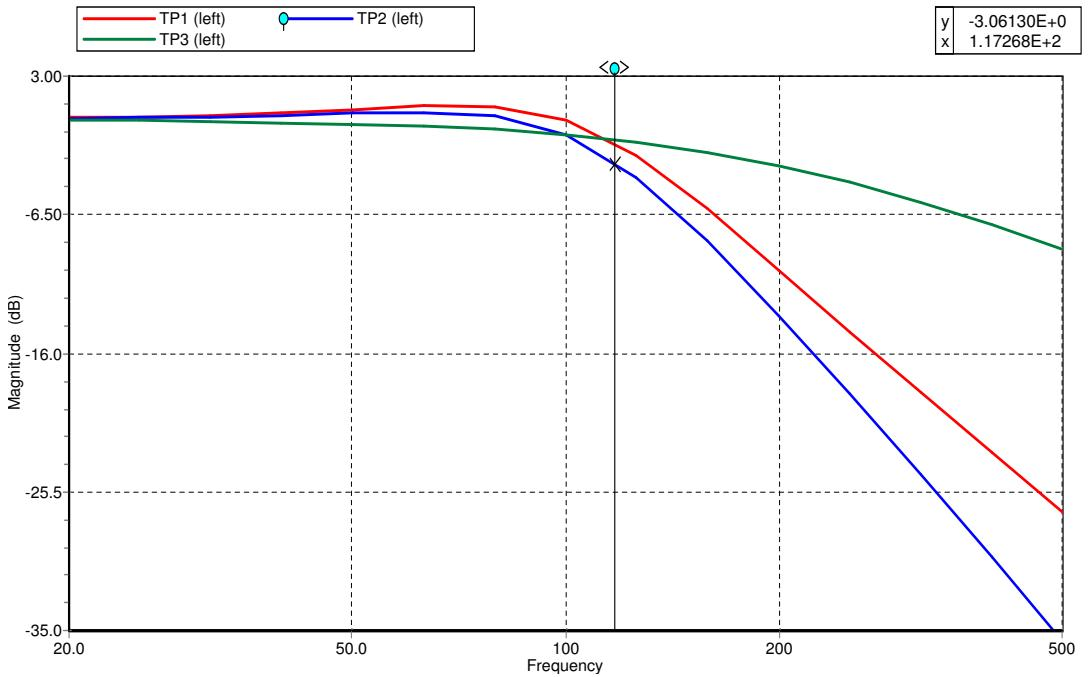
Figure 5.35: Simulated frequency response plot for input filters used on the throttle motor controller. The Green line shows the 1<sup>st</sup> order filter response, red the 2<sup>nd</sup> order, and blue shows the combined 3<sup>rd</sup> order response. The cursor marks the -3dB point for the combined filter stages.
