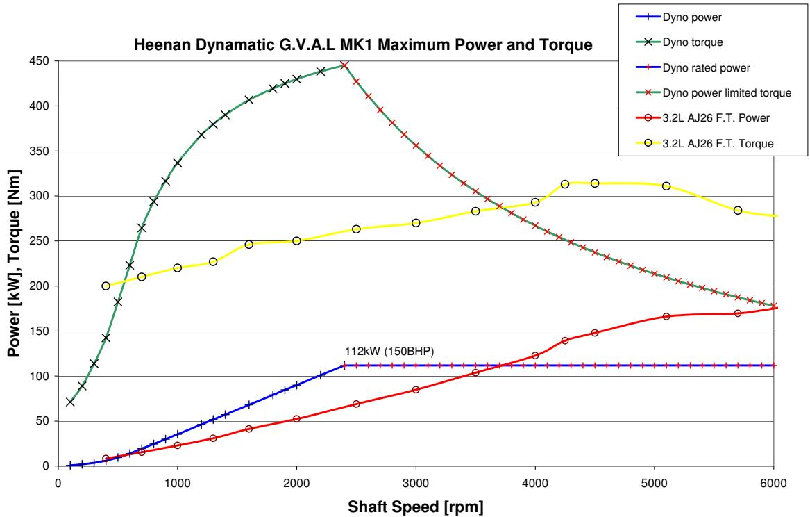
Figure 4.12: Dynamometer and AJ26 V8 engine maximum power and torque curves shown together for comparison
