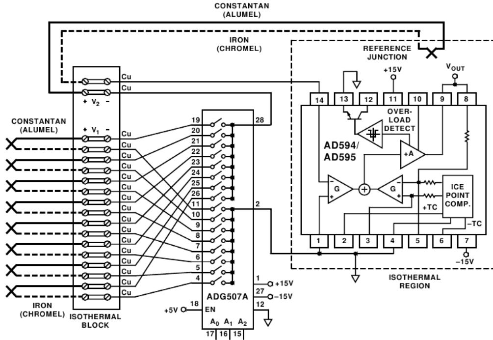
Figure 4.84: Thermocouple multiplexing circuit (Marcin, 1998)
