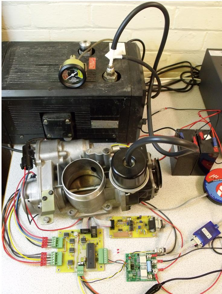
Figure 5.37: Photograph of the throttle unit test setup including the controller board, CAN interface, vacuum pump, and batteries
