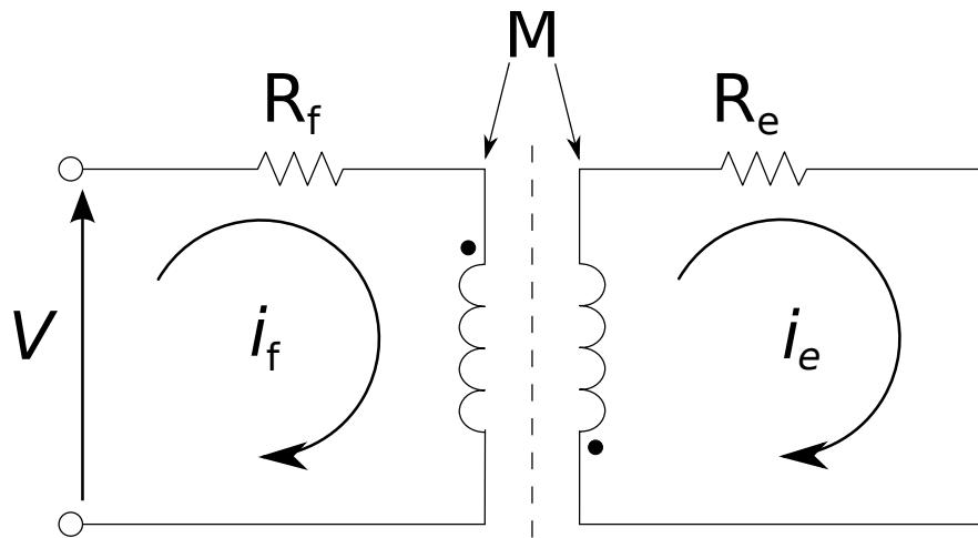
Figure 3.5: Field circuit and fictitious shorted damper winding circuit representing eddy-current path (Wright, 1972; Fegley, 1956)
