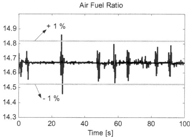
Figure 3.18: Results of direct inverse modelling approach to air/fuel ratio control (Arsie et al., 2004)
