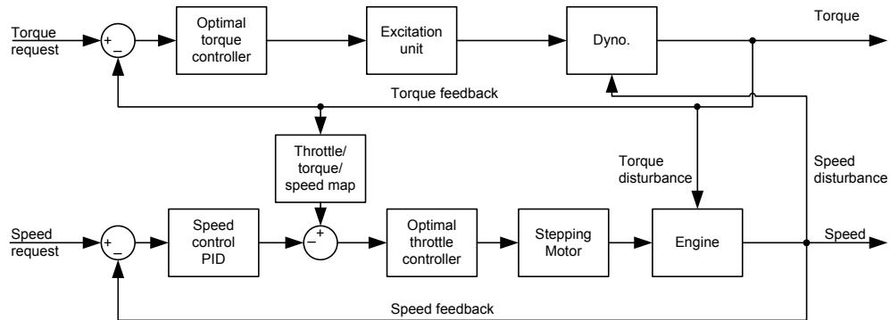
Figure 3.6: Block diagram of modes 1 and 3, no preview. (Koureas & Watson, 1984)
