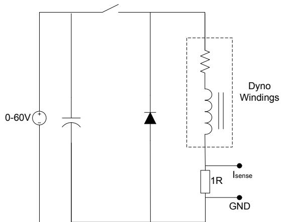
Figure 4.38: Test circuit modified to capture the turn-off response
