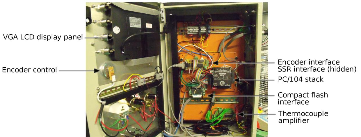
Figure 4.9: Inside the pendant operator's box
