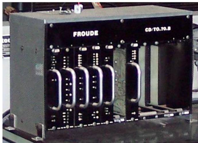
Figure 4.1: Froude dynamometer controller
