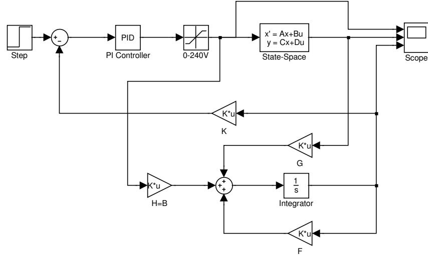
Figure 4.50: State-space model with full order estimator and state variable feedback control
