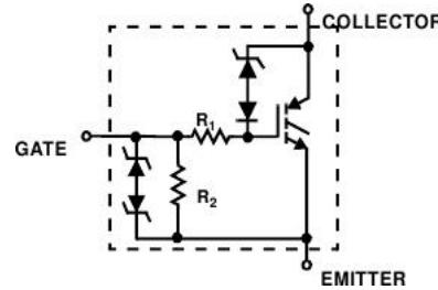
Figure 5.17: N-Channel ignition IGBT (Fairchild-Semiconductor, 2005)
