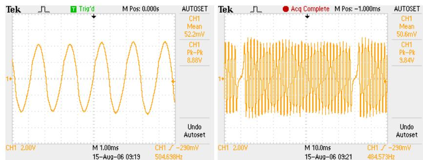
Figure 5.20: Engine speed sensor outputs captured using an oscilloscope
