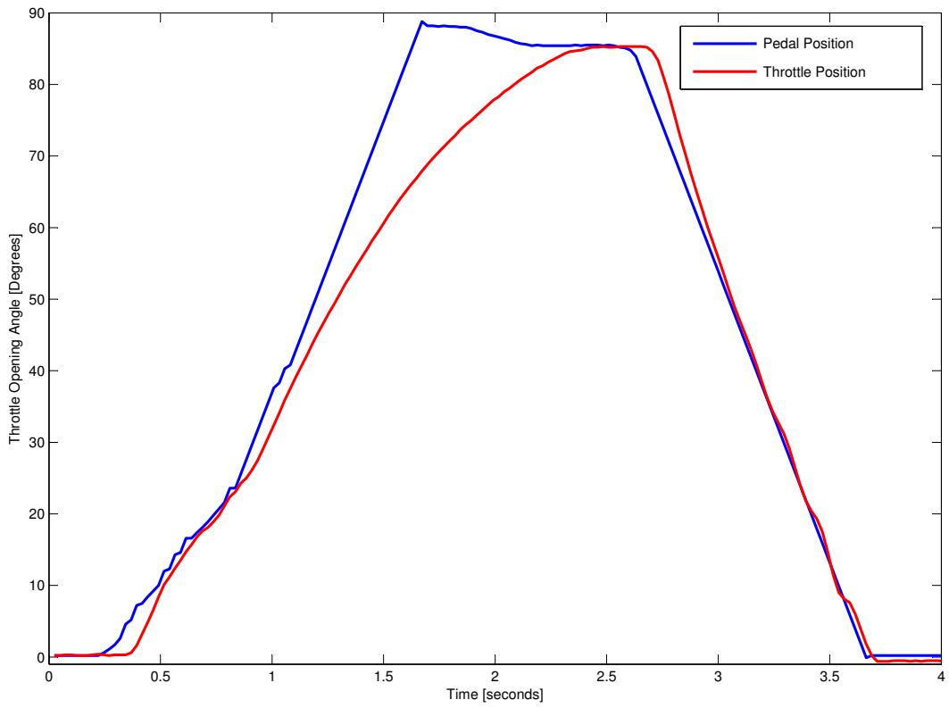
Figure 5.40: Throttle tracking of accelerator pedal lever demand position
