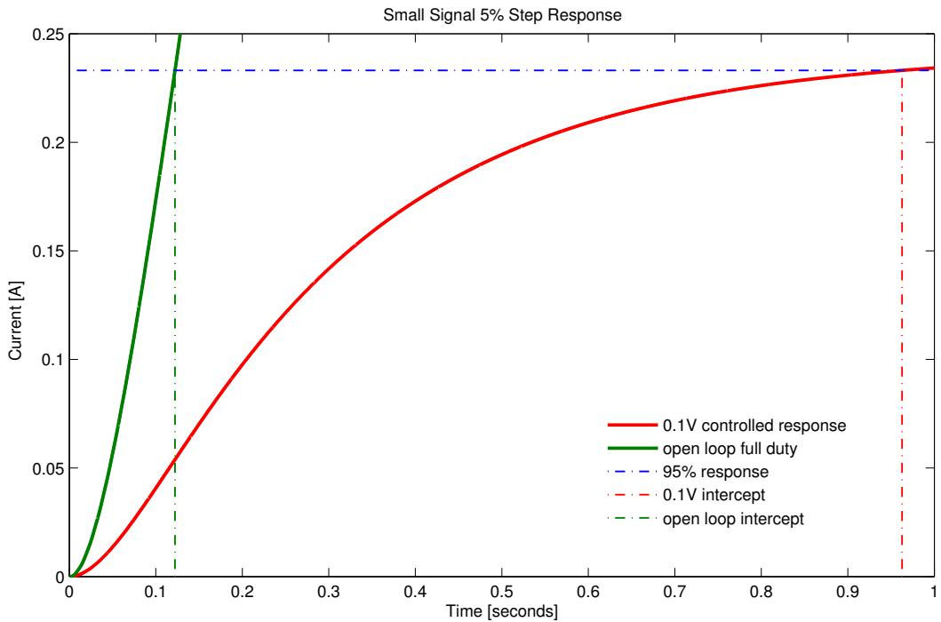
Figure 4.27: Comparison of open loop rise time with a small signal response
