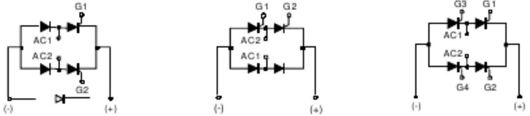
Figure 4.17: P series SCR configurations
