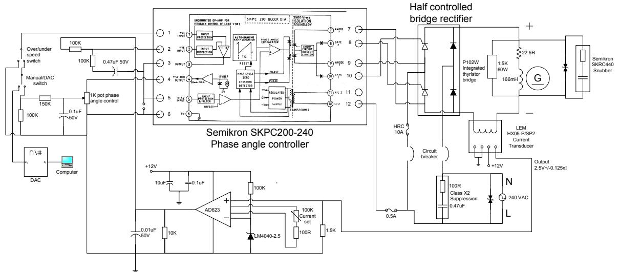
Figure 4.19: Current controller schematic
