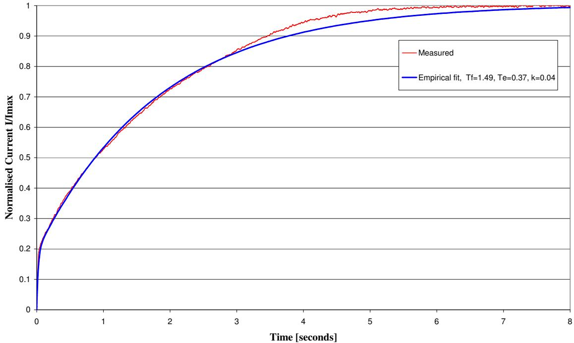
Figure 4.48: Modelled and measured normalised current responses to a 60 V applied voltage
