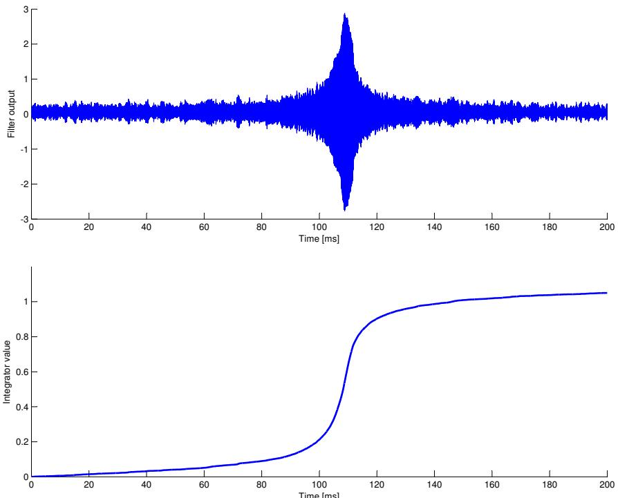
Figure 5.29: Plot of filtered chirp signal and model detection output
