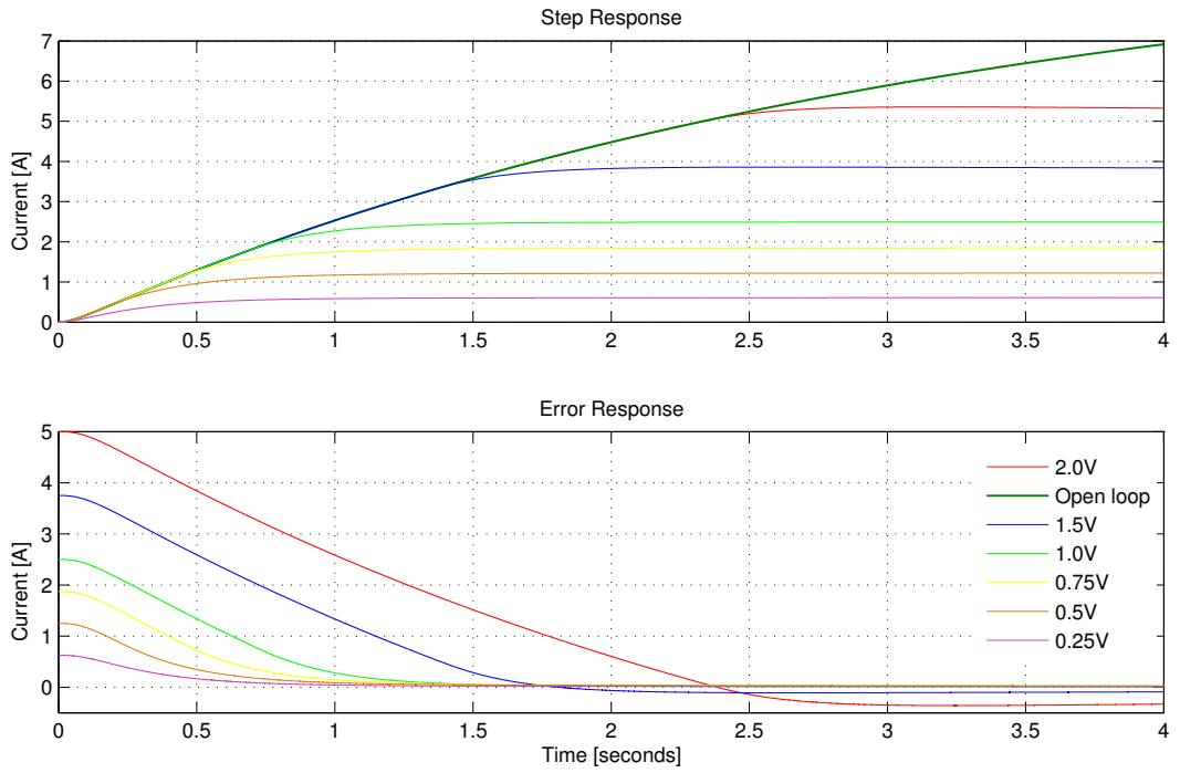
Figure 4.26: Plot of step response to various control set points and corresponding error response
