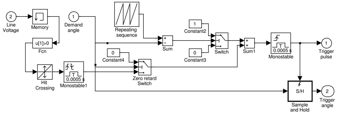
Figure 4.23: Phase detection and gate trigger pulse generation subsystem
