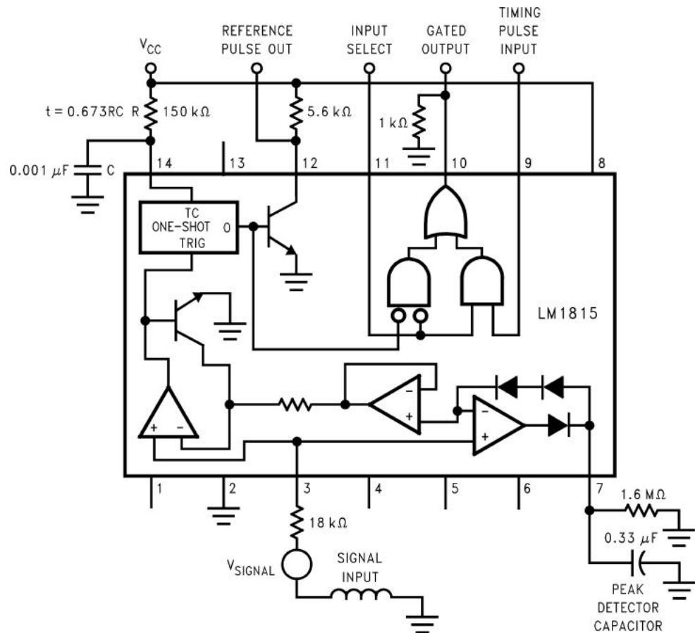
Figure 5.22: Adaptive sense amplifier typical application circuit (National-Semiconductor, 2005)
