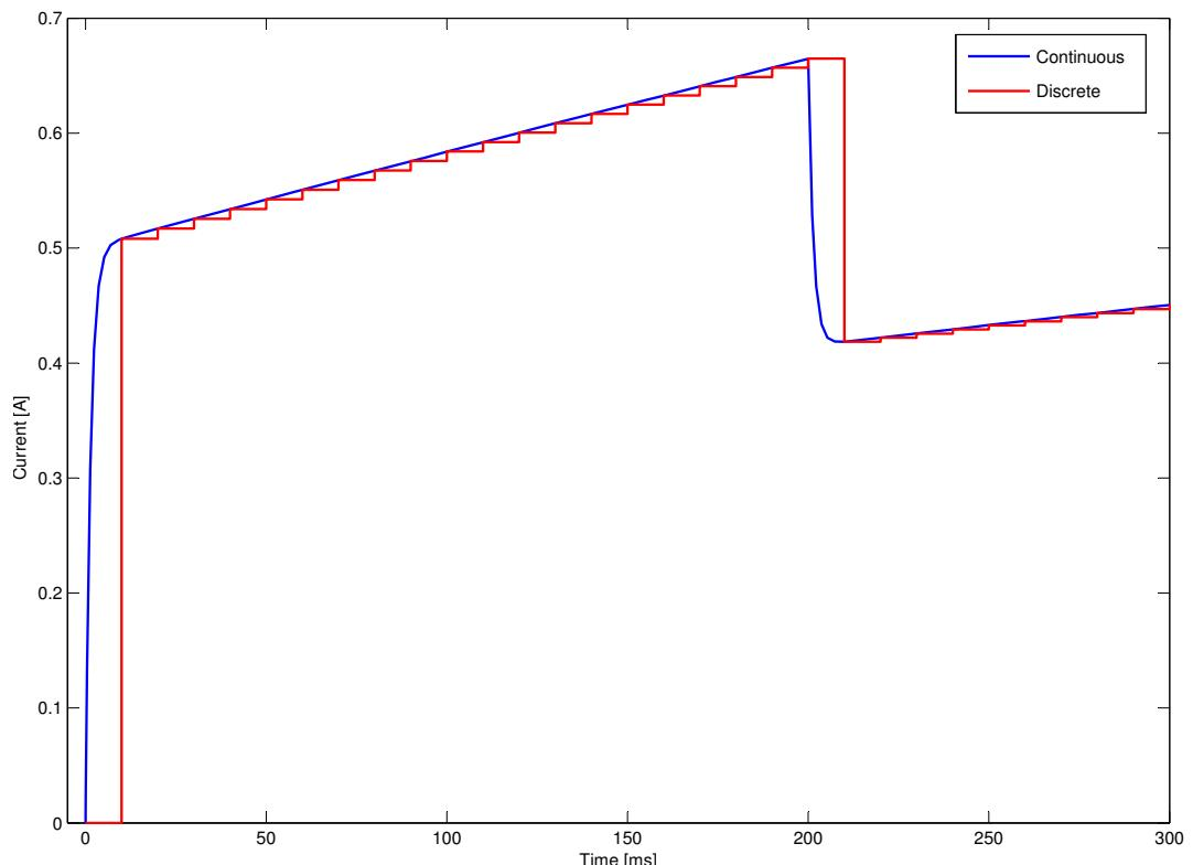
Figure 4.53: Plot showing the correspondence between continuous and discrete models
