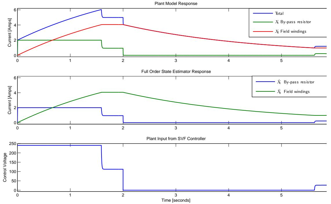
Figure 4.51: Time response plots of the estimated system to step inputs of 4 A and 1 A, at  $t=2$  and  $t=4$  seconds respectively
