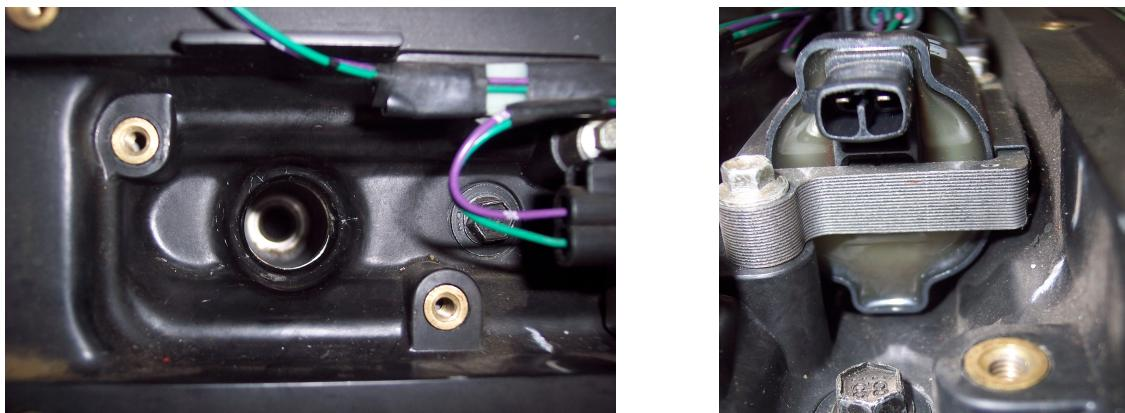
Figure 4.81: Photographs of spark plug bore and coil channel
