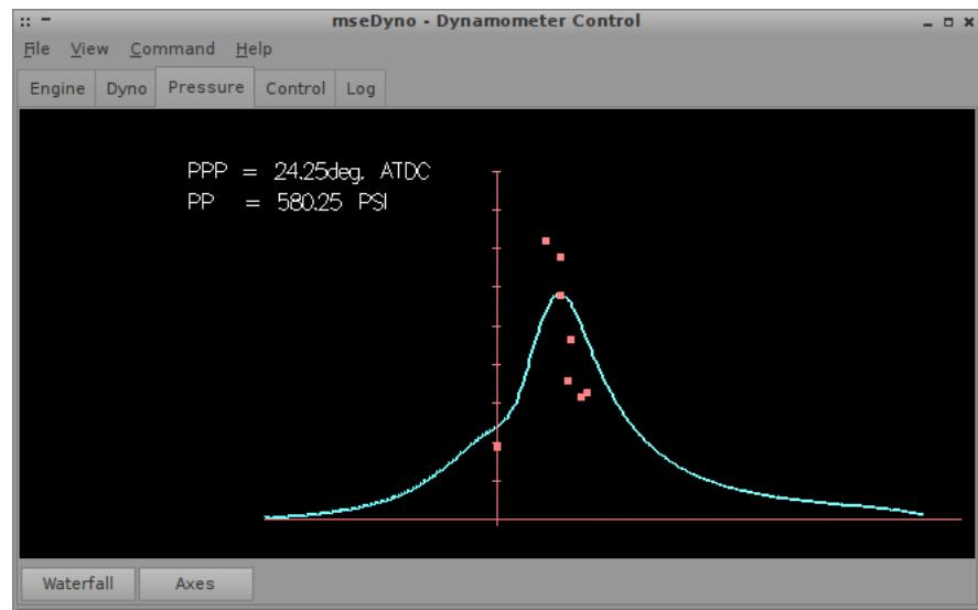
Figure 4.86: The mseDyno front end GUI showing the pressure plotter panel
