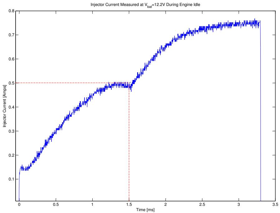
Figure 5.13: Fuel injector current response showing a *knee* point as the solenoid opens
