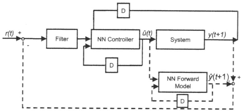
Figure 2.12: Internal Model Control structure
