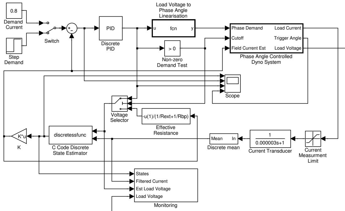
Figure 4.57: Block diagram of the full dynamometer system model with modifications for discrete controller and state estimator
