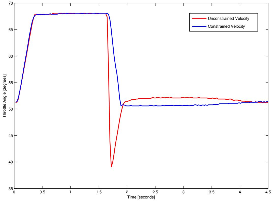
Figure 5.39: Throttle controller transients in response to CAN demanded step changes
