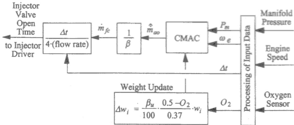
Figure 3.15: Block diagram of a the CMAC fuel injection controller (Shiraishi et al., 1995)
