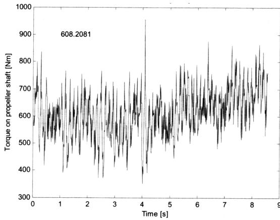
Figure 3.22: Propeller shaft torque (vehicle travelling at 81 km/h sampled at 100 Hz) (Sandberg, 2001)
