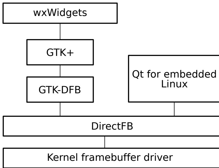
Figure B.4: wxWidgets on top of a DirectFB stack
