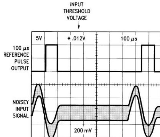
Figure 5.23: LM1815 output triggered from a low amplitude input signal
