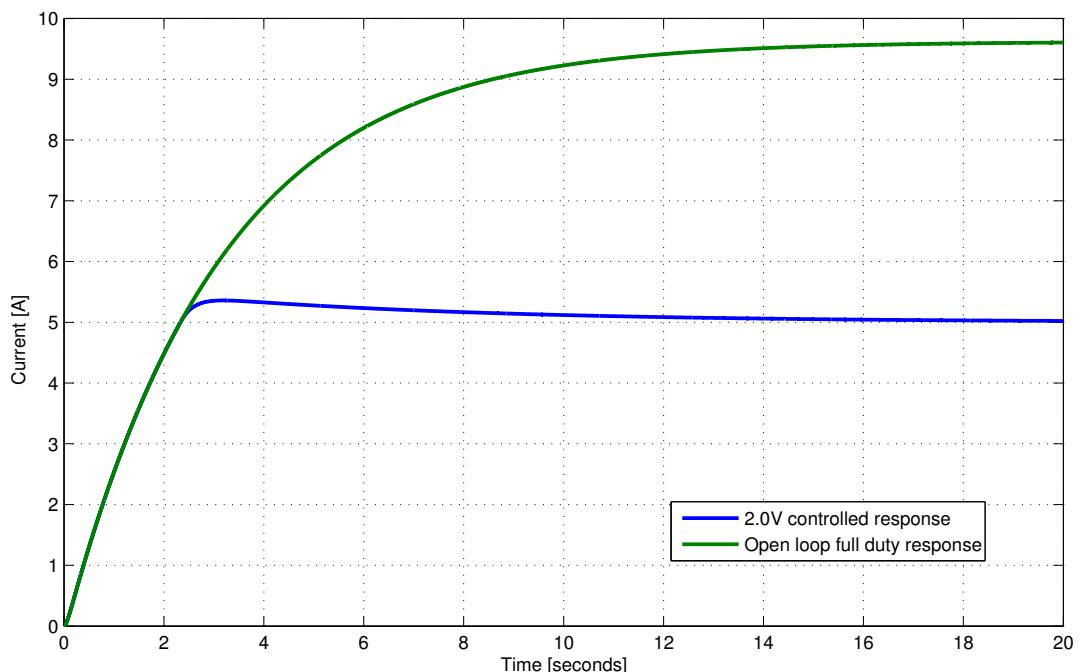
Figure 4.25: Plot of maximum demand controlled response and open loop full duty response
