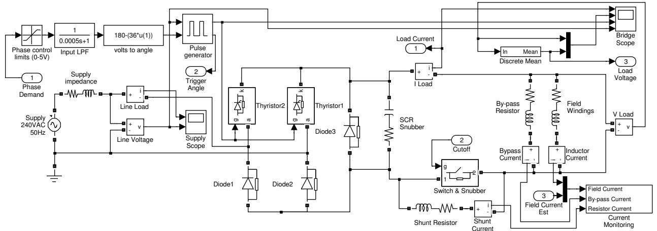
Figure 4.59: Dynamometer and phase angle controller subsystem block diagram with shunt resistor modification
