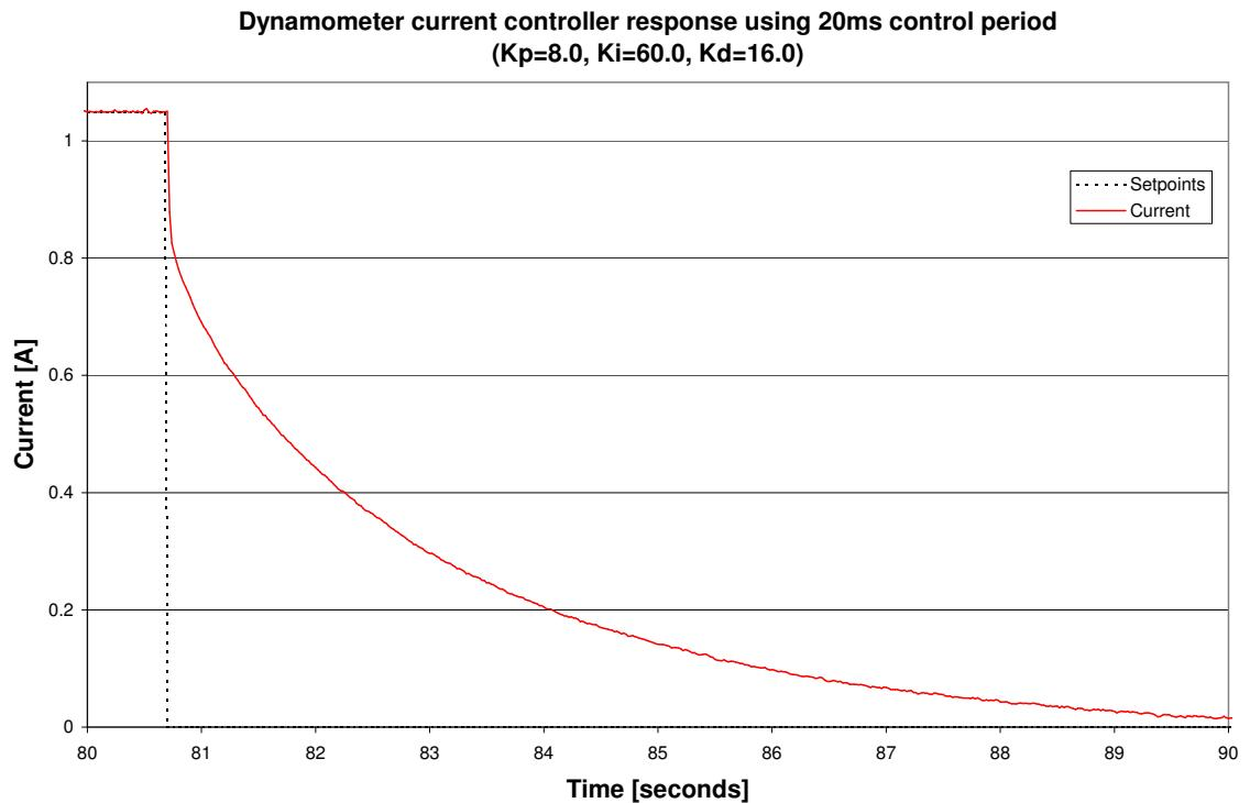
Figure 4.71: Response to step change to zero demand current
