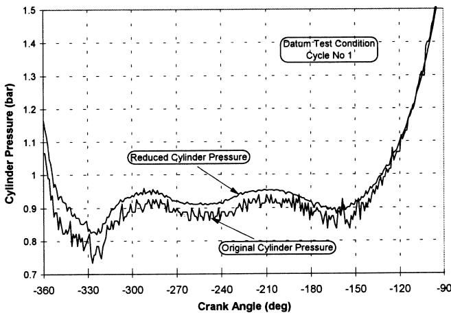
Figure 3.12: Comparison of reduced cylinder pressure and original data (Brunt et al., 2000)
