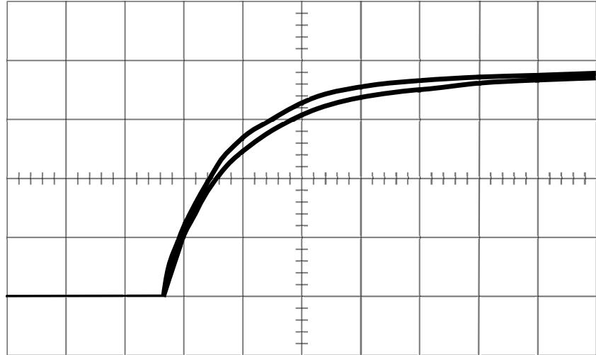
Figure 3.4: Eddy current coupling current (upper trace) and flux (lower trace) response at 100 rpm, 10 Hz pole frequency (Wright, 1972). 20 ms timebase, arbitrary vertical scale
