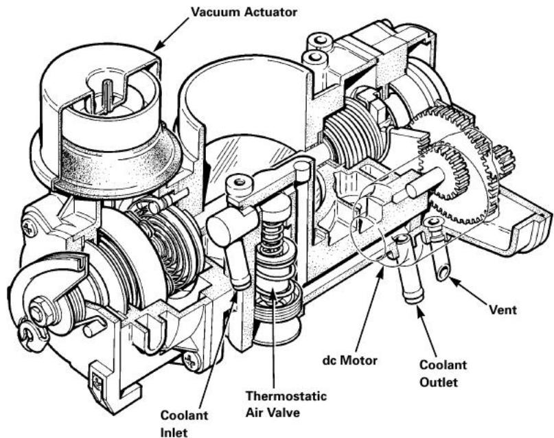
Figure 5.30: Electronic throttle unit cross-section (Jaguar, 1996)
