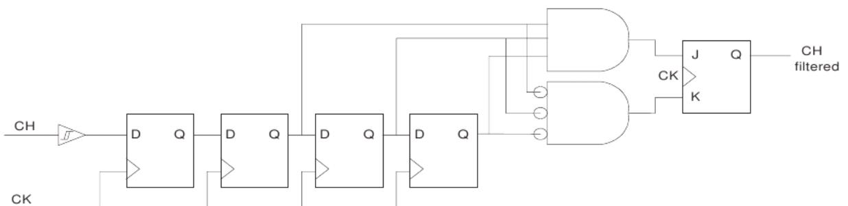
Figure 4.79: HCTL digital channel filter (csewards, 2004)
