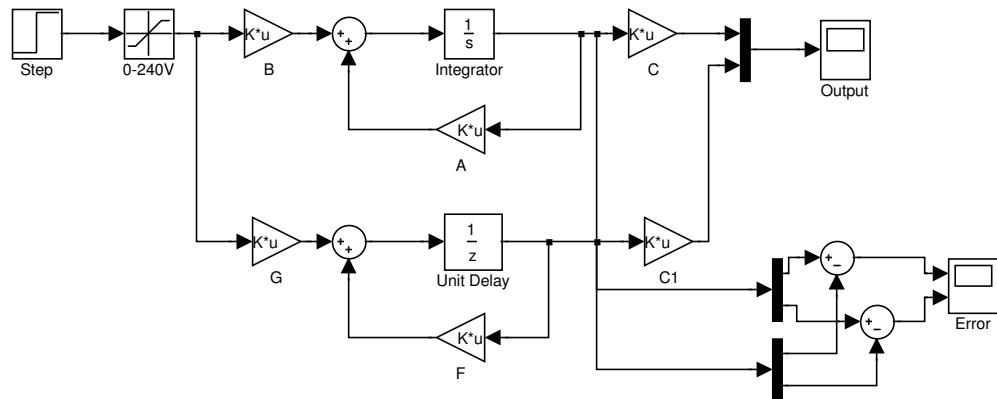
Figure 4.52: Continuous and discrete models for comparison
