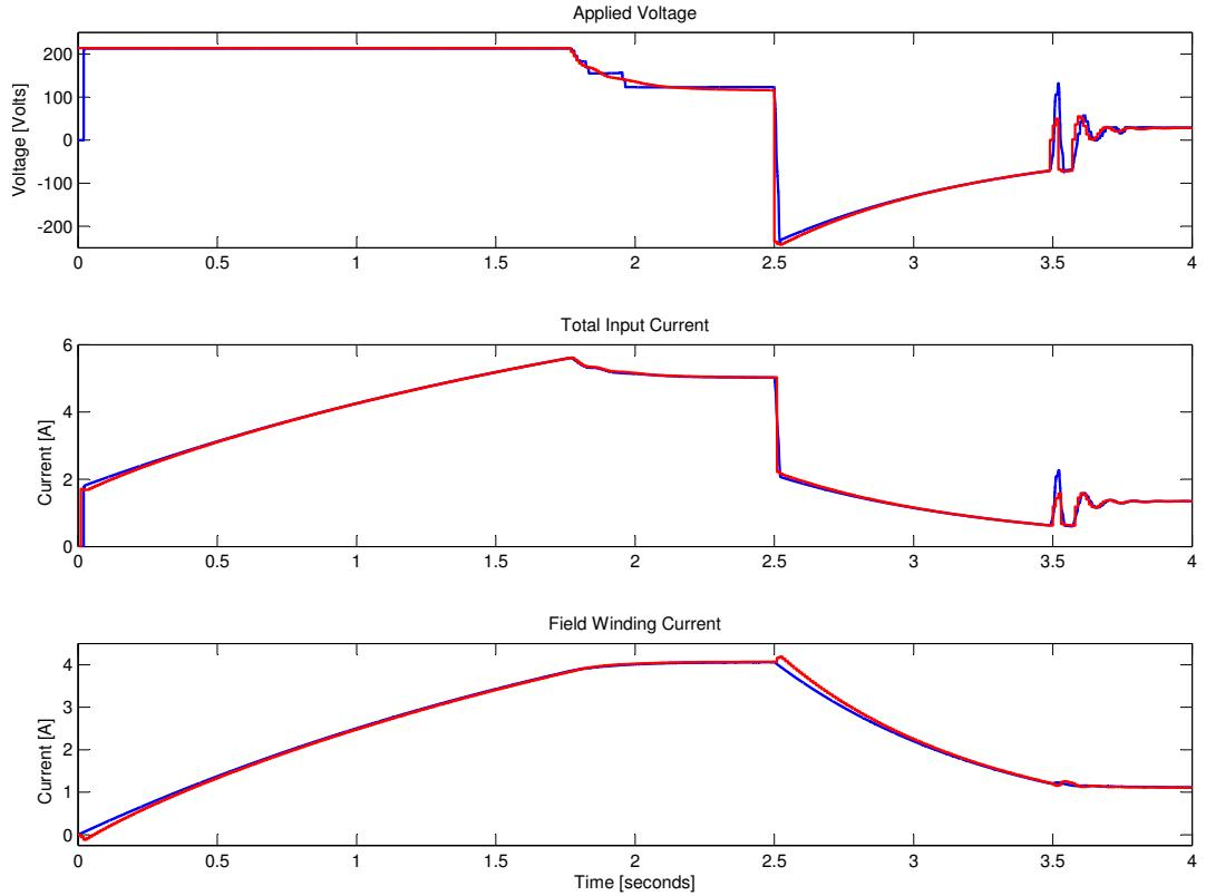
Figure 4.61: Plot of full model and estimator response to control set-point step changes for comparison. (blue represents the model output and red the estimator)
