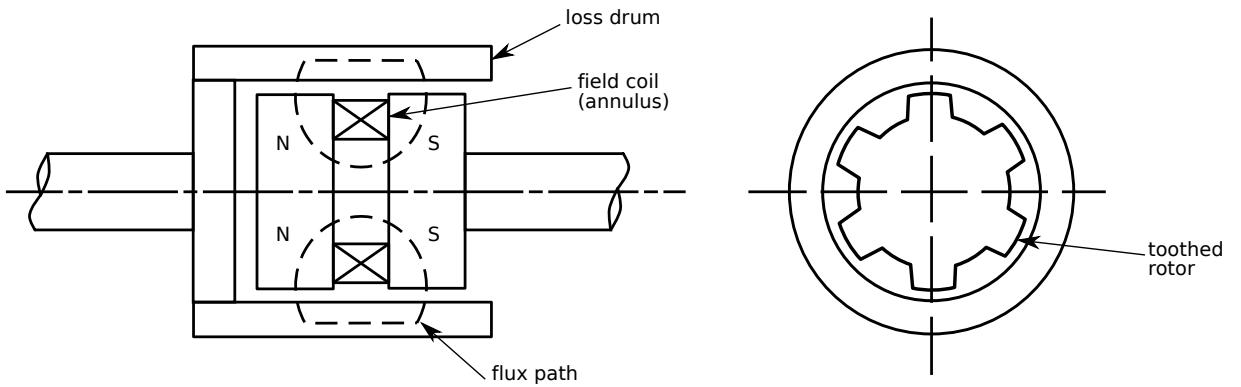
Figure 3.1: Schematic of an eddy-current coupling (Davies, 1966)
