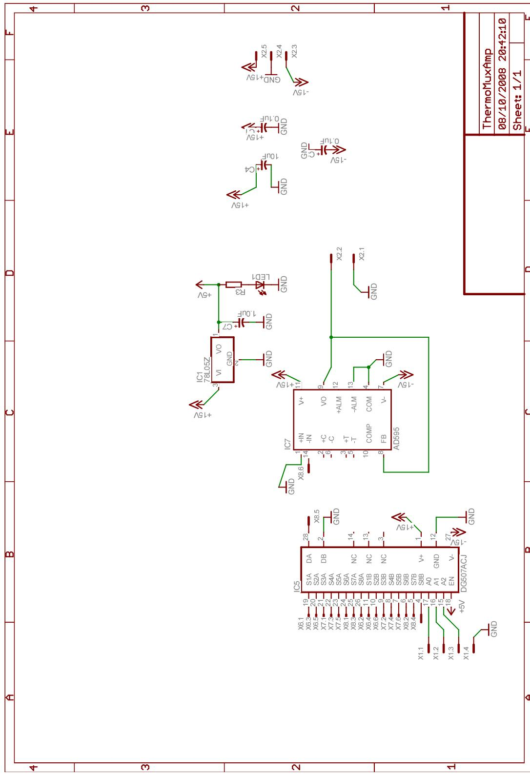
Figure A.5: Thermocouple amplification board schematic
