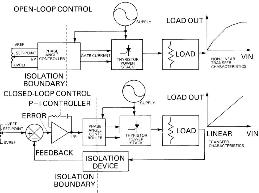
Figure 4.14: Comparison of open and closed loop current control modes
