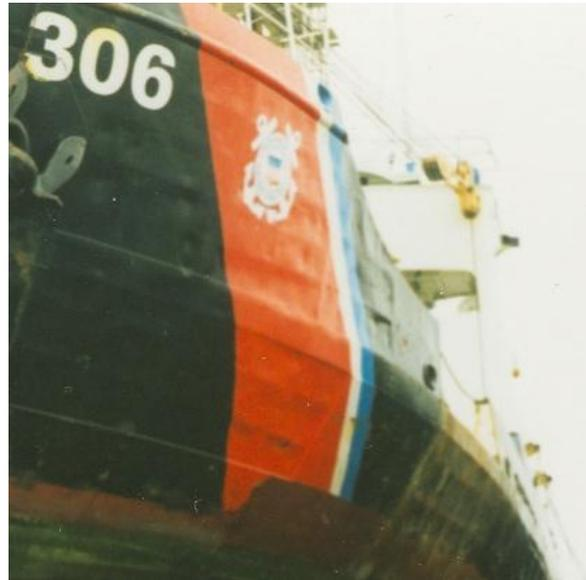
**Figure 29 – USCGC Buttonwood in dry-dock. Evidence of hungry horse imperfections in the side shell plating.**
