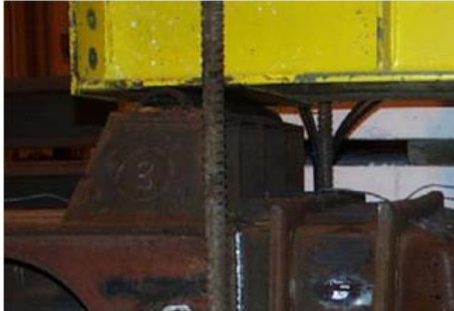
**Figure 146 – Load points for four point bending [121]**
