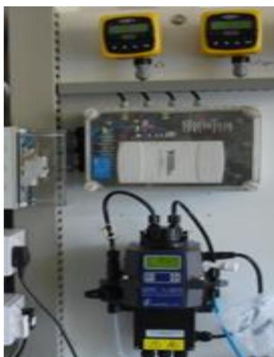
Figure 4-9: DAQ card wired up to the sensors
