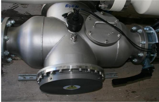
**Figure 4-6: UV reactor for the large scale setup**
