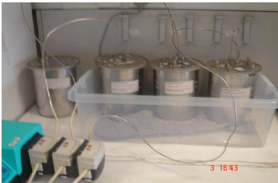
Figure 4.1 Laboratory mini-lysimeters system, control, PP, E10 and B20 fuel mixtures respectively.
