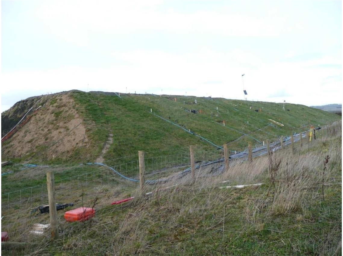
Figure 3.3 The BIONICS test embankment viewed from an approximately easterly direction. Various markers on the slope indicate the location of embedded instruments used in other studies. Blue piping, used for a sprinkler system, mark the approximate edges of the earthwork test plots.
