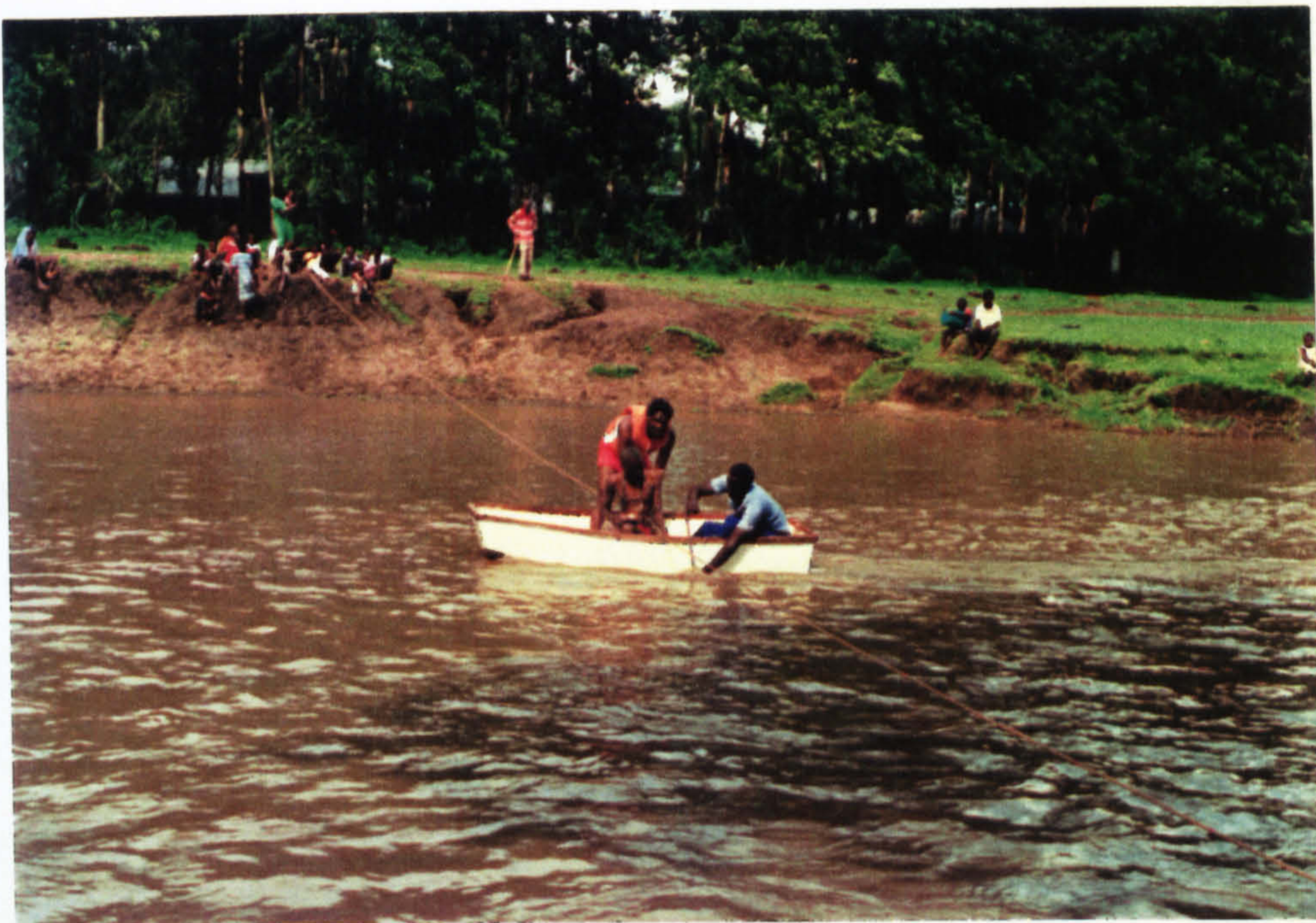
Fig 3.10a Discharge measurement on the River Nyando, on the upstream of the Ahero bridge.
