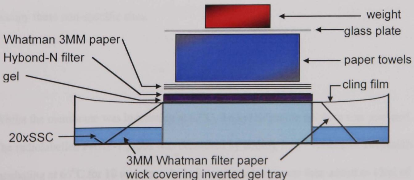
Figure 2.1 A diagram showing the apparatus required for Southern blotting
