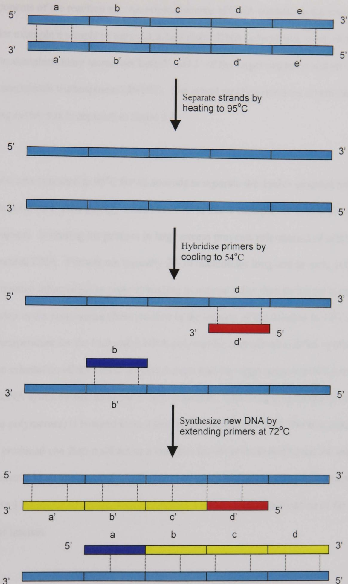
**Figure 2.3** Diagram summarising the polymerase chain reaction
