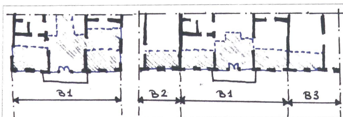
Figure 7.7. Daylight penetration in rooms of attached and detached buildings (referring to a rule of thumb: daylight penetrates about 2.5x the aperture height. Robbins, 1986).
