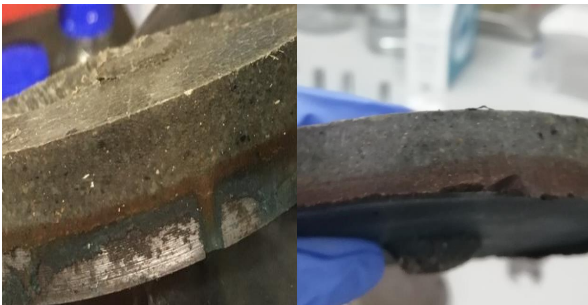
Figure 7.1: Steel and clay recovered from test cells. Layers of green and orange corrosion were observed in inoculated experiment with steel (left), whereas no green layer was observed in the sterile experiment (right).
