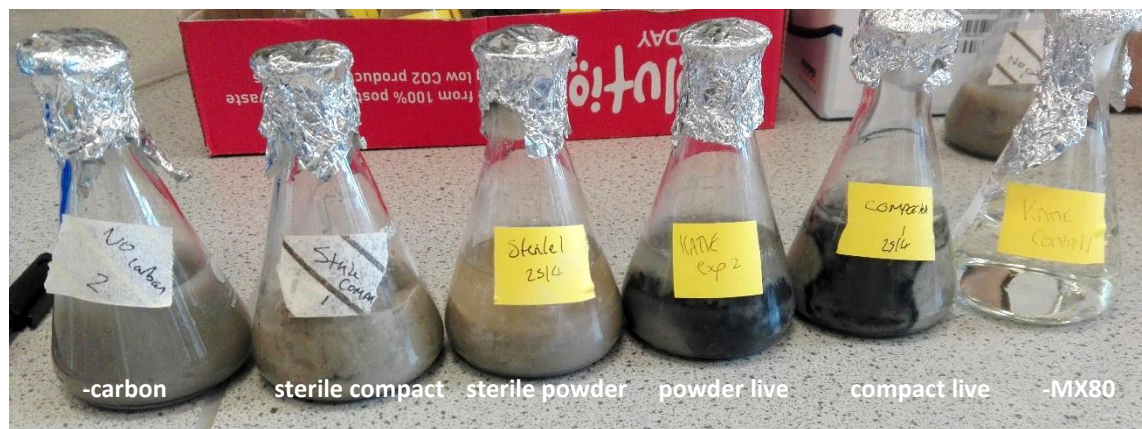
Figure 4.4: Aerobic enrichments of MX80 bentonite on day 18. The no carbon control shows no precipitates and is uniformly grey. The sterile controls have a small concentration of black precipitate present in small particles. The live experiments have an obvious colour change from grey to black in localised anaerobic areas. The no MX80 control (-MX80) is colourless.
