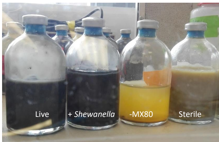
Figure 4.1: Compact MX80 iron-reducing enrichments on day 21, obvious colour differences were seen between each flask. The biotic flasks were black, indicating iron reduction and the precipitation of reduced iron minerals. The control flask which contained no MX80 remained orange (the colour of PCFeO), and the sterilised flasks remained orange / grey.
