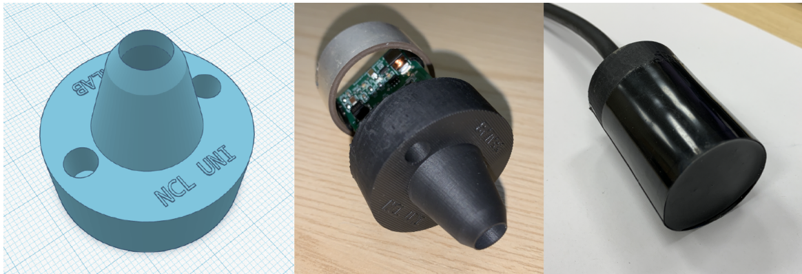
Fig. 5.15 This figure shows the design and construction of a 3D printer encapsulation component. This shows progress made to enable mass production of the potted vessel detector/communication device. Key design aspects in the 3D printed design include; cable gland, mounting holes, PCB holder and transducer end potting process.
