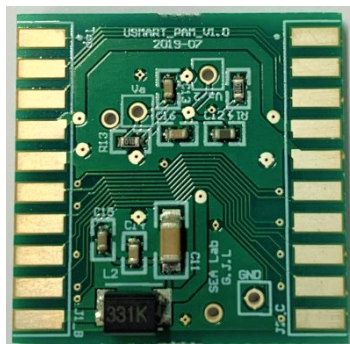
(a) PCB Top - Power Supply
