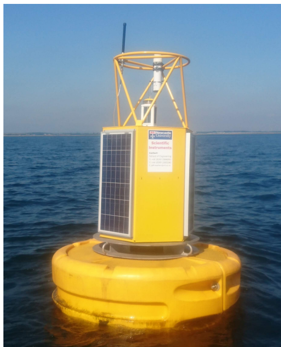
Fig. 5.7 Newcastle University WiFi Gateway Data Buoy.
