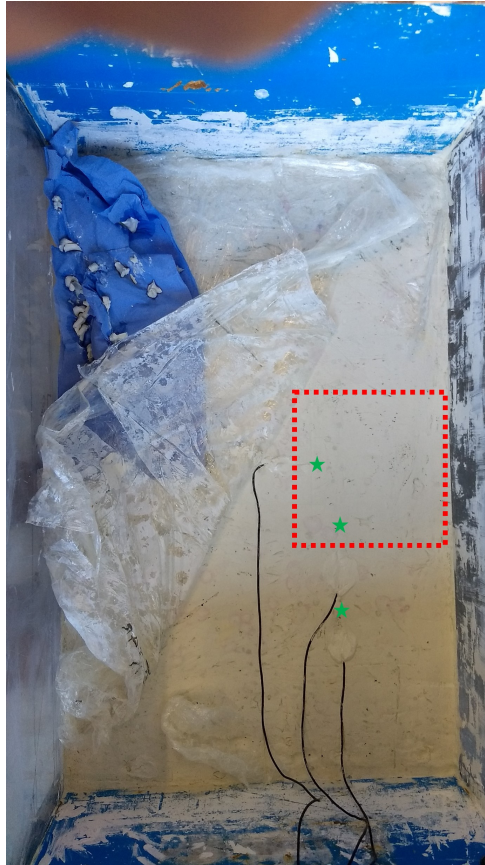
Figure 4.10: Placement of the PPTs in the soil, Red line to outline the position of the foundation, Green stars to note the position of the PPTs in the clay
