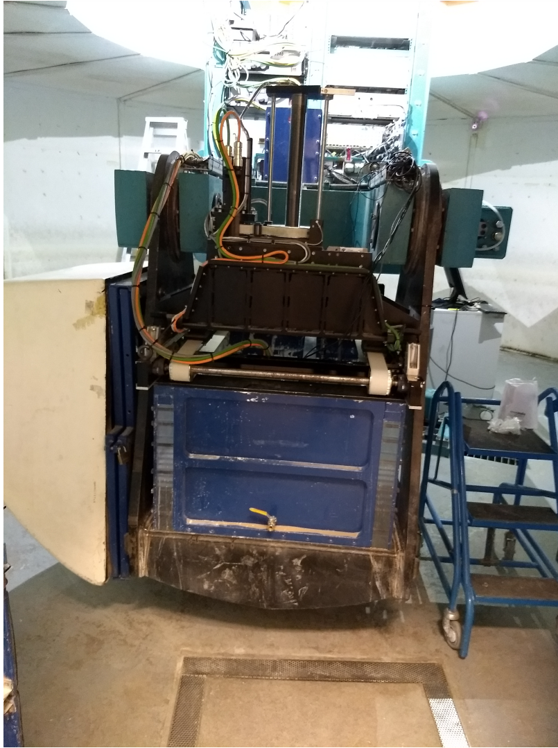
Figure 5.2: The centrifuge box and robot loaded into the centrifuge ready for the test to begin
