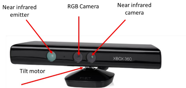
Figure 3-11 Structure of Kinect 3D scanner
