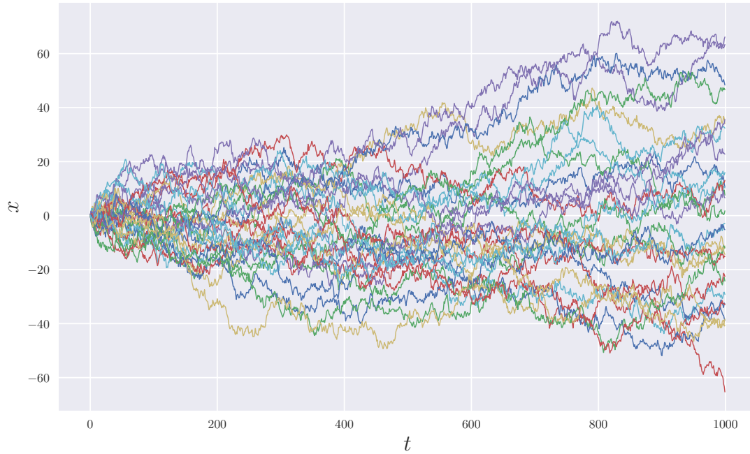
Figure 3.3 30 samples of a simple random walk as specified by (3.3).
