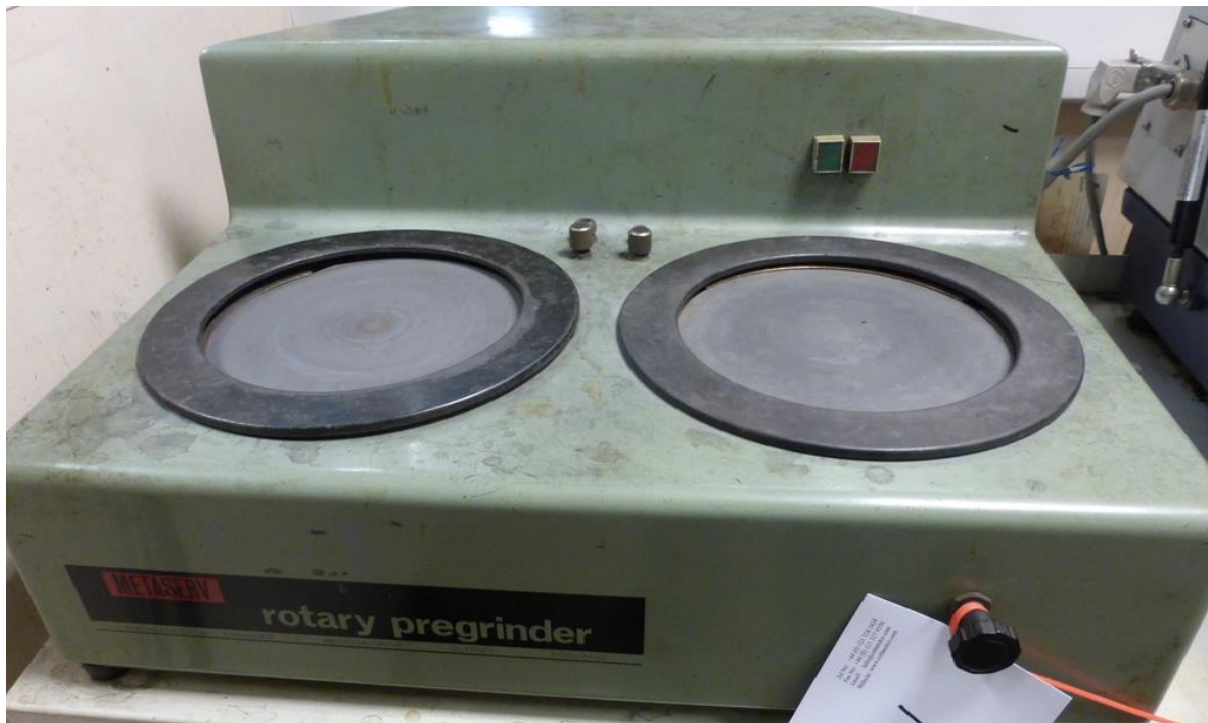
Figure 3-4 Rotary pregrinder (Buehler UK, Coventry, UK) used for manually polishing the HMWPE discs.
