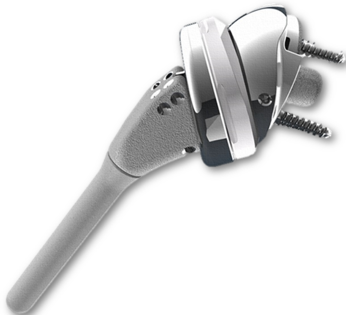
Figure 2.22 Reverse total shoulder joint replacement. To the upper right is the CoCr glenosphere component with its titanium baseplate. To the left is the humeral component, with the UHMWPE humeral component atop a hydroxyapatite ceramic coated stem. Adapted from JRI VAIOS®
