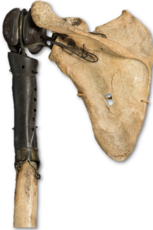
Figure 2.18 Péan’s first artificial shoulder joint, which consisted of a platinum stem, a rubber ball coated with paraffin, and two metal loops which attached the ball to the scapula and stem. Adapted from National Museum of Health and Medicine (NMHM)
