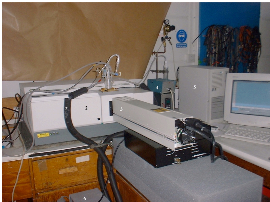
Figure 2. 22 (1) The in-situ electrochemical FTIR cell; (2) BioRad FTS 6000 Spectrometer; [(3) 325nm Laser]; (4) Heated block controller; (5) Control PC; (6) Heating/ cooling unit; (7) Cooling/heating tubes to cell.
