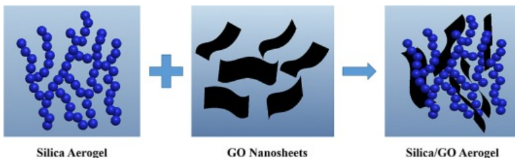
Figure 1. 15 Schematic illustration of the formation of composite aerogels (Lei et al., 2017).
