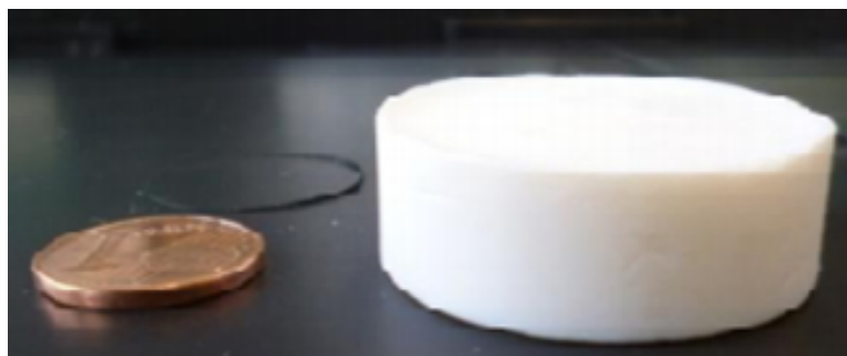
Figure 3. 1 Silica aerogels produced from water glass by using novel APD method (Han et al., 2018).
