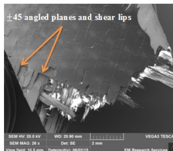
Figure 6-12. SEM micrograph revealing the top surface view of a sample with -45°/+45° fibre configuration indicating multiple angled fracture planes.
