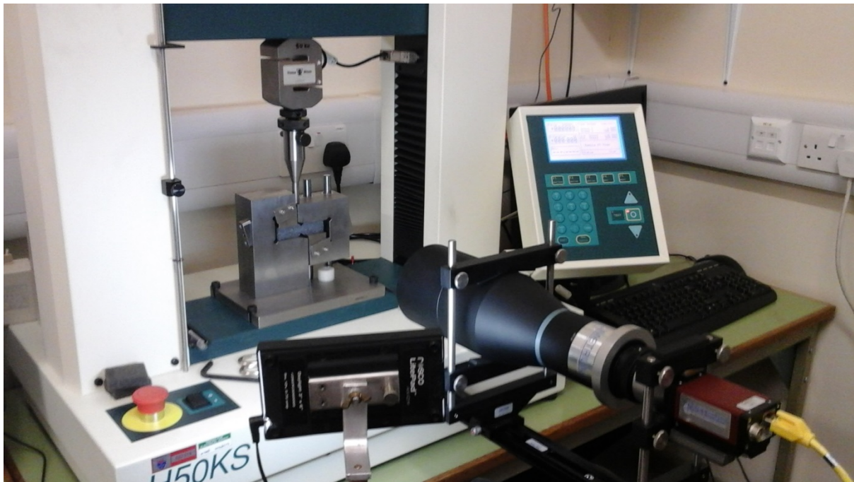
Figure 3-11. Experimental set up for Iosipescu shear testing coupled with DIC system.
