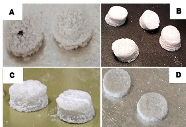
Fig.4. 11. Representative green parts, 3DP with the following powder blends: A. AW1.01, B. AW1.03 C. AW1.1 and D. Representative sample for AW1.2 AW2.1, AW2.2 and AW2.3.
