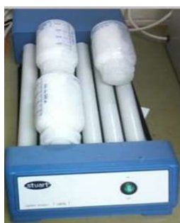
Fig.2. 6. Roller mixer used for mixing MD and AW powders into a powder blend.
