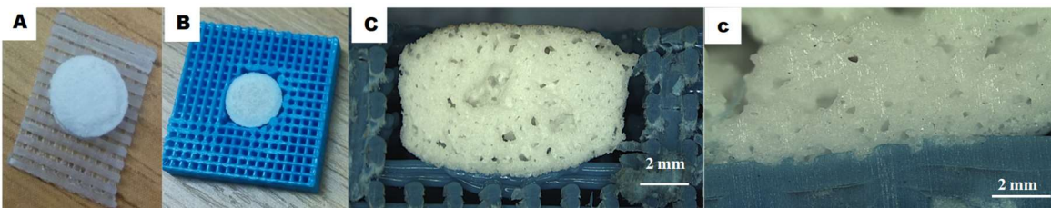
Fig.5. 9. Stereomicroscope images of ultrasonic welded porous PLA with AW (2.5 mm thick sample): A. Simple PLA squared geometry, B. PLA porous box with AW disc inserted and C and c. Cross section images of structure obtained in B (increasing magnification).
