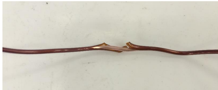
Figure 7.20 Damaged magnet wire after 49 day thermal aging at 175°C – not a pressed coil
