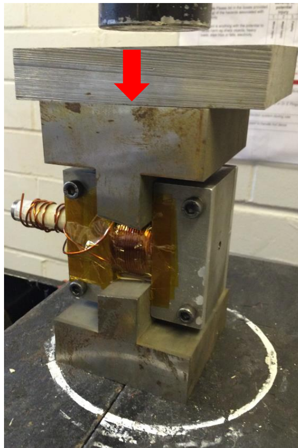
Figure 6.10 Compression of a coil under hydraulic press
