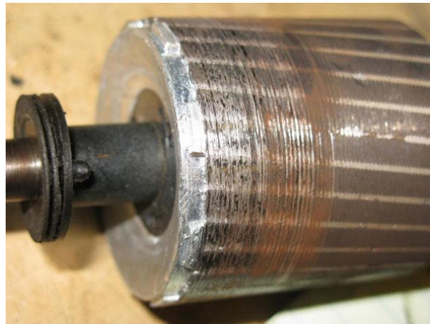
Figure 7.1 Rotor damage due to eccentricity
