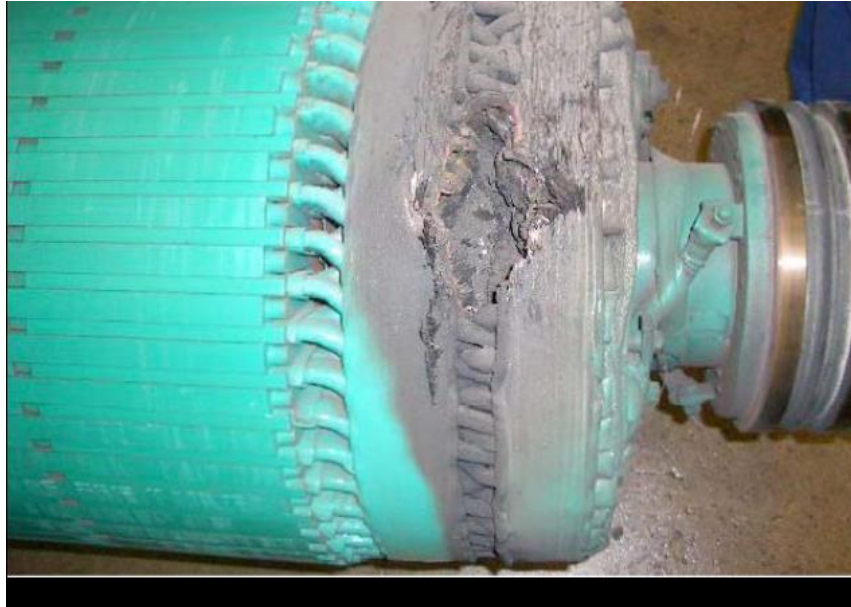
Figure 2.5 Turn to turn winding fault in an induction machine [47].
