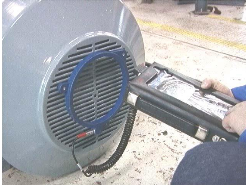
Figure 2.6 Search coil (Emerson M-343F-1204) [7]
