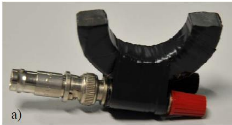
Figure 2.8 C shape magnet flux coil
