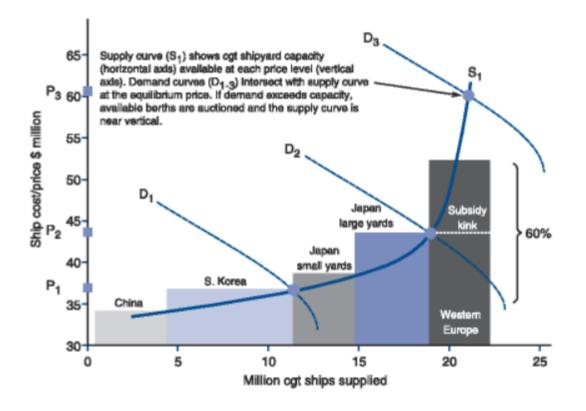
Figure 7.1 – Short run bulk shipbuilding demand and supply functions (Stopford, 2009, p. 633)
