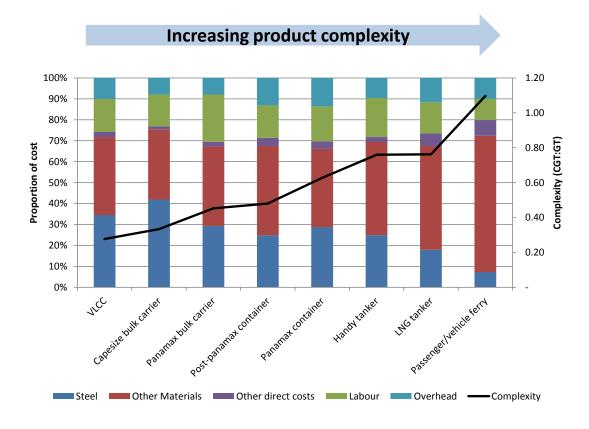
Figure 6.3– Variation in cost breakdown by ship type
