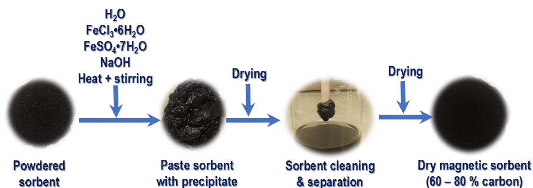
Figure 3.1: Production of magnetic sorbent
