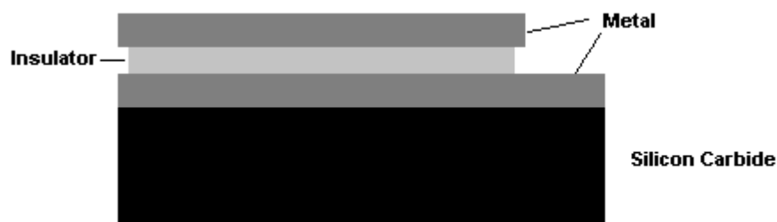
Figure 2.7 Schematic of a Metal-Insulator-Metal capacitor
