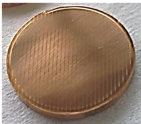
Figure 6.4 – Photo of 20 mm copper anode tool with photoresist linear pattern
