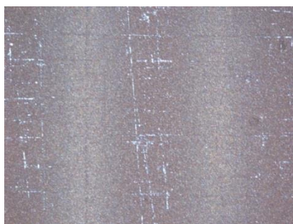
Figure 7.19 - Optical microscope image of deposition between linear features, located below area H, plated at 20 mA/cm 2 under PUS conditions at 40 W/L (Mag x5)
