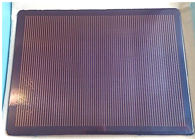
Figure 4.19 – Photo of A7 size dry resist tool with linear pattern features
