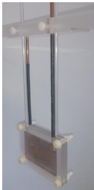
Figure 4.12 – Photo of the Enface electrode holder for A7 size substrates with support rods and support block
