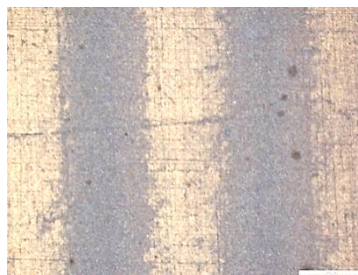
Figure 7.17 - Optical microscope image of linear features within location E, plated at 20 mA/cm 2 under DC conditions with CUS at a power of 40 W/L, (Mag x5)
