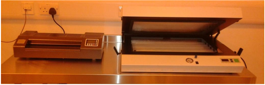
Figure 4.17 – Equipment used for dry photolithography with a lamination device (left) for applying the photoresist and a UV light box (right) for exposing the photoresist to ultraviolet light through a photomask
