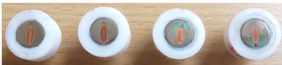
Figure 6.15 – Photo of deposit features plated in small-scale cell with 1 x 5 mm rectangular anode feature. (a) 75% i_{\text{Lim}} silent pulsed, (b) 75% i_{\text{Lim}} pulsed US, (c) 50% i_{\text{Lim}} pulsed US, (d) 50% i_{\text{Lim}} , silent pulsed.
