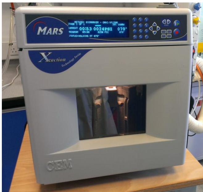
Figure 5.1: The MARS 5 microwave at Newcastle University used for extracting total lipids as part of the GDGT extraction procedure.
