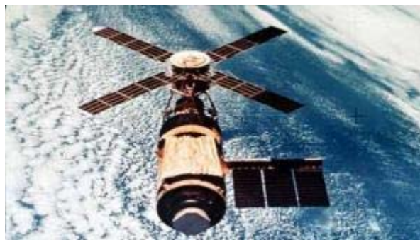
Figure 78 Skylab 4 space station (1973) generated over 20kW of electricity by PV panels (photo reproduced from [23]).
