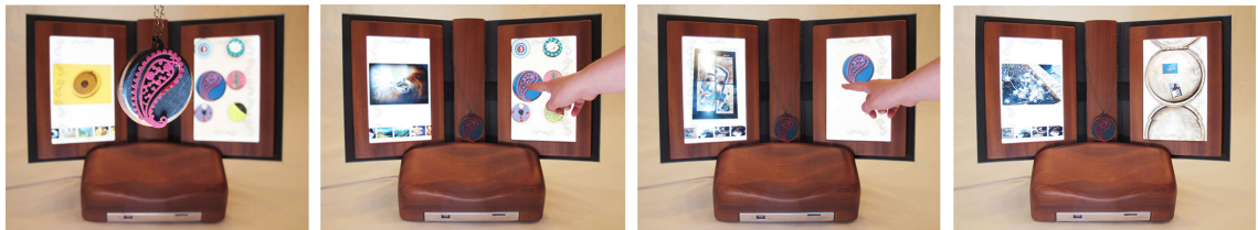
Figure 11: Connecting: A wireless accelerometer is embedded in a jewelry piece such as a necklace. When the necklace is within a 50 cm range of the book, the icon on the right screen enlarges. When pressed it opens to show the inside of a locket.
