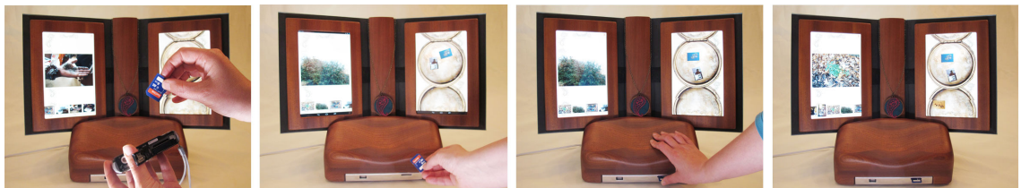
Figure 12: Uploading: When the locket is open an SD card or USB can be inserted into the base and images will appear at the bottom of the right hand screen.
