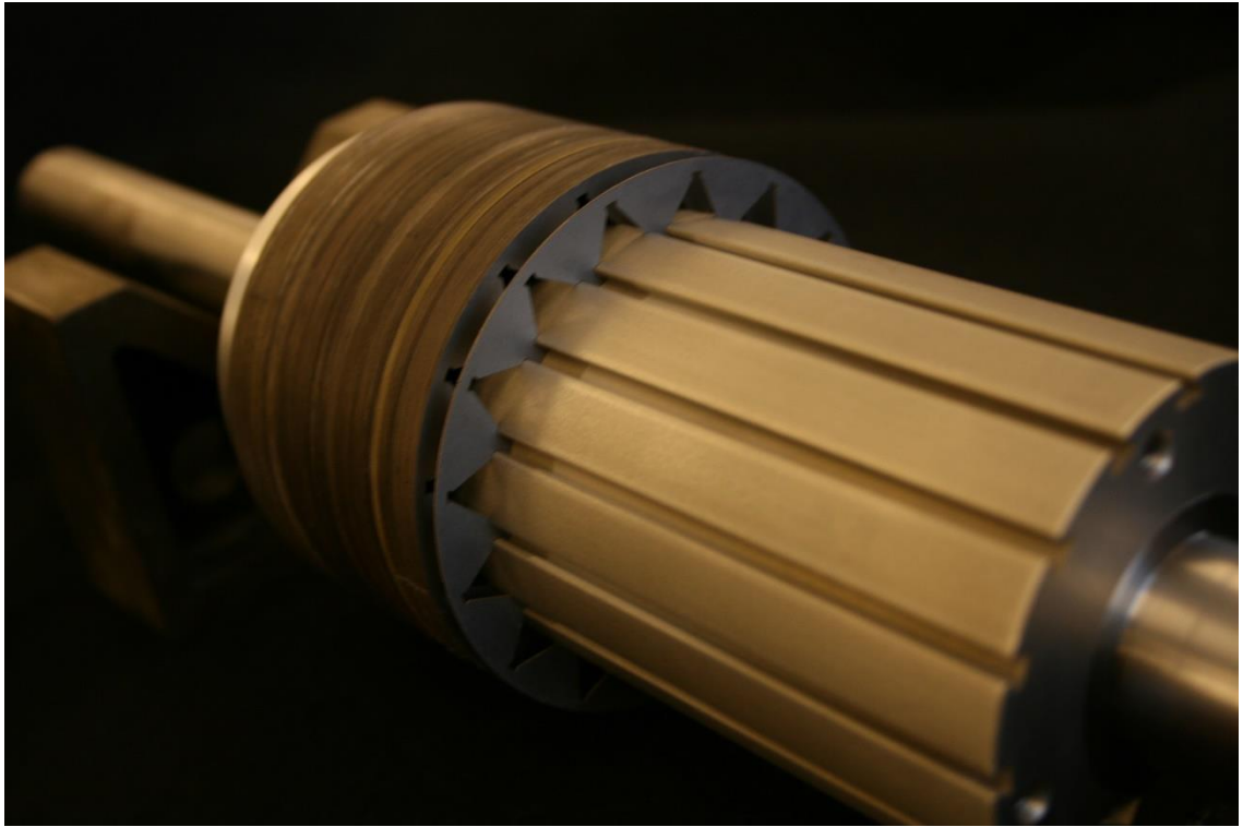
Figure 4-5: Showing construction of rotor with lamination rings being fitted to slotted, aluminium rotor support.
