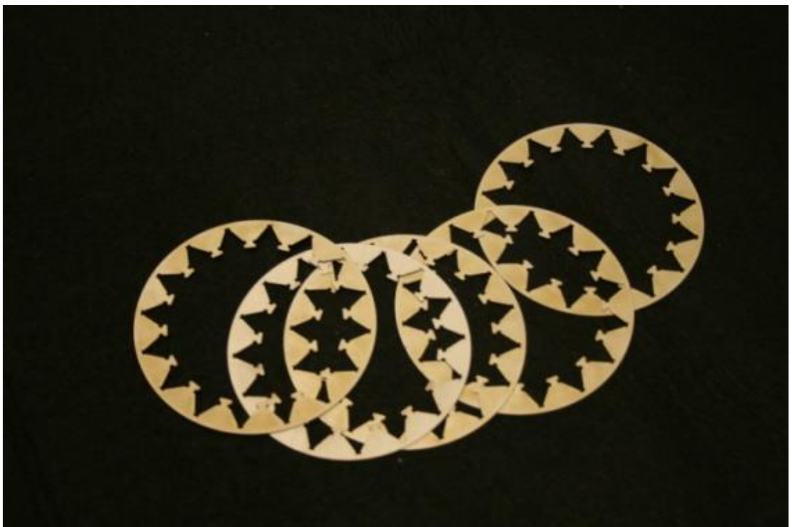
Figure 4-2: Rotor Laminations were cut as a continuous ring in order to simplify prototype construction.
