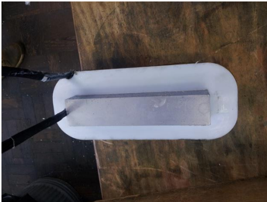
Figure 9-8: Showing the top insert, used to protect the coil from extrusion between the punch and the bobbin / die.
