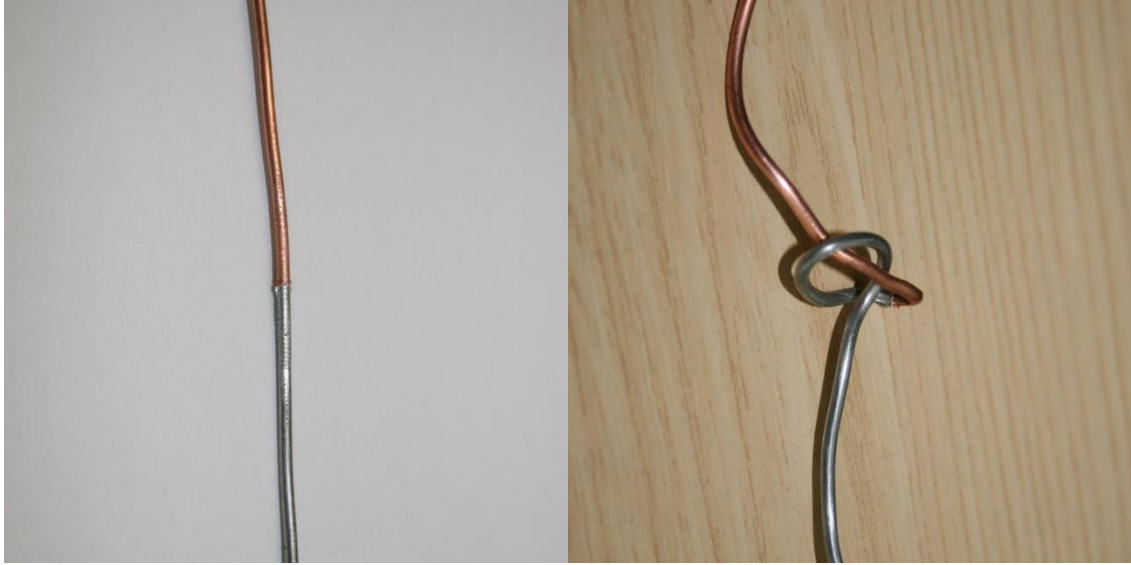
Figure 6-6: Showing (left) cold pressure welded joint between 1.4mm copper and 1.4mm aluminium enamelled wires. (Right) demonstrates the mechanical integrity of the joint.
