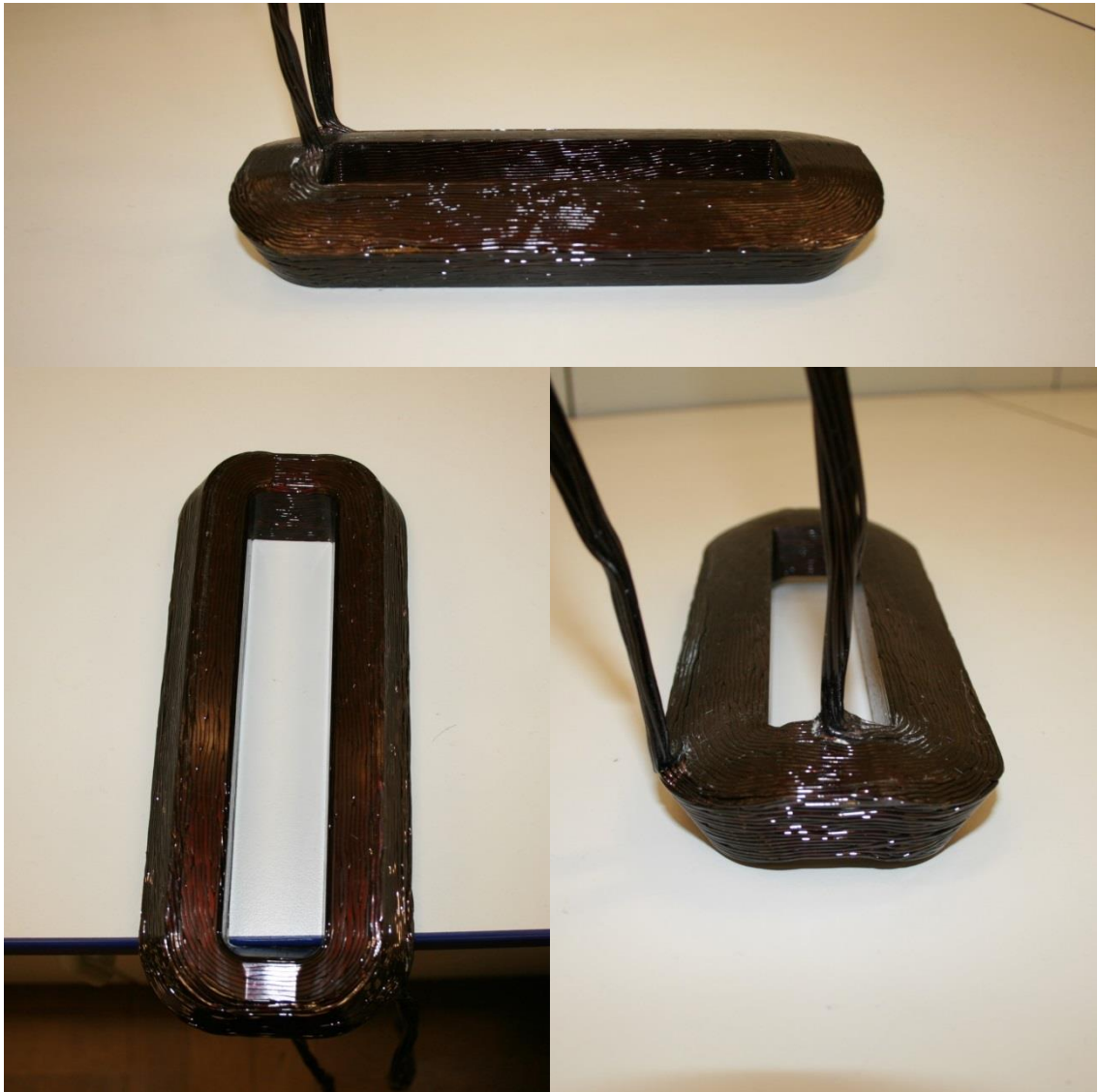
Figure 9-12: Showing final compressed coil details.
