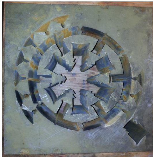
Figure 9-2: M270-35A bonded lamination stack showing how all motor lamination steel could be cut from a single 300mm by 300mm block.
