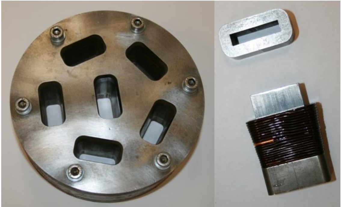
Figure 6-2: Compressed winding die (left) suitable for compaction of 6 coils simultaneously. Compressed coil fitted to bobbin, pictured with punch above (right).
