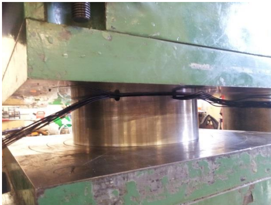
Figure 9-10: Punch pressed flat into die under 400 tonnes force. Termination wires remain undamaged.
