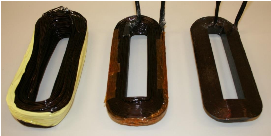
Figure 9-5: Coils at three stages of construction (left to right); following bobbin winding, the 'blank' following first stage compression and completed coil following final compression.
