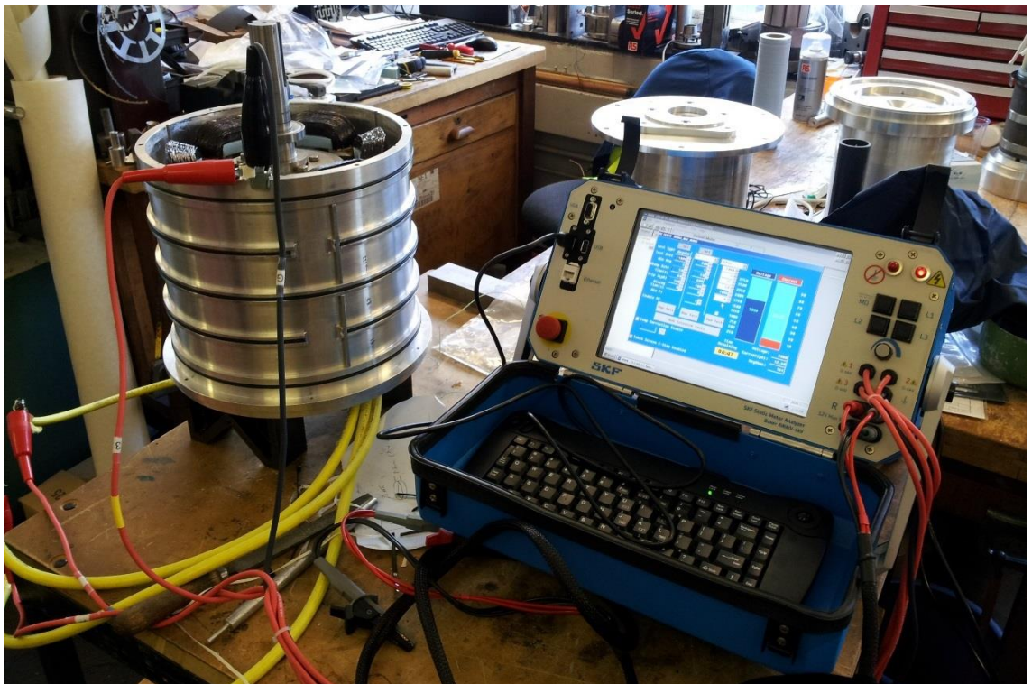
Figure 9-19: Stator laminations fitted into inner-water jacket and under test with Baker Instruments motor winding test system.
