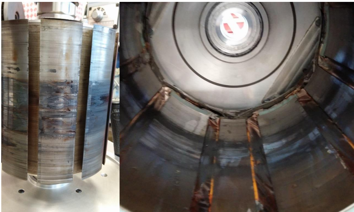
Figure 10-29: Witness marks on rotor and stator following Test 3.
