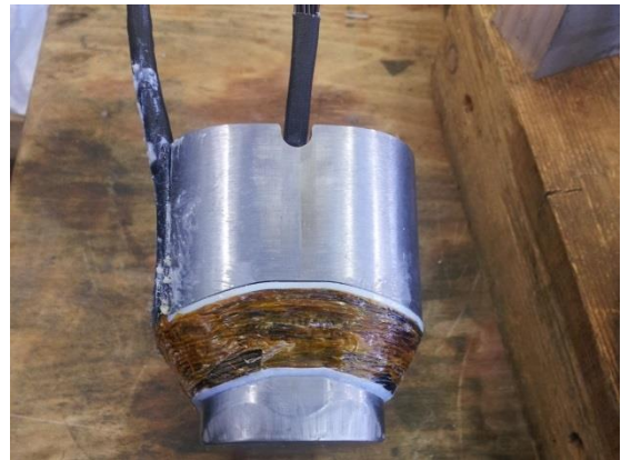
Figure 9-11: Bobbin and Punch removed from die, clearly showing compressed coil and both top and bottom inserts.
