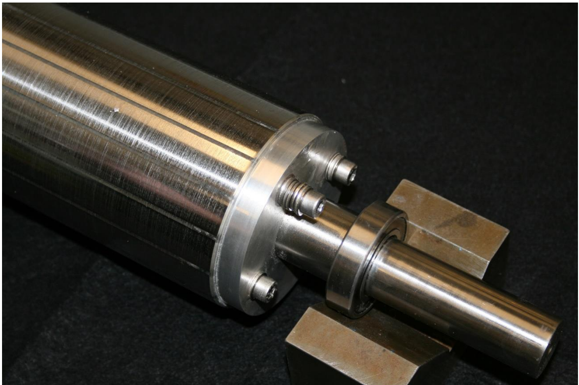
Figure 4-6: Completed rotor after machining to final outer diameter. This figure also shows how the rotor was balanced by fitting additional washers to the end-cap bolts.
