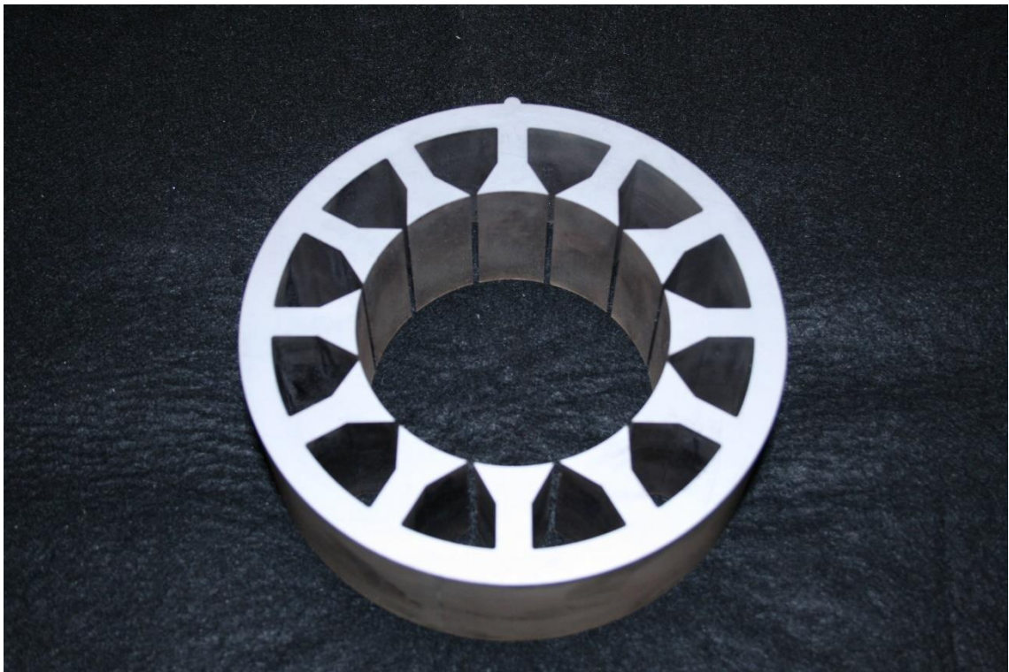
Figure 4-1: EDM cut, 50mm stator lamination sub-stack.
