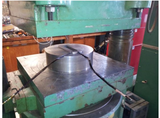
Figure 9-9: Die tooling positioned in 500 tonne press ready for compression. Wire terminations are shown laid flat in specially prepared channels.
