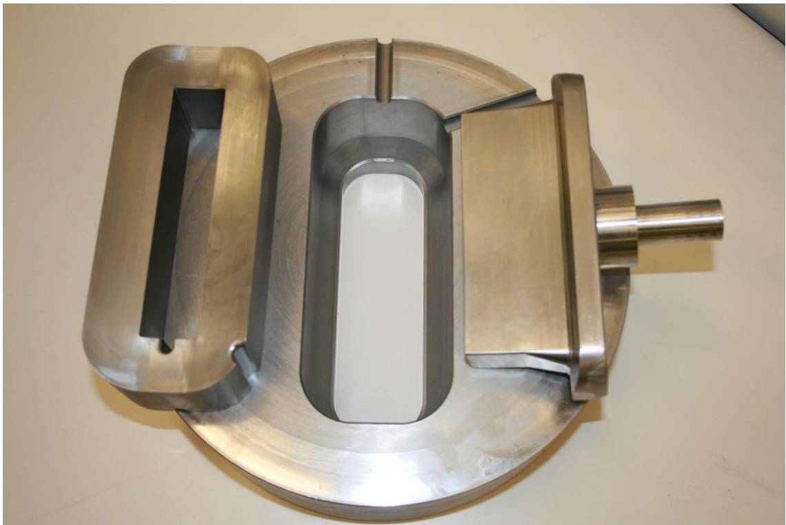
Figure 9-3: Showing final punch (left), die (bottom) and bobbin (right) set.
