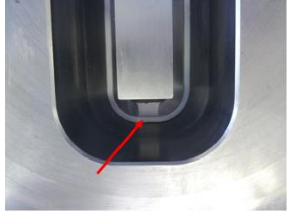
Figure 9-7: The rapid prototyped insert to prevented extrusion of the aluminium wire between bobbin and die.
