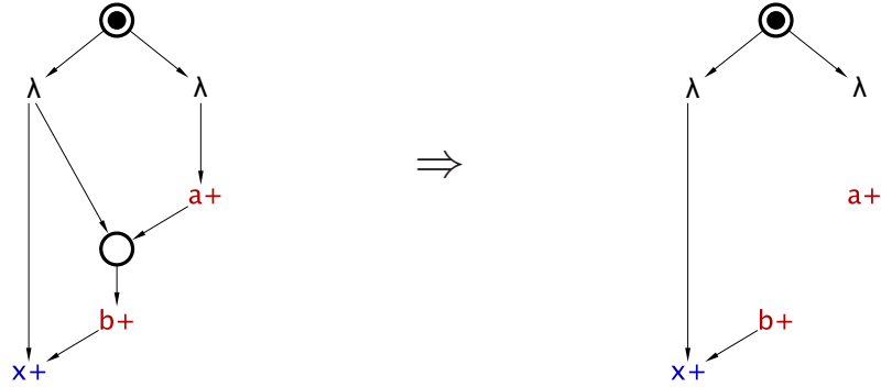
Figure 3.4: Example of an STG where removal of places in the postset of dummy transitions results in a wrong behaviour.
