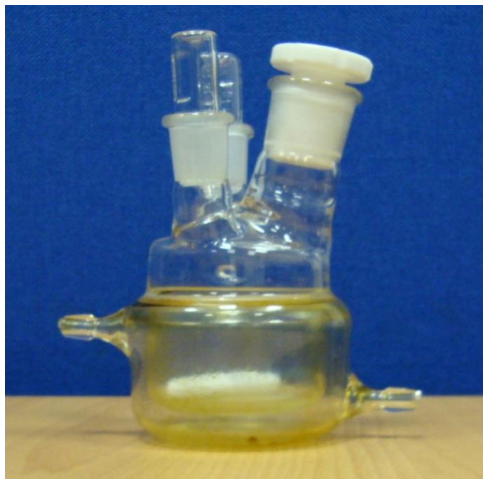
Figure 3.1: Jacketed 3-neck stirred tank batch reactor
