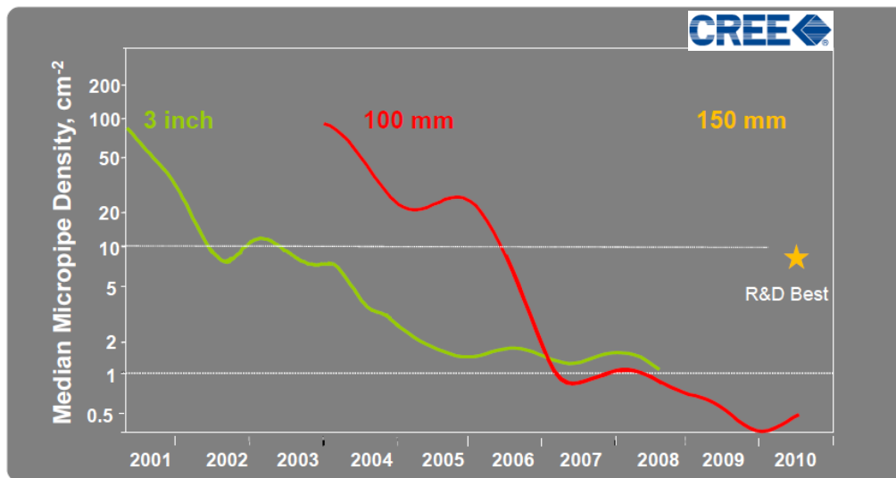
Figure 2.9. Micropipe reduction of 4H-SiC substrates by Cree [42].
