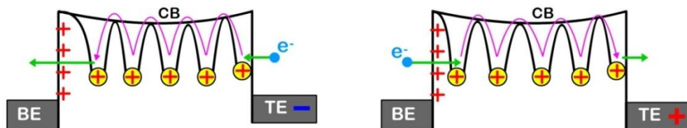
Figure 5.2: Illustrations of conduction mechanism under different voltage polarities.
