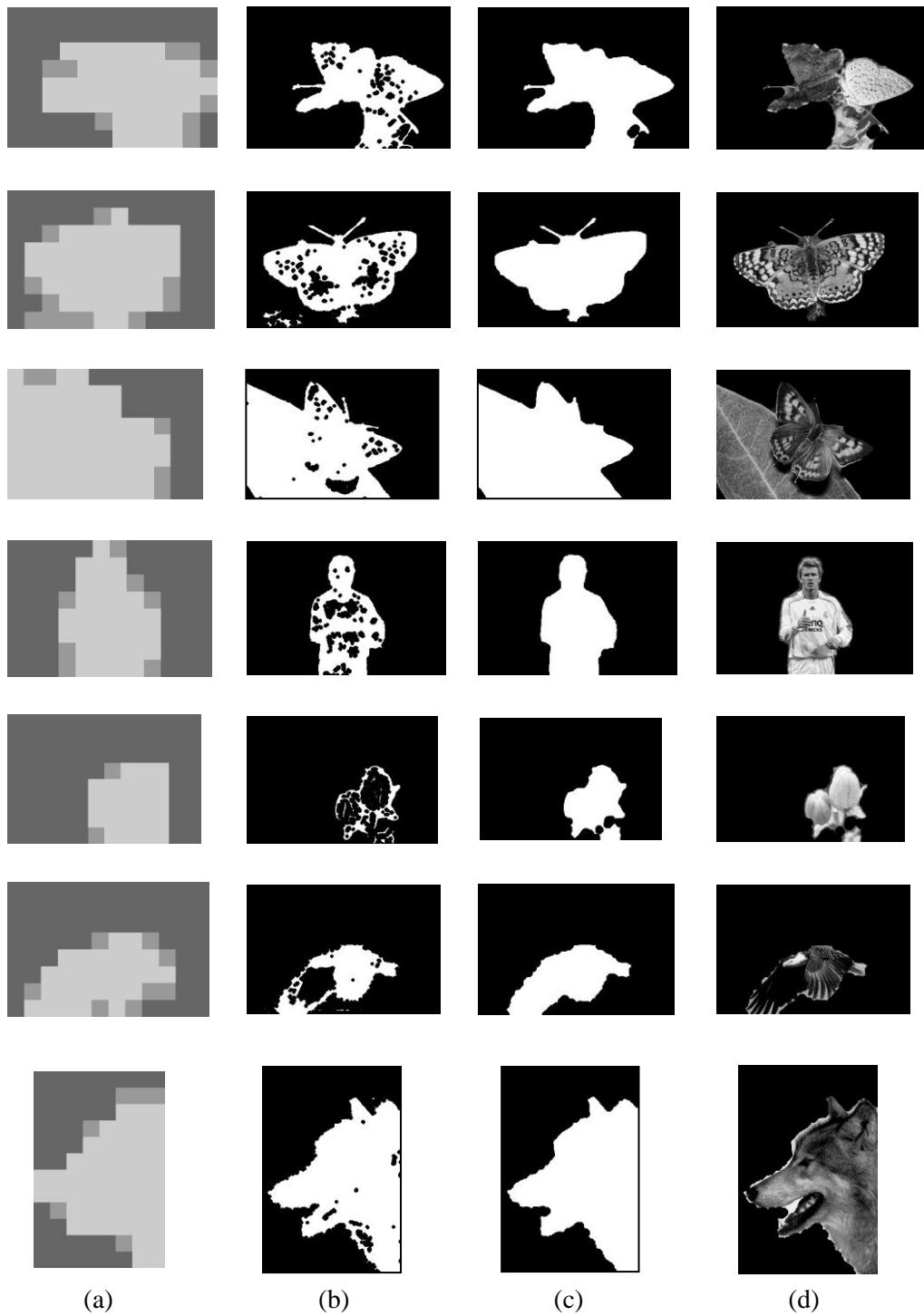
Figure 4.9: Illustration of final clustering results. (a) Block-based interest regions using the ensemble clustering algorithm. Region saliency map (b). Estimated mask by the proposed approach (c). Final segmentation results (d).
