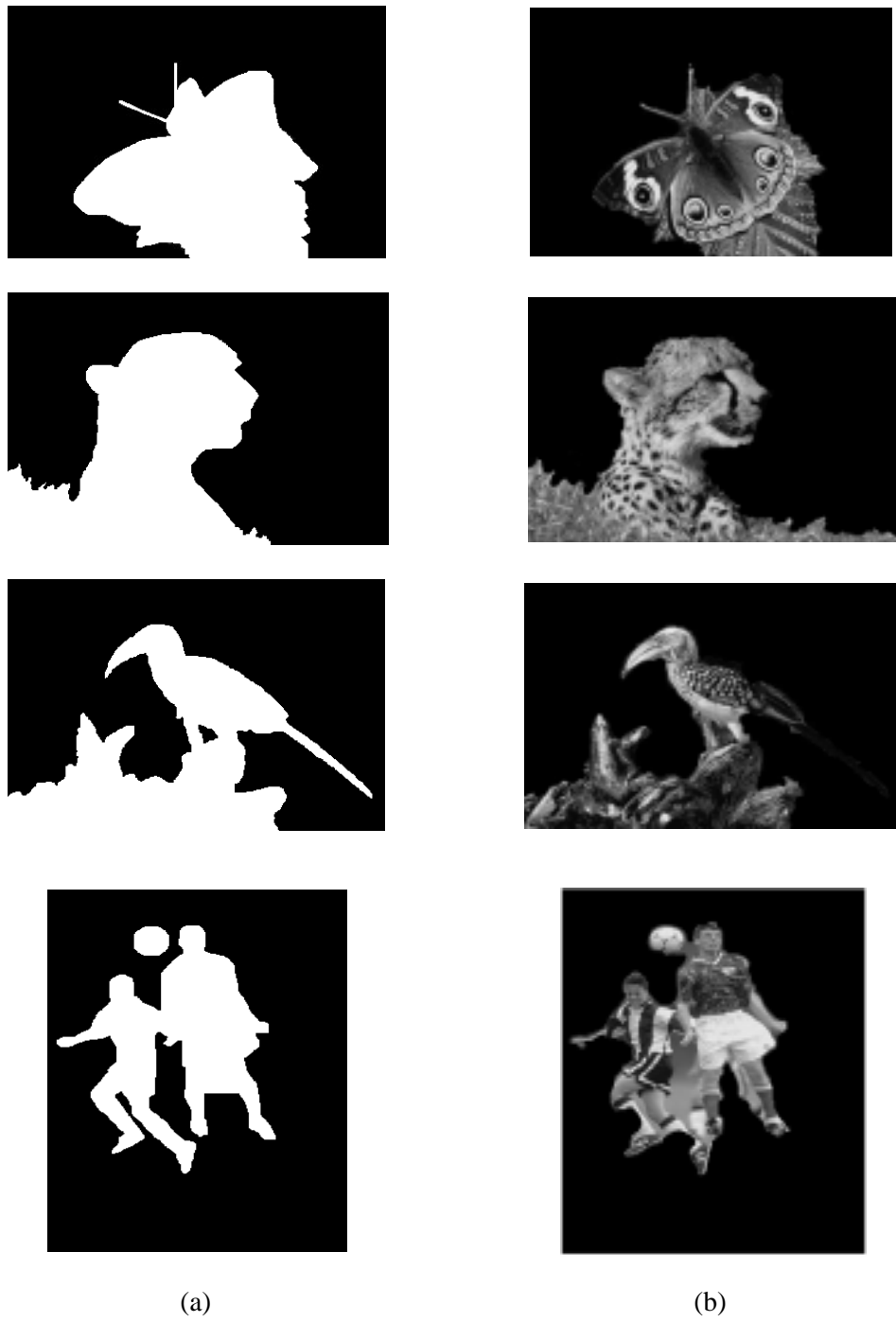
Figure 2.20: Illustration of segmentation results obtained from the approach [42]. (a) Manually segmented images (i.e., ground truth masks). (b) Segmentation results using the supervised learning approach.
