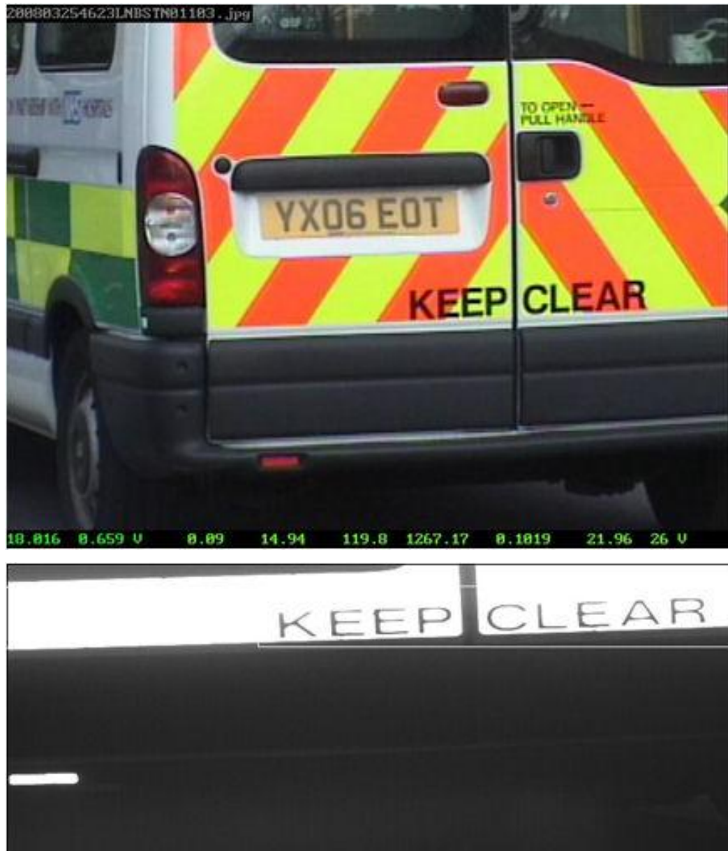
Figure 50: Example ANPR error reading 'Keep Clear' sign
