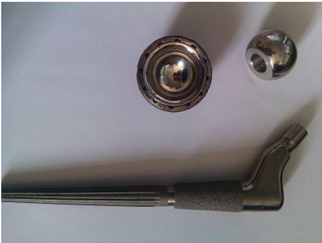
Figure 1.5: The Pinnacle® acetabular cup system, with a metal lining, a 36mm CoCrMo femoral head and a titanium stem. Note the internal taper of the head, which connects to the trunnion at the proximal end of the stem.
