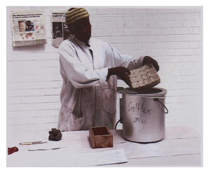
Plate 3-124: Melting the Gelflex  $\circ$
