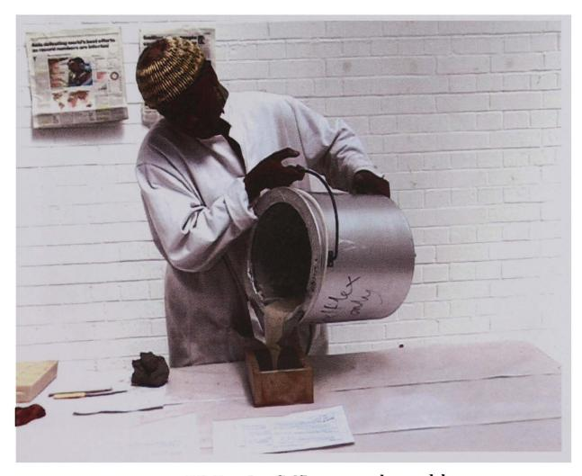
Plate 3-125: Pouring Gelflex over a clay model.
